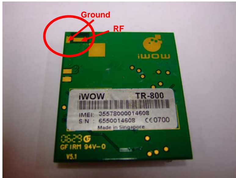
Figure 10: RF and Ground pad on TR-800
