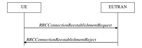
Figure 5.3.7.1-2: RRC connection re-establishment, failure
