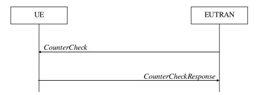
Figure 5.3.6.1-1: Counter check procedure
