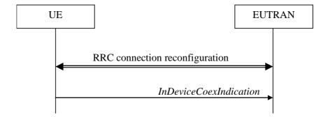
Figure 5.6.9.1-1: In-device coexistence indication
