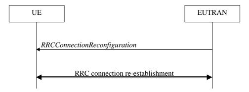
Figure 5.3.5.1-2: RRC connection reconfiguration, failure
