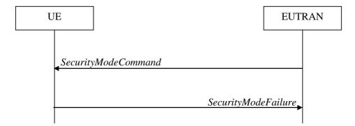
Figure 5.3.4.1-2: Security mode command, failure
