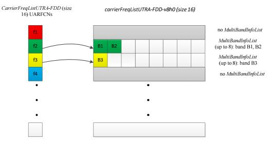
Figure D.1.3-1: Mapping of UARFCNs to MultiBandInfoList
