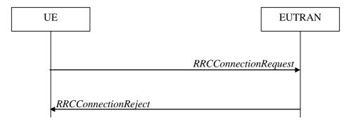
Figure 5.3.3.1-2: RRC connection establishment, network reject
