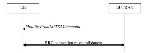
Figure 5.4.3.1-2: Mobility from E-UTRA, failure
