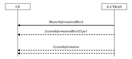
Figure 5.2.2.1-1: System information acquisition, normal
