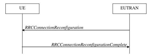
Figure 5.3.5.1-1: RRC connection reconfiguration, successful
