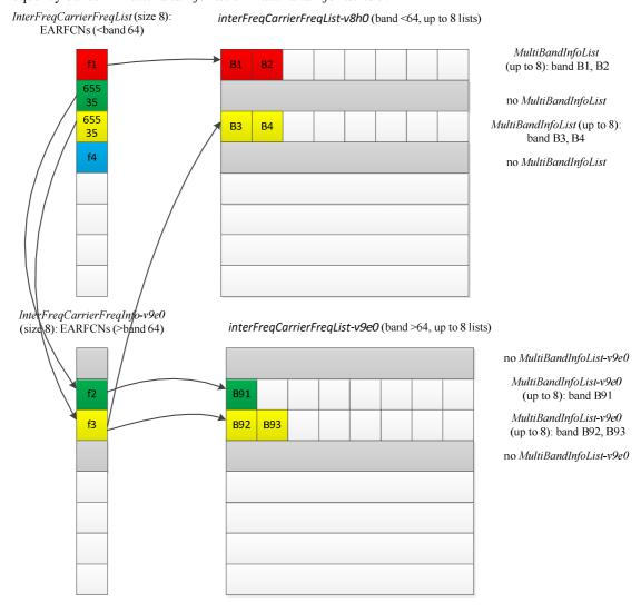
Figure D.1.2-1: Mapping of EARFCNs to MultiBandInfoList/MultiBandInfoList-v9e0
