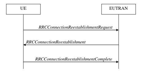
Figure 5.3.7.1-1: RRC connection re-establishment, successful
