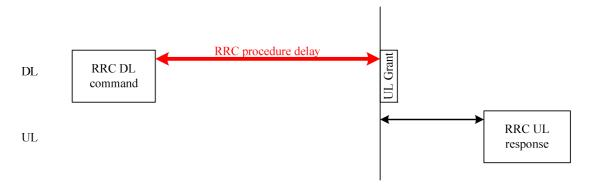
Figure 11.2-1: Illustration of RRC procedure delay
