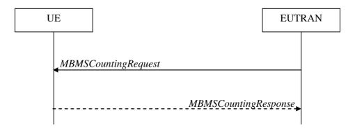
Figure 5.8.4.1-1: MBMS Counting procedure
