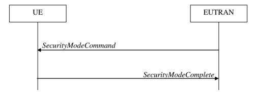
Figure 5.3.4.1-1: Security mode command, successful
