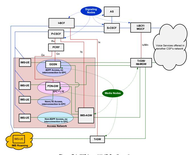
Figure E.1: IMS-based VoIP Configuration
