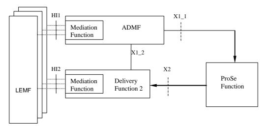
Figure 17.1-1: ProSe Direct Discovery Intercept configuration
