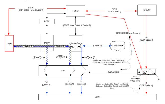
Figure G.3-1: Transcoded Media with e2ae encryption
