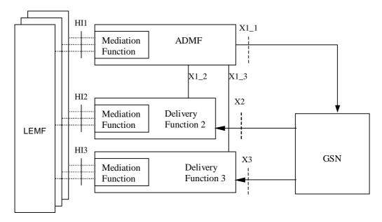
Figure 1b: Packet Switched Intercept configuration
