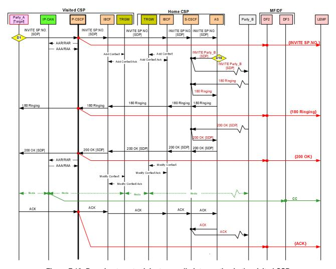
Figure F.10: Roaming target originates a call - interception in the visited CSP
