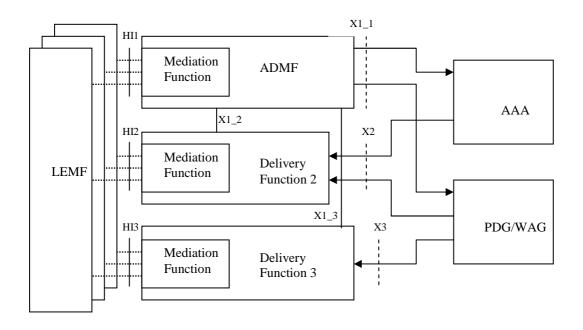
Figure 1e: WLAN Interworking Intercept configuration
