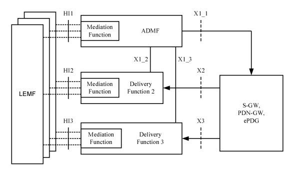
Figure 12.1.3: S-GW, PDN-GW, ePDG Intercept configuration
