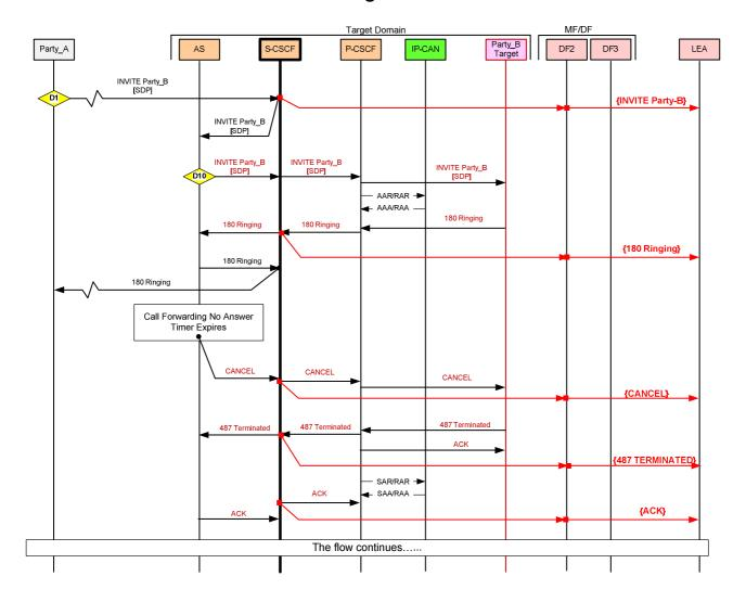
Figure F.5: Incoming call to target is forwarded due to call forwarding no answer within the CSP (flow 1 of 2)
