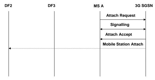
Figure B.1: Interception of mobile originated Mobile Station Attachment
