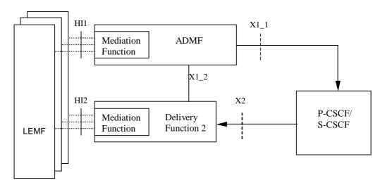
Figure 1d: IMS-CSCF Intercept configuration
