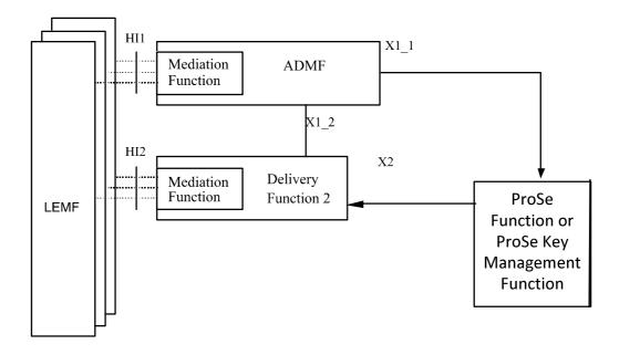
Figure 17.2-1: ProSe One To Many Communications Intercept configuration
