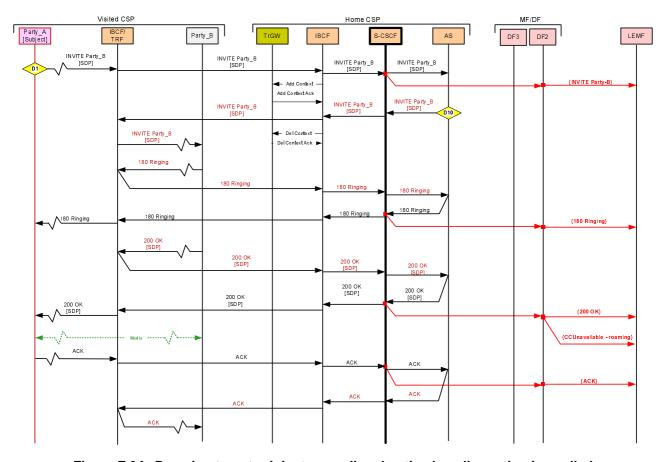
Figure F.8A: Roaming target originates a call and optimal media routing is applied
