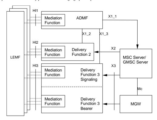
Figure 1a: Circuit switched intercept configuration
