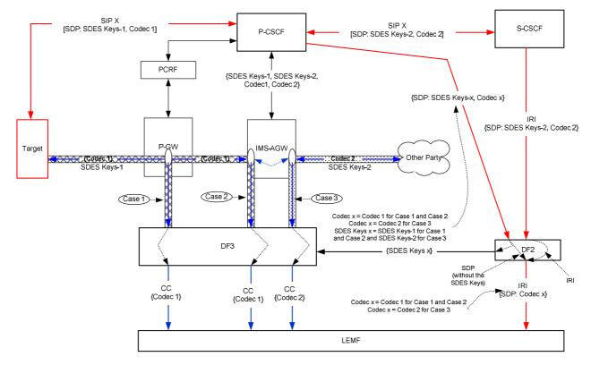
Figure G.4-1: Transcoded Media with e2e encryption
