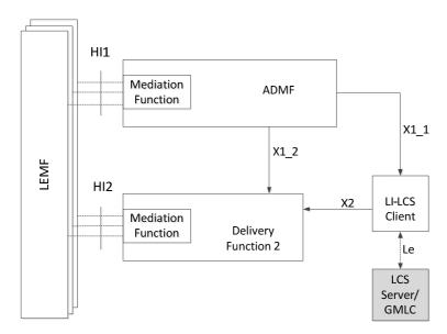
Figure 19.2.1: LALS Model for Target Positioning
