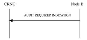
Figure 9: Audit Required procedure, Successful Operation
