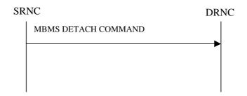
Figure 32: MBMS Detach procedure, Successful Operation
