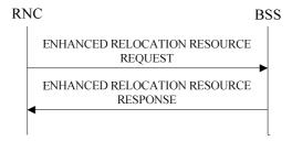
Figure 4B: Enhanced Relocation Resource Allocation Procedure, Successful Operation
