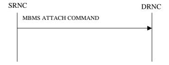
Figure 31: MBMS Attach procedure, Successful Operation
