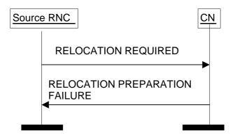
Figure 6: Relocation Preparation procedure. Unsuccessful operation.
