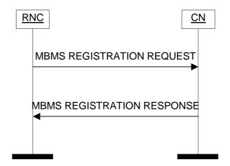
Figure 52: MBMS Registration procedure. Successful operation.
