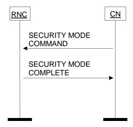
Figure 19: Security Mode Control procedure. Successful operation.
