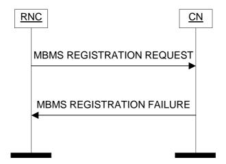
Figure 53: MBMS Registration procedure. Unsuccessful operation.
