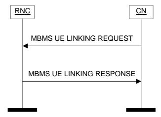
Figure 51: MBMS UE Linking procedure. Successful operation.
