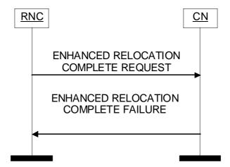
Figure 69: Enhanced Relocation Complete procedure. Unsuccessful operation.
