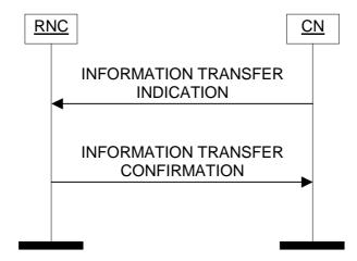
Figure 39: Information Transfer procedure. Successful operation.
