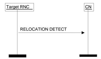
Figure 9: Relocation Detect procedure: Successful operation.
