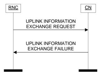
Figure 45: Uplink Information Exchange procedure. Unsuccessful operation.
