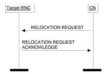
Figure 7: Relocation Resource Allocation procedure. Successful operation.
