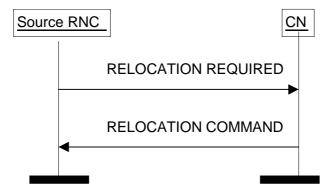
Figure 5: Relocation Preparation procedure. Successful operation.
