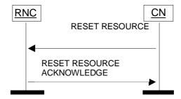
Figure 35: CN initiated Reset Resource procedure. Successful operation.
