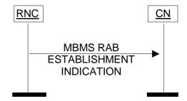
Figure 55: MBMS RAB Establishment Indication procedure. Successful operation.
