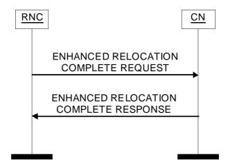
Figure 58: Enhanced Relocation Complete procedure. Successful operation.
