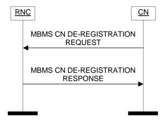
Figure 54: MBMS CN De-Registration procedure. Successful operation.
