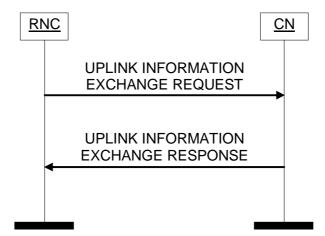
Figure 44: Uplink Information Exchange procedure. Successful operation.
