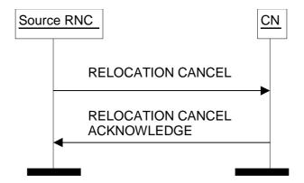
Figure 11: Relocation Cancel procedure. Successful operation.
