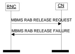
Figure 57: MBMS RAB RELEASE procedure. Unsuccessful operation.
