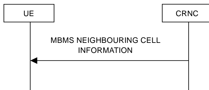
Figure 8.3.5: MBMS Neighbouring Cell Information signalling flow
