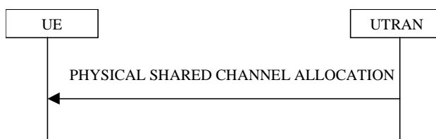
Figure 8.2.7-1: Physical Shared Channel Allocation
