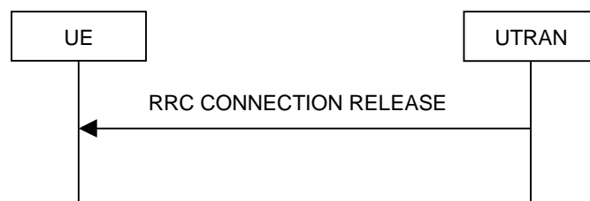
Figure 8.1.4-2: RRC Connection Release procedure on the CCCH
