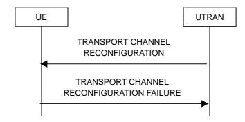
Figure 8.2.2-8: Transport channel reconfiguration, failure case
