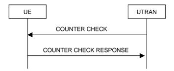
Figure 8.1.15-1: Counter check procedure
