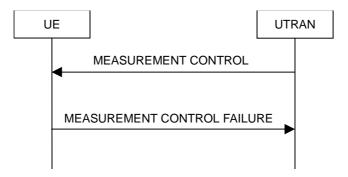
Figure 8.4.1-2: Measurement Control, failure case
