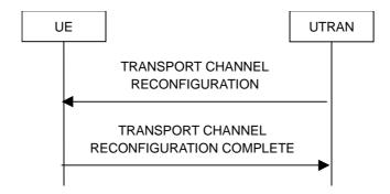
Figure 8.2.2-7: Transport channel reconfiguration, normal flow
