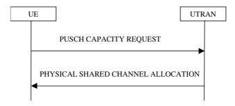
Figure 8.2.8-1: PUSCH Capacity request procedure
