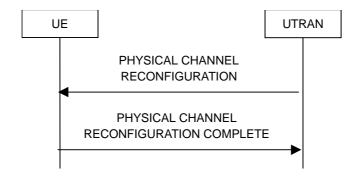
Figure 8.2.2-9: Physical channel reconfiguration, normal flow
