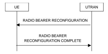
Figure 8.2.2-3: Radio bearer reconfiguration, normal flow
