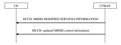
Figure 8.7.3-2: MBMS notification on DCCH
