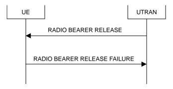
Figure 8.2.2-6: Radio Bearer Release, failure case
