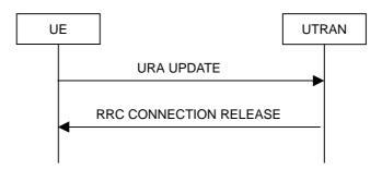
Figure 8.3.1-10: URA update procedure, failure case
