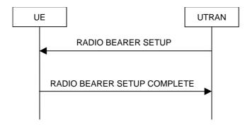
Figure 8.2.2-1: Radio Bearer Establishment, normal case
