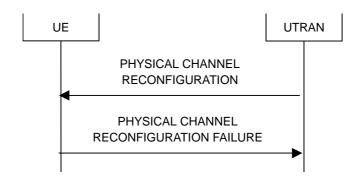
Figure 8.2.2-10: Physical channel reconfiguration, failure case
