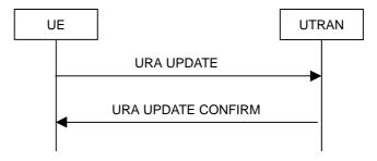
Figure 8.3.1-8: URA update procedure, basic flow
