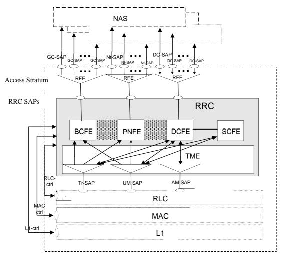
Figure 4.2-1: UE side model of RRC
