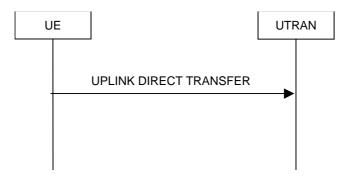
Figure 8.1.10-1: Uplink Direct transfer, normal flow
