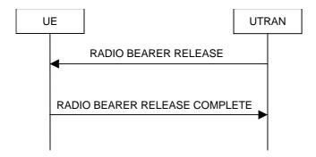
Figure 8.2.2-5: Radio Bearer Release, normal case
