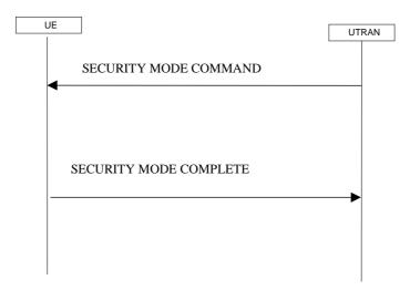
Figure 8.1.12-1: Security mode control procedure
