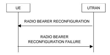
Figure 8.2.2-4: Radio bearer reconfiguration, failure case
