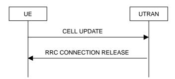
Figure 8.3.1-7: Cell update procedure, failure case
