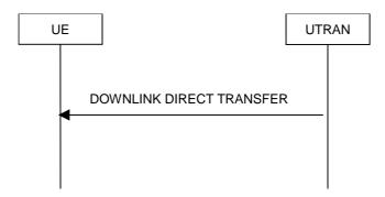
Figure 8.1.9-1: Downlink Direct transfer, normal flow
