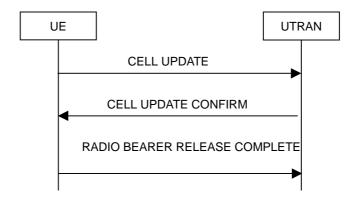
Figure 8.3.1-5: Cell update procedure with radio bearer release
