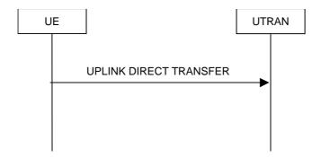
Figure 8.1.10-1: Uplink Direct transfer, normal flow
