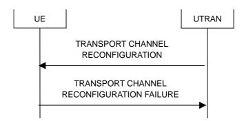
Figure 8.2.2-8: Transport channel reconfiguration, failure case
