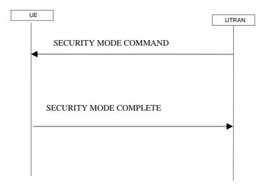
Figure 8.1.12-1: Security mode control procedure
