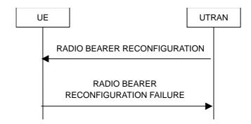
Figure 8.2.2-4: Radio bearer reconfiguration, failure case
