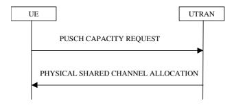
Figure 8.2.8-1: PUSCH Capacity request procedure
