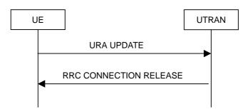
Figure 8.3.1-10: URA update procedure, failure case
