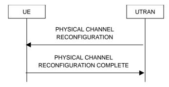
Figure 8.2.2-9: Physical channel reconfiguration, normal flow
