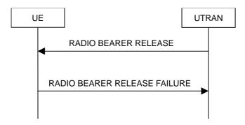
Figure 8.2.2-6: Radio Bearer Release, failure case
