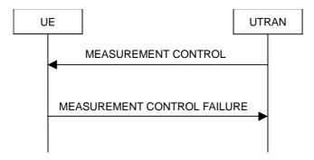
Figure 8.4.1-2: Measurement Control, failure case
