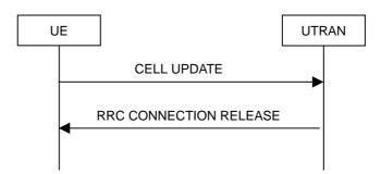
Figure 8.3.1-7: Cell update procedure, failure case
