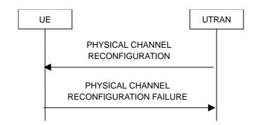
Figure 8.2.2-10: Physical channel reconfiguration, failure case
