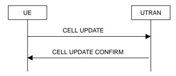
Figure 8.3.1-1: Cell update procedure, basic flow
