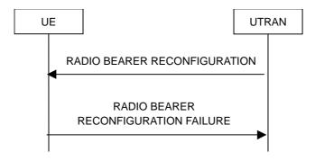
Figure 8.2.2-4: Radio bearer reconfiguration, failure case
