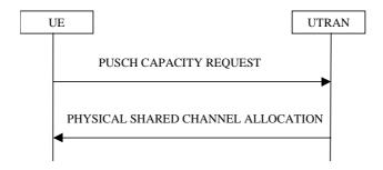
Figure 8.2.8-1: PUSCH Capacity request procedure
