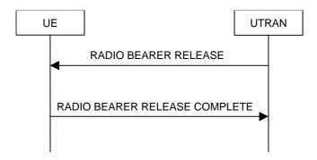
Figure 8.2.2-5: Radio Bearer Release, normal case
