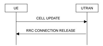
Figure 8.3.1-7: Cell update procedure, failure case
