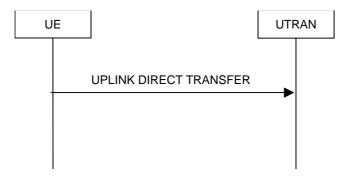
Figure 8.1.10-1: Uplink Direct transfer, normal flow
