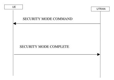
Figure 8.1.12-1: Security mode control procedure
