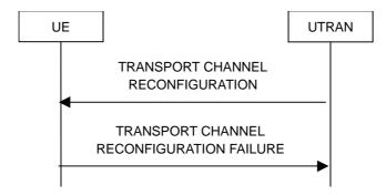
Figure 8.2.2-8: Transport channel reconfiguration, failure case
