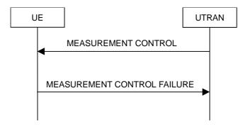
Figure 8.4.1-2: Measurement Control, failure case
