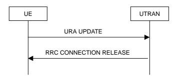
Figure 8.3.1-10: URA update procedure, failure case
