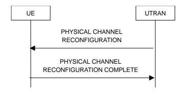
Figure 8.2.2-9: Physical channel reconfiguration, normal flow
