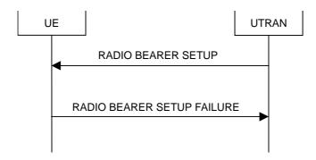
Figure 8.2.2-2: Radio Bearer Establishment, failure case
