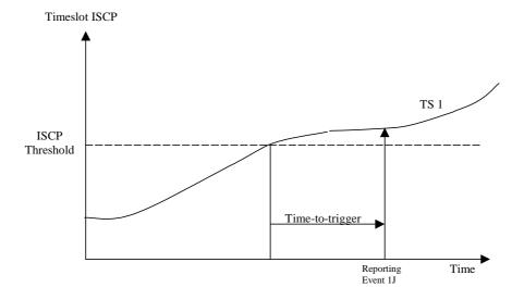
Figure 14.1.5.2-2: Time-to-trigger limits the amount of measurement reports
