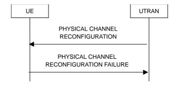
Figure 8.2.2-10: Physical channel reconfiguration, failure case
