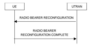
Figure 8.2.2-3: Radio bearer reconfiguration, normal flow
