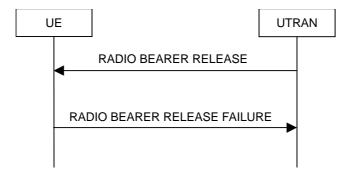
Figure 8.2.2-6: Radio Bearer Release, failure case
