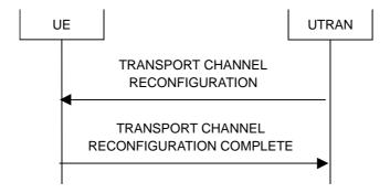
Figure 8.2.2-7: Transport channel reconfiguration, normal flow
