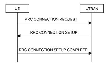
Figure 8.1.3-1: RRC Connection Establishment, network accepts RRC connection
