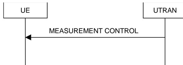
Figure 8.4.1-1: Measurement Control, normal case
