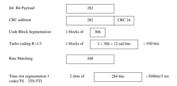
Figure A.12A: Coding for E-DCH FRC1 (1.28 Mcps TDD Option)
