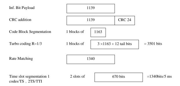
Figure A.13: Coding for E-DCH FRC2 (1.28 Mcps TDD Option)
