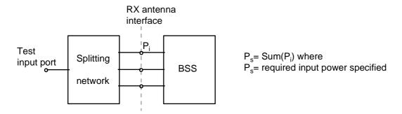
Figure 5.1: Receiver test set up
