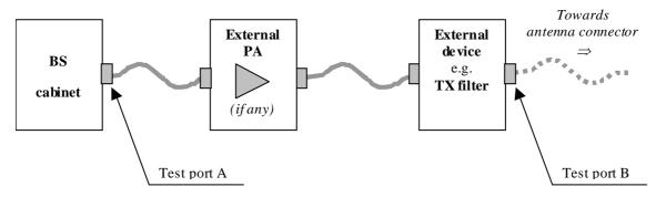
Figure 6.1: Transmitter test ports
