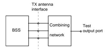
Figure 5.2: Transmitter test setup
