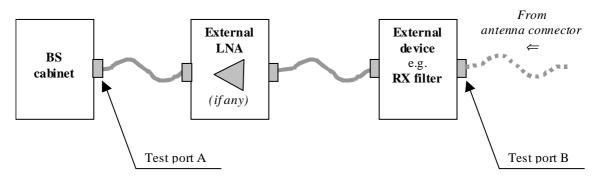
Figure 7.1: Receiver test ports
