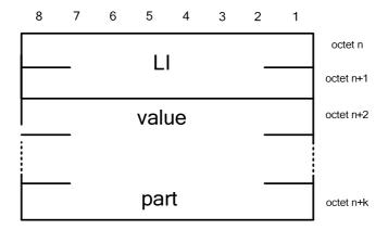
Figure I.2.2.4-9: Type 6 IE of format LV-E (k = 1, 2, ...)
