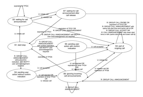
Figure 10.2.2.2-1: Basic call control state machine
