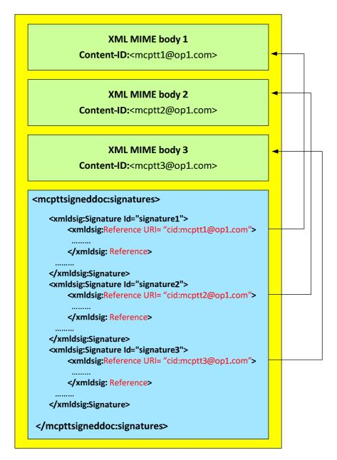
Figure 6.6.3.1-1: Integrity Protection of XML MIME bodies in SIP requests and SIP responses
