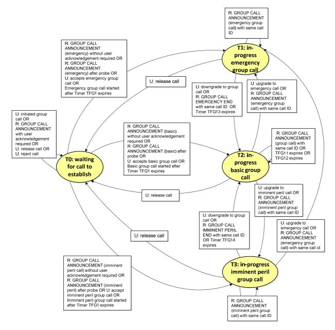
Figure 10.2.3.2-1: Call type control state machine
