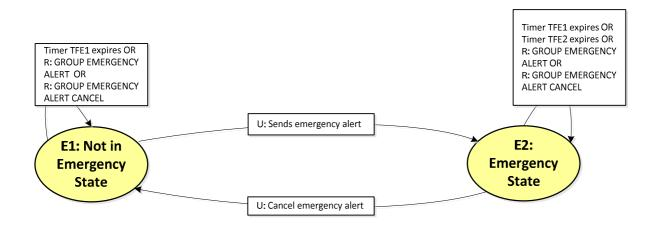
Figure 12.2.2.2-1: Emergency alert state machine
