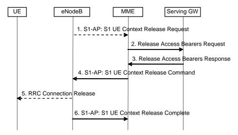
Figure 5.3.5-1: S1 Release Procedure
