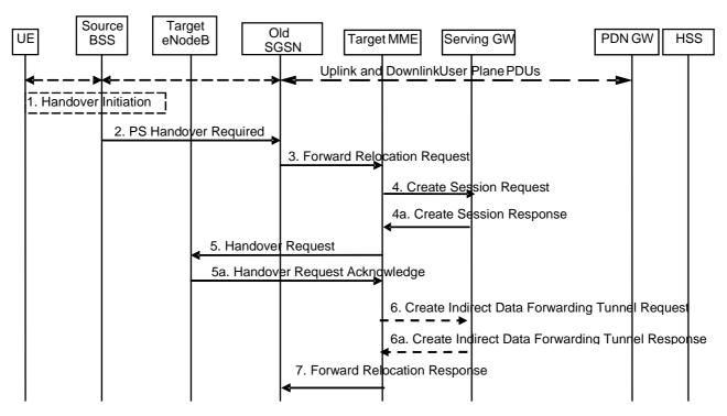
Figure D.3.8.2-1: GERAN A/Gb mode to E-UTRAN inter RAT HO, preparation phase
