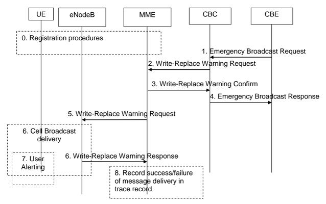
Figure 5.12.2.1-1: Warning message delivery procedure
