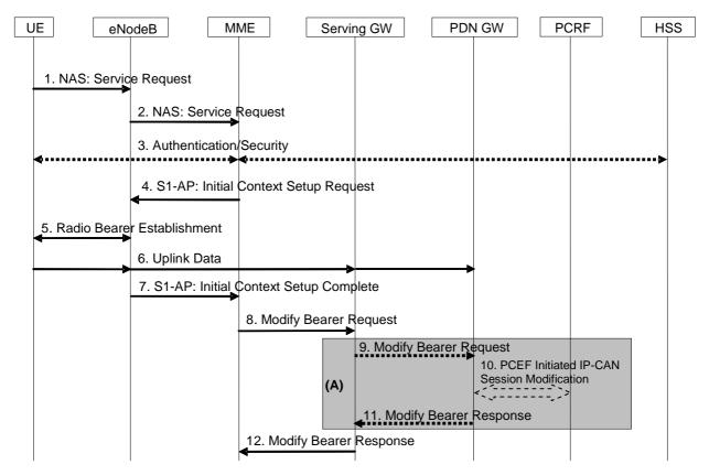
Figure 5.3.4.1-1: UE triggered Service Request procedure
