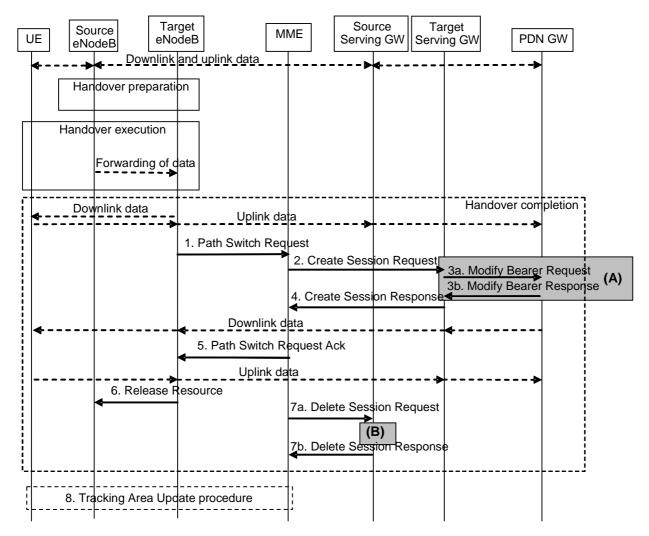
Figure 5.5.1.1.3-1: X2-based handover with Serving GW relocation
