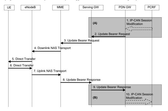
Figure 5.4.3-1: Bearer Modification Procedure without Bearer QoS Update
