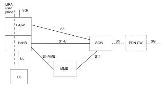
Figure 4.4.9-1: LIPA architecture for HeNB using a local PDN connection
