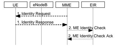
Figure 5.3.10.5-1: Identity Check Procedure
