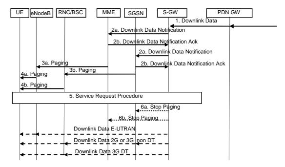
Figure 5.3.4.3-1: Network triggered Service Request procedure
