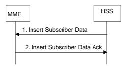
Figure 5.3.9.2-1: Insert Subscriber Data procedure
