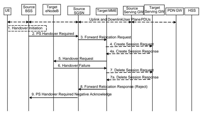
Figure 5.5.2.4.4-1: GERAN A/Gb mode to E-UTRAN inter RAT HO reject
