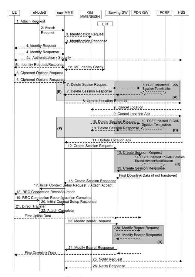
Figure 5.3.2.1-1: Attach procedure
