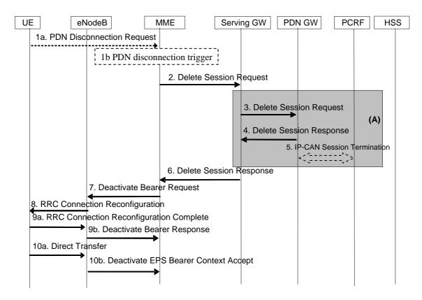
Figure 5.10.3-1: UE or MME requested PDN disconnection
