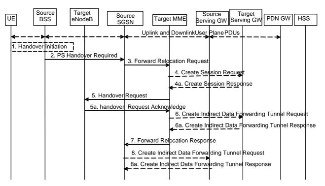
Figure 5.5.2.4.2-1: GERAN A/Gb mode to E-UTRAN inter RAT HO, preparation phase
