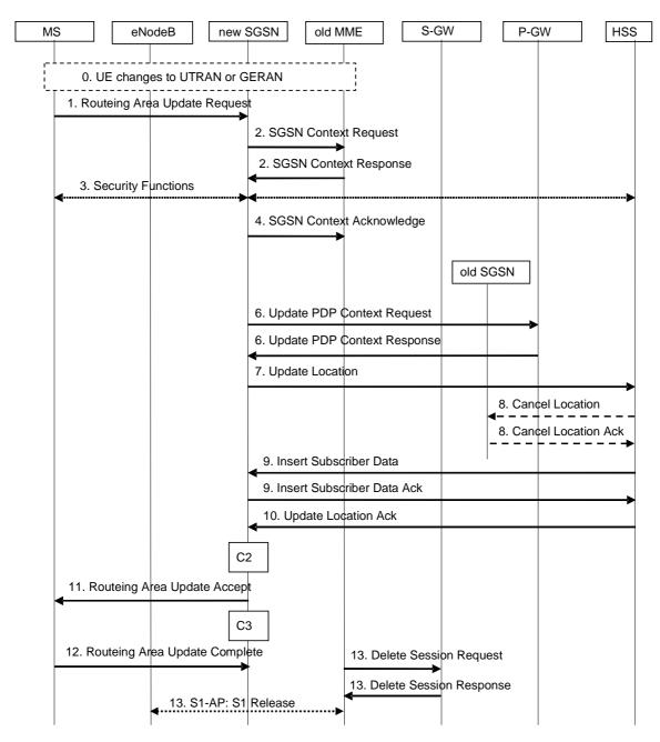
Figure D.3.5-1: Routing Area Update procedure
