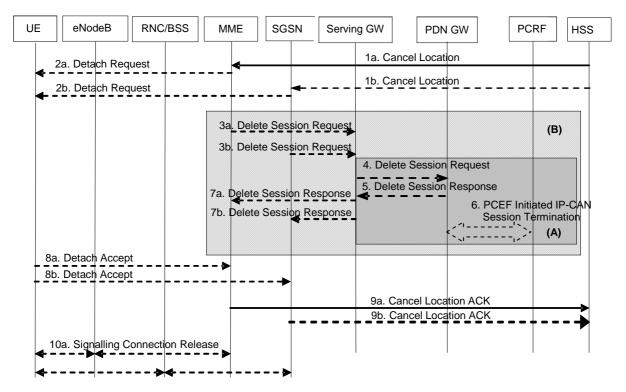
Figure 5.3.8.4-1: HSS-Initiated Detach Procedure
