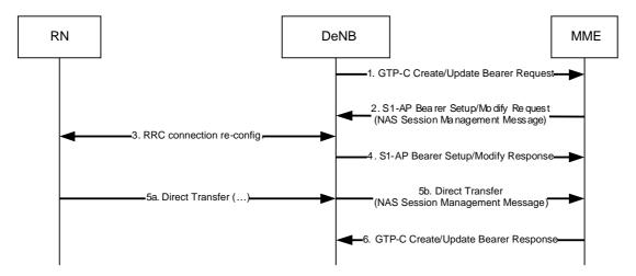
Figure 4.3.20.3-1: DeNB-initiated bearer activation/modification procedure
