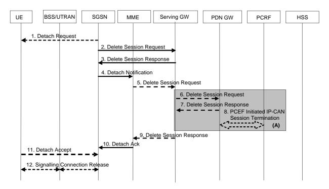
Figure 5.3.8.3A-1: SGSN-Initiated Detach Procedure with ISR activated
