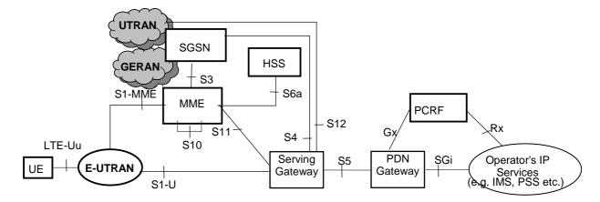
Figure 4.2.1-1: Non-roaming architecture for 3GPP accesses
