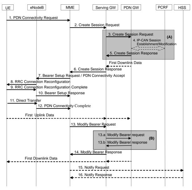
Figure 5.10.2-1: UE requested PDN connectivity
