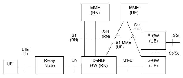
Figure 4.3.20.1-1: Relaying Architecture
