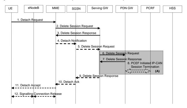
Figure 5.3.8.2-1: UE-Initiated Detach Procedure - UE camping on E-UTRAN
