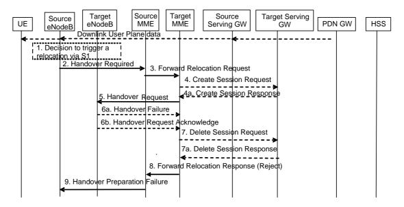
Figure 5.5.1.2.3-1: S1-based handover, Reject
