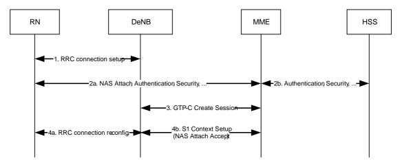
Figure 4.3.20.2-1: RN attach procedure
