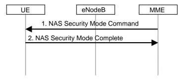
Figure 5.3.10.4.2-1: NAS Security Mode Command Procedure
