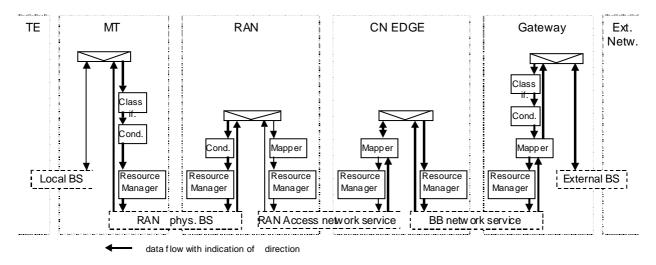
Figure 3: QoS management functions for the UMTS bearer service in the user plane
