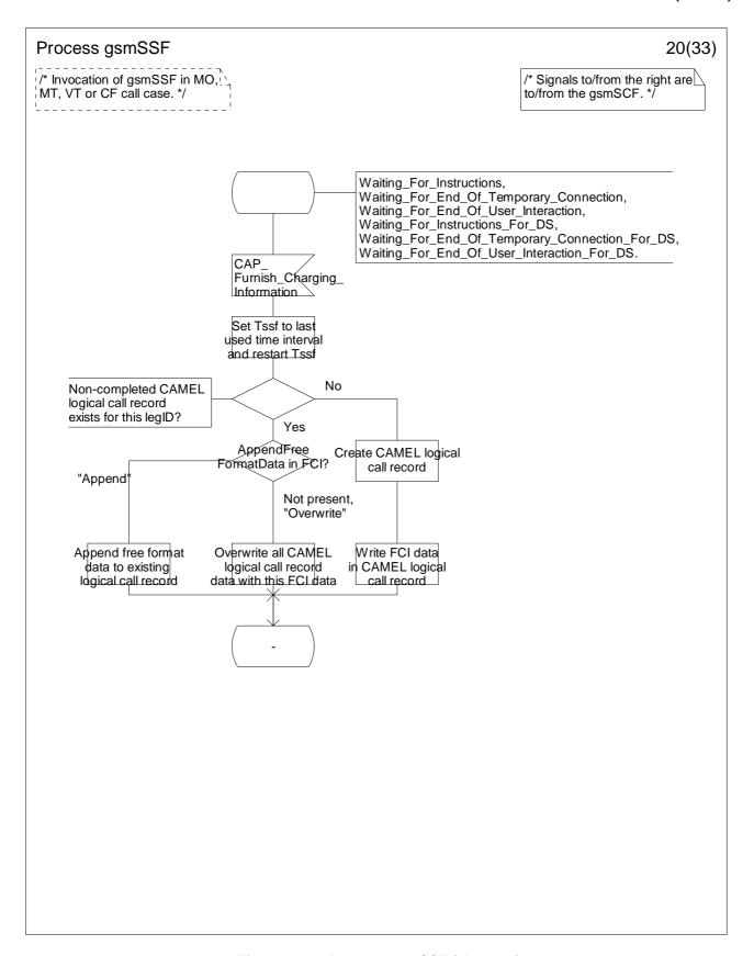
Figure 4.64t: Process gsmSSF (sheet 20)
