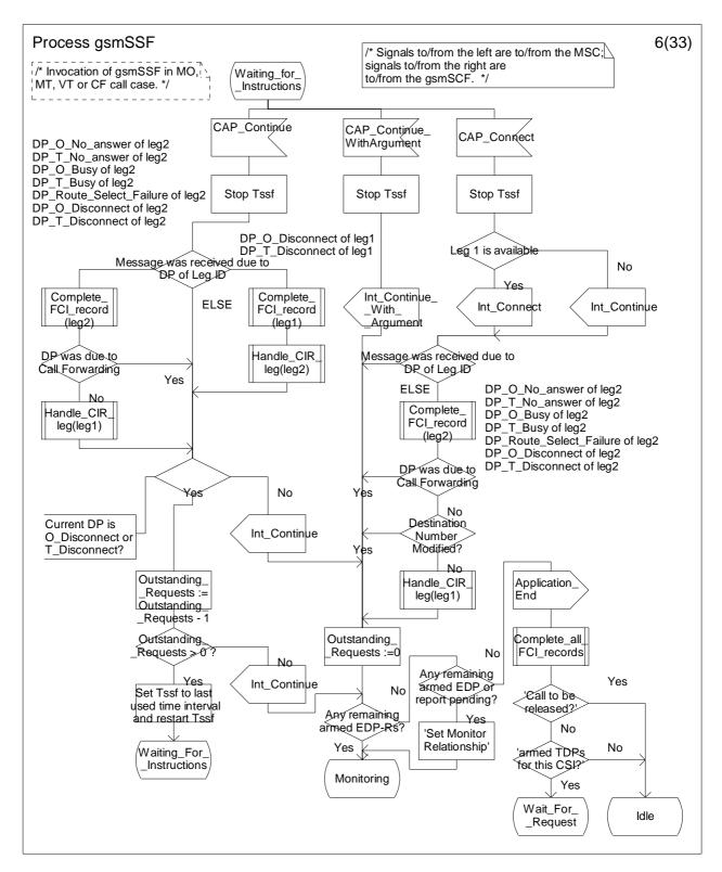
Figure 4.64f: Process gsmSSF (sheet 6)
