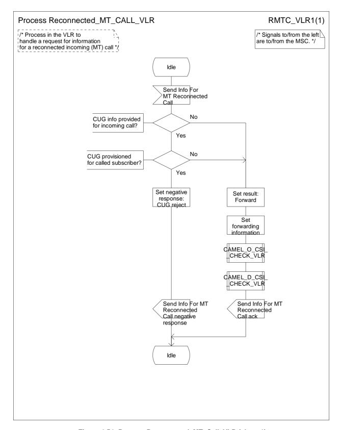
Figure 4.54: Process Reconnected\_MT\_Call\_VLR (sheet 1)
