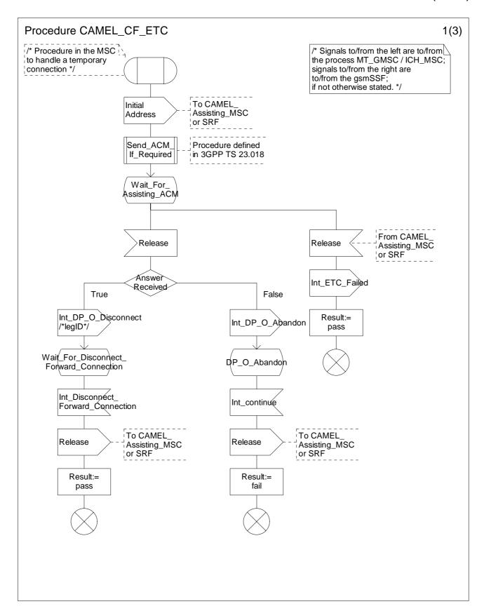
Figure 4.61a: Process CAMEL\_CF\_ETC (sheet 1)
