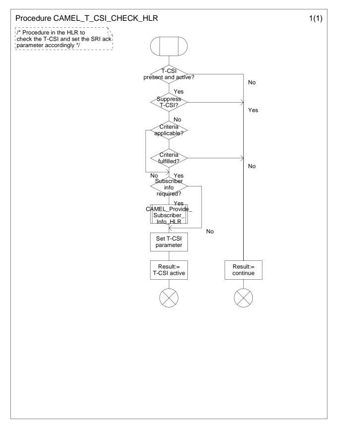
Figure 4.45: Procedure CAMEL\_T\_CSI\_CHECK\_HLR (sheet 1)
