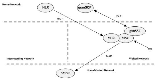
Figure 7.1: Functional architecture for support of CAMEL control of MSC switched MO SMS
