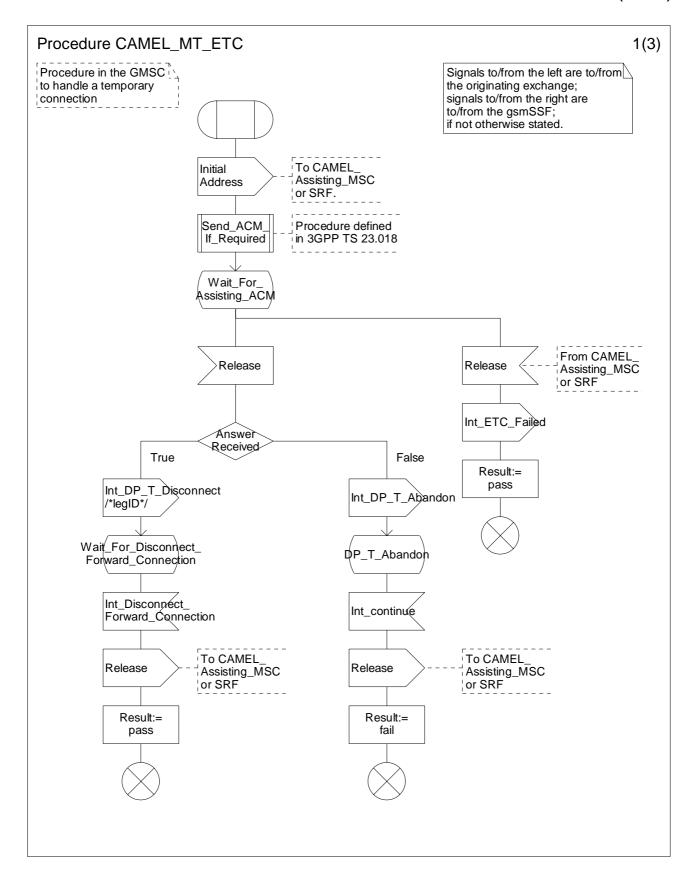
Figure 4.38a: Procedure CAMEL\_MT\_ETC (sheet 1)
