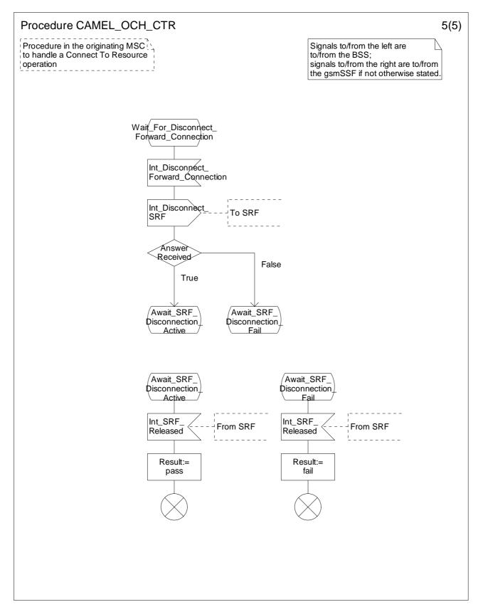
Figure 4.21e: Procedure CAMEL\_OCH\_CTR (sheet 5)
