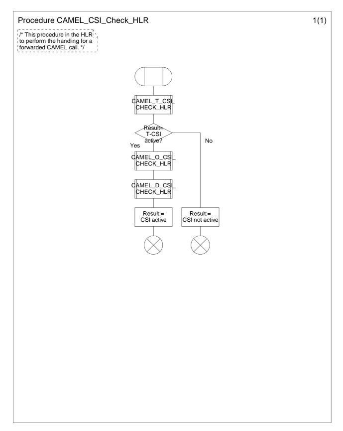
Figure 4.42: Procedure CAMEL\_CSI\_Check\_HLR (sheet 1)
