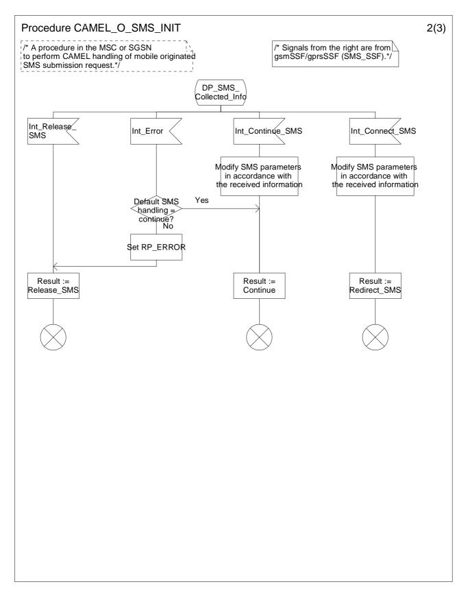
Figure 7.7b: Procedure CAMEL\_O\_SMS\_INIT (sheet 2)
