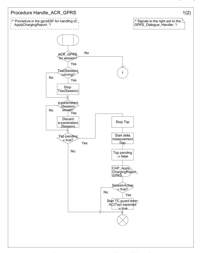
Figure 6.20a: Procedure Handle\_ACR\_GPRS (sheet 1)
