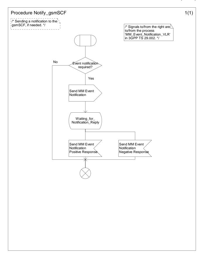
Figure 9.4: Procedure Notify\_gsmSCF (sheet 1)
