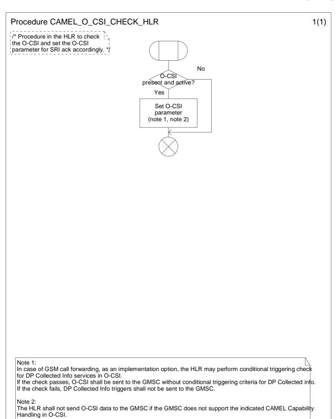
Figure 4.43: Procedure CAMEL\_O\_CSI\_CHECK\_HLR (sheet 1)
