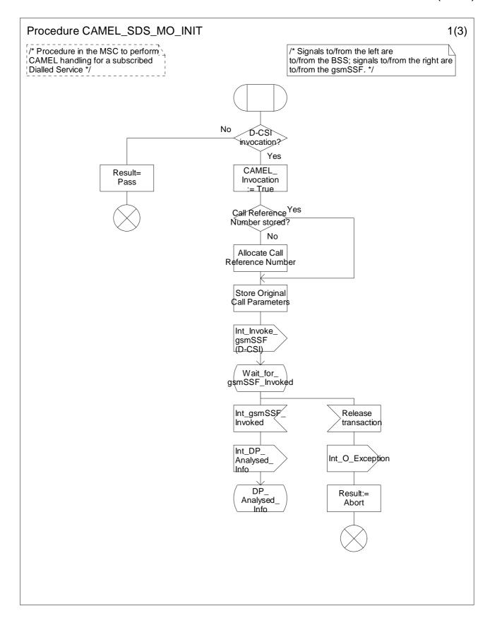
Figure 4.11a: Procedure CAMEL\_SDS\_MO\_Init (sheet 1)
