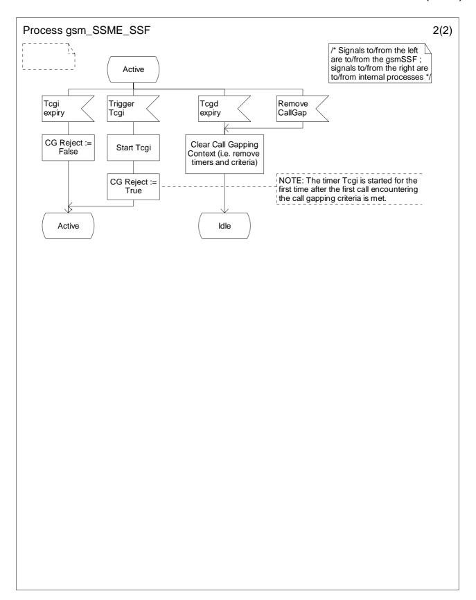
Figure 4.77b: Process gsm\_SSME\_SSF (sheet 2)
