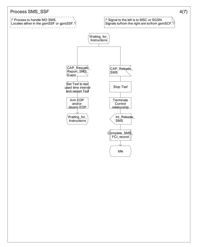
Figure 7.10d: Process SMS\_SSF (sheet 4)
