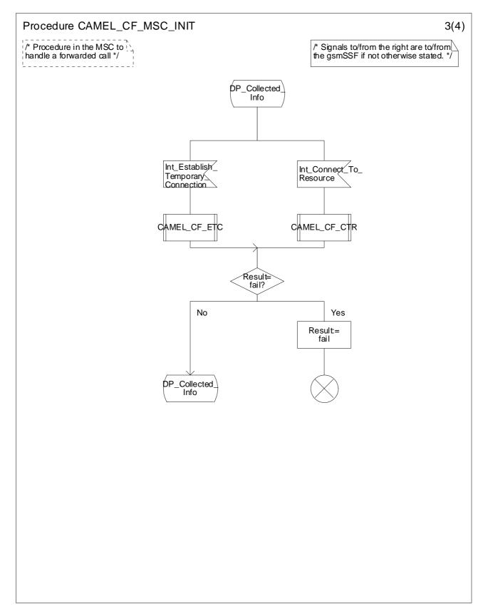
Figure 4.57c: Procedure CAMEL\_CF\_MSC\_INIT (sheet 3)
