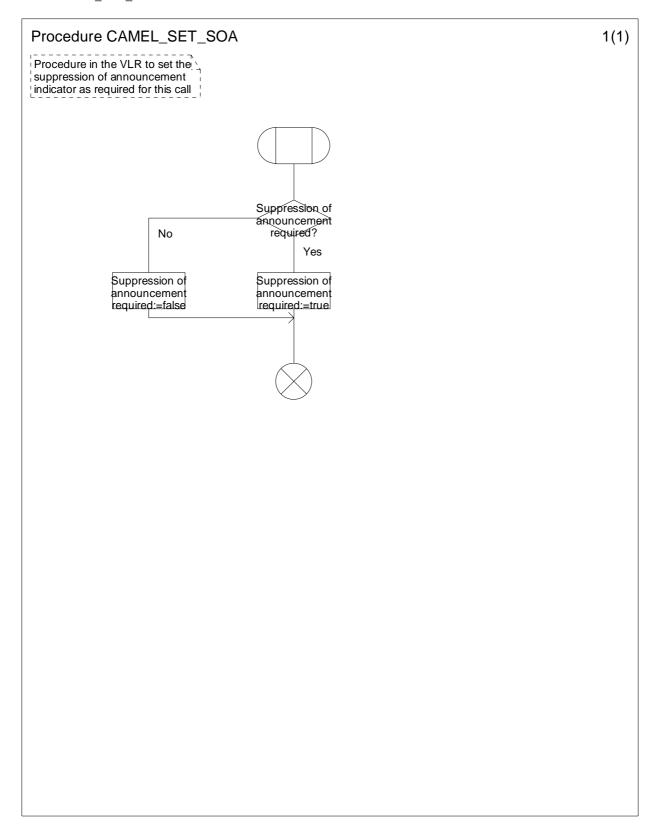
Figure 4.47: Procedure CAMEL\_SET\_SOA (sheet 1)
