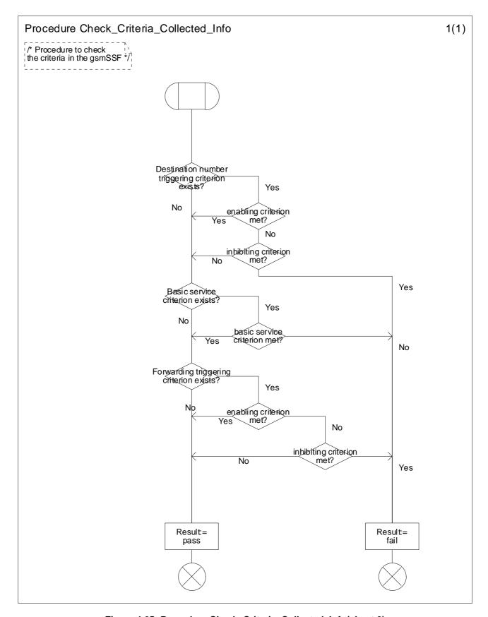
Figure 4.65: Procedure Check\_Criteria\_Collected\_Info(sheet 0)
