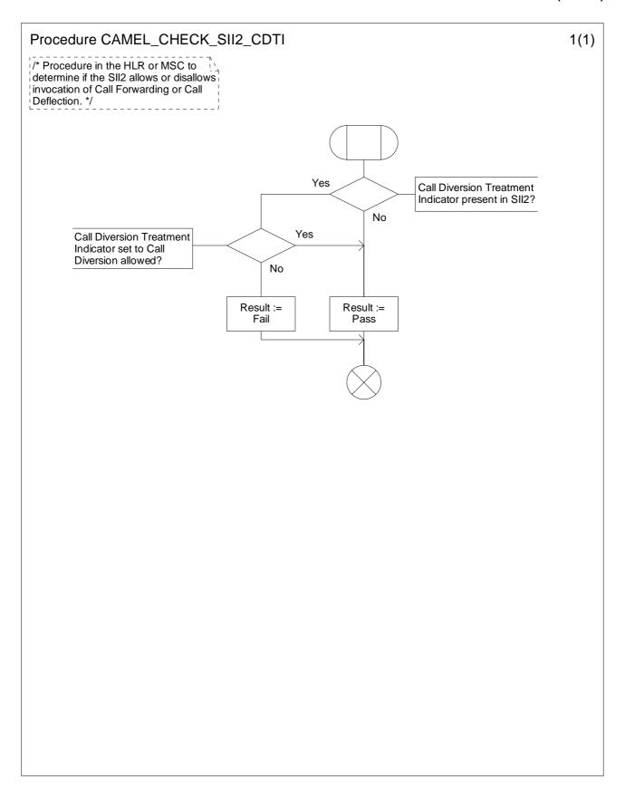
Figure 4.46: Procedure CAMEL\_CHECK\_SII2\_CDTI (sheet 1)
