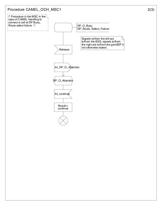
Figure 4.14b: Procedure CAMEL\_OCH\_MSC1 (sheet 2)
