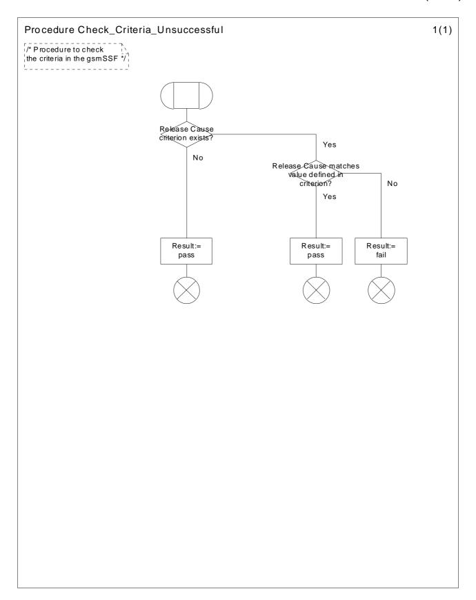
Figure 4.67: Procedure Check\_Criteria\_Unsuccessful(sheet 0)
