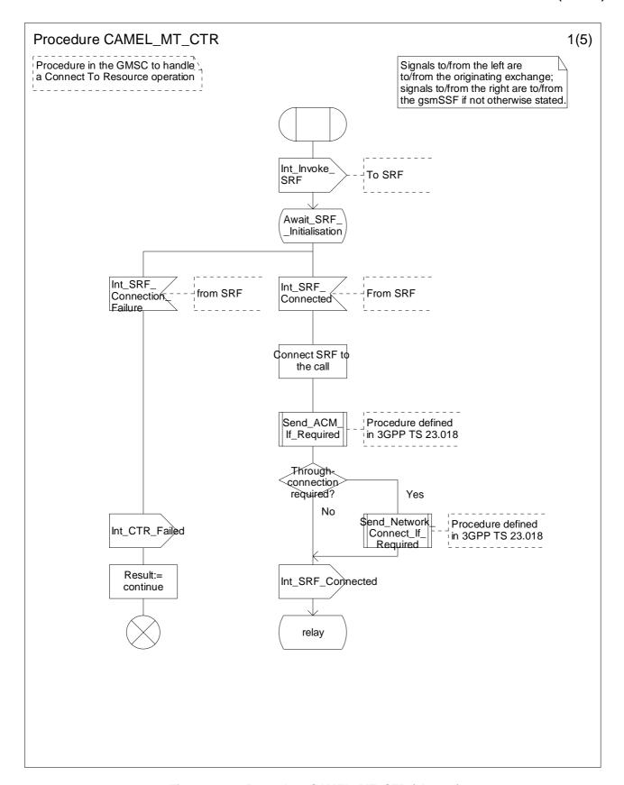
Figure 4.39a: Procedure CAMEL\_MT\_CTR (sheet 1)
