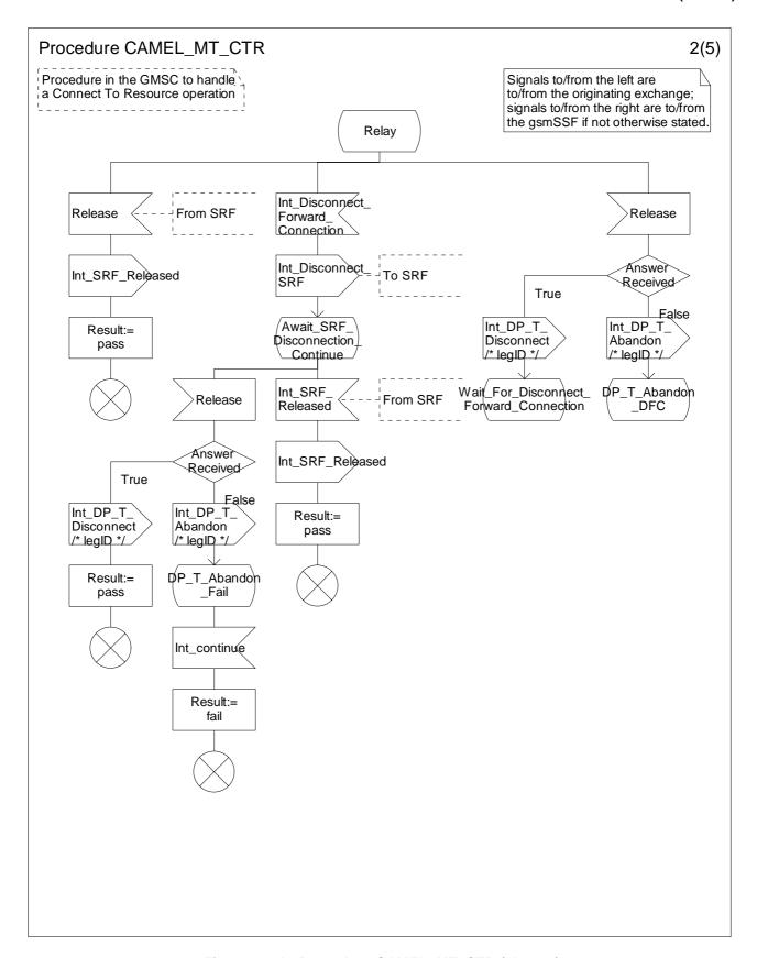
Figure 4.39b: Procedure CAMEL\_MT\_CTR (sheet 2)
