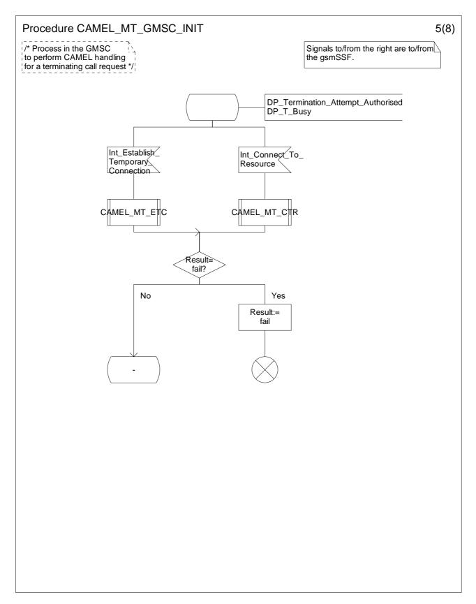
Figure 4.30e: Procedure CAMEL\_MT\_GMSC\_INIT (sheet 5)
