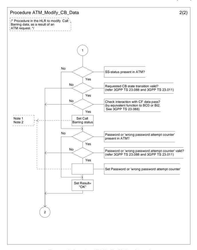
Figure 10.7b: Procedure ATM\_Modify\_CB\_Data (sheet 2)
