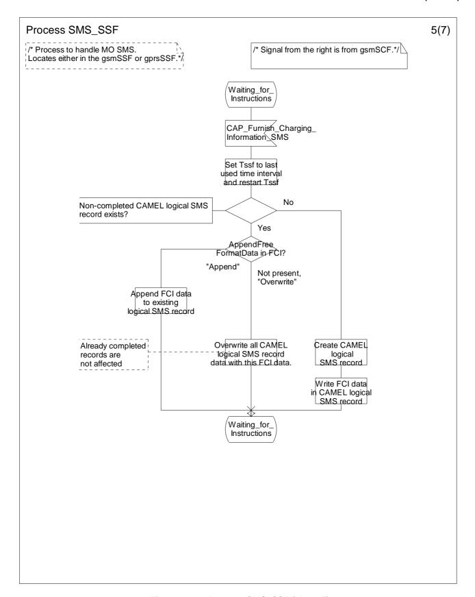
Figure 7.10e: Process SMS\_SSF (sheet 5)
