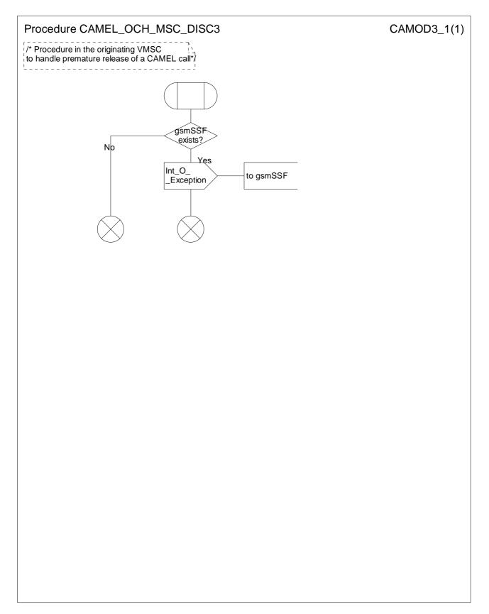
Figure 4.18: Procedure CAMEL\_OCH\_MSC\_DISC3 (sheet 1)
