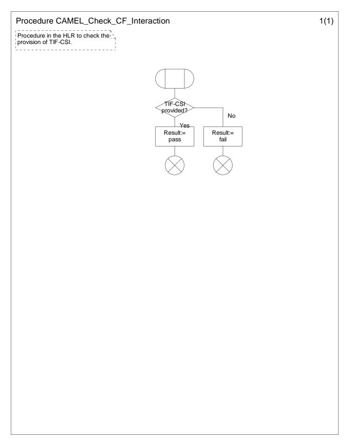
Figure 4.83: Procedure CAMEL\_Check\_CF\_Interaction
