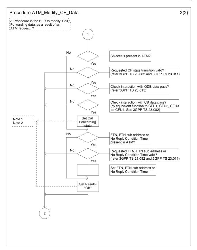
Figure 10.6b: Procedure ATM\_Modify\_CF\_Data (sheet 2)
