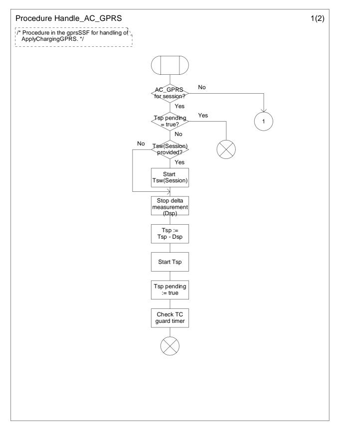
Figure 6.19a: Procedure Handle\_AC\_GPRS (sheet 1)
