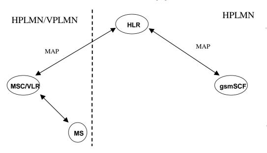
Figure 11.1a: Functional architecture for Any Time Interrogation
