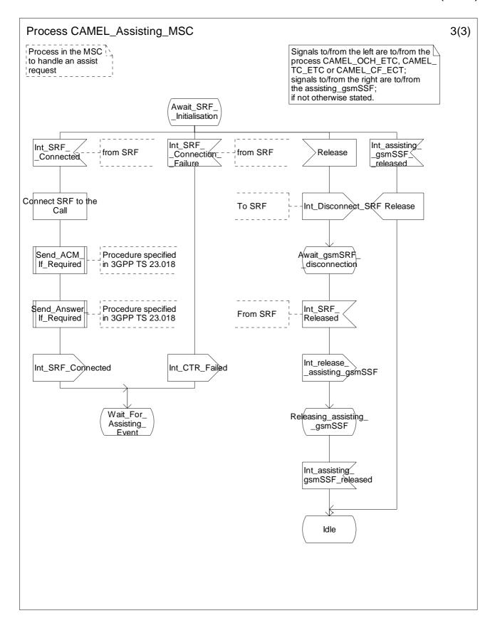
Figure 4.80c: Process CAMEL\_Assisting\_MSC (sheet 3)
