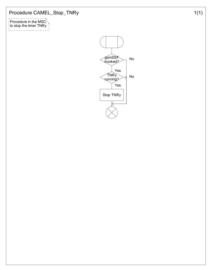
Figure 4.23: Procedure CAMEL\_Stop\_TNRy (sheet 1)
