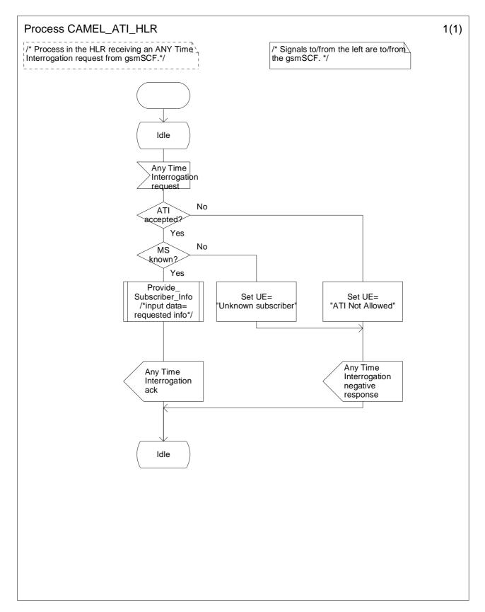
Figure 11.3: Process CAMEL\_ATI\_HLR (sheet 1)
