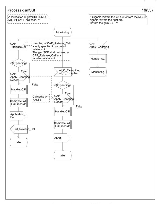
Figure 4.64s: Process gsmSSF (sheet 19)
