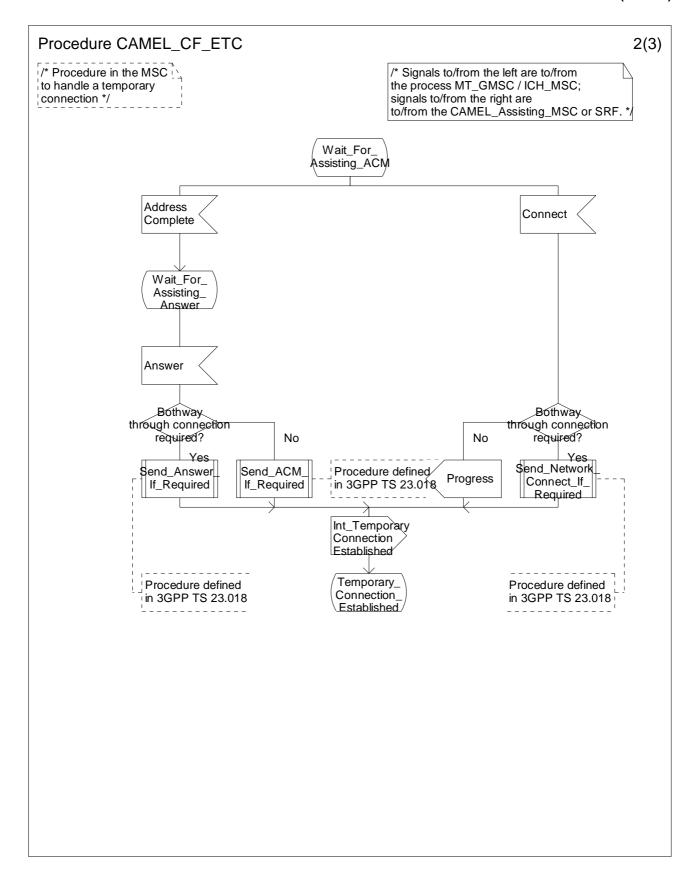
Figure 4.61b: Procedure CAMEL\_CF\_ETC (sheet 2)
