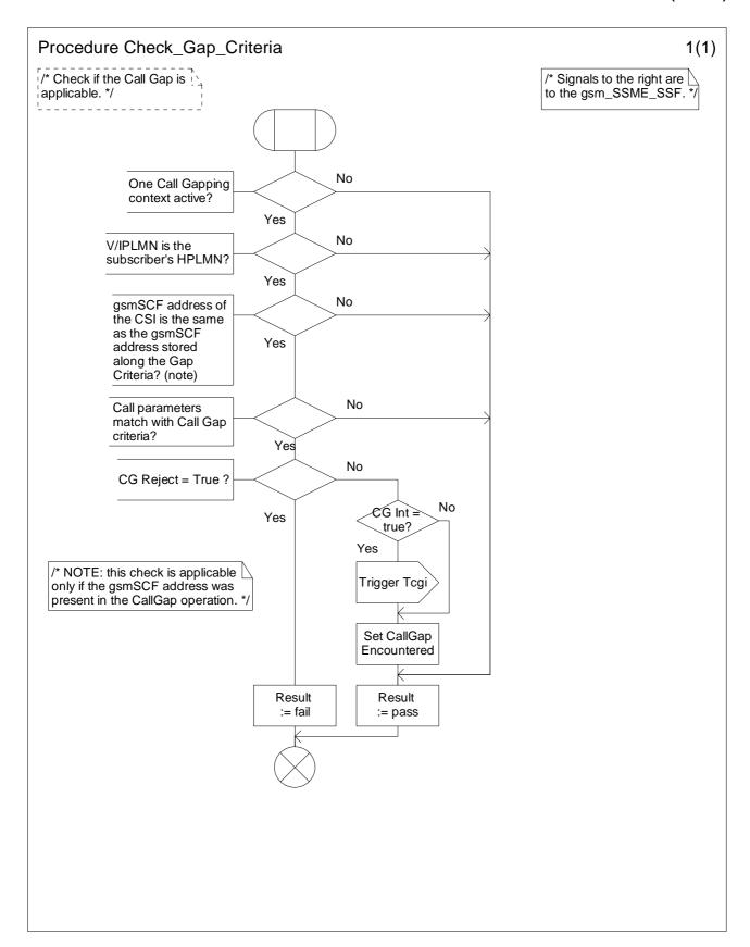
Figure 4.79: Procedure Check\_Gap\_Criteria (sheet 0)
