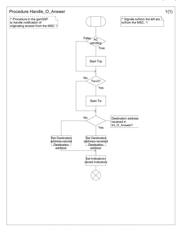
Figure 4.75: Procedure Handle\_O\_Answer (sheet 1)
