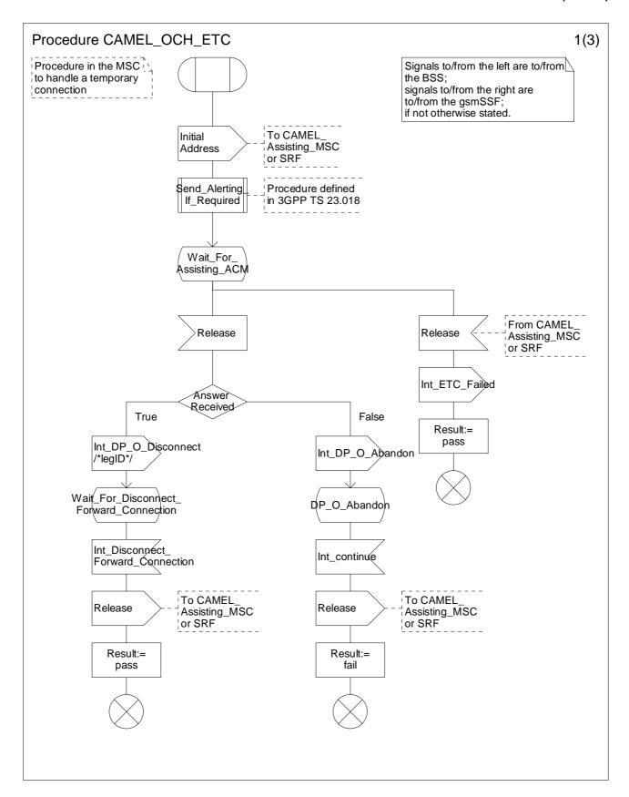
Figure 4.20a: Procedure CAMEL\_OCH\_ETC (sheet 1)
