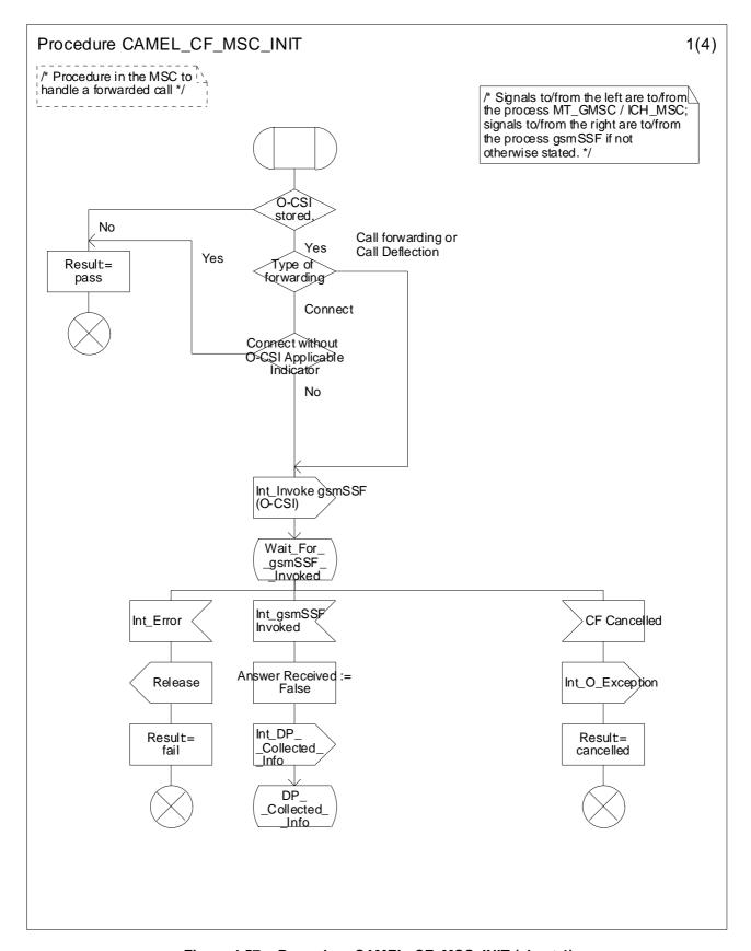
Figure 4.57a: Procedure CAMEL\_CF\_MSC\_INIT (sheet 1)
