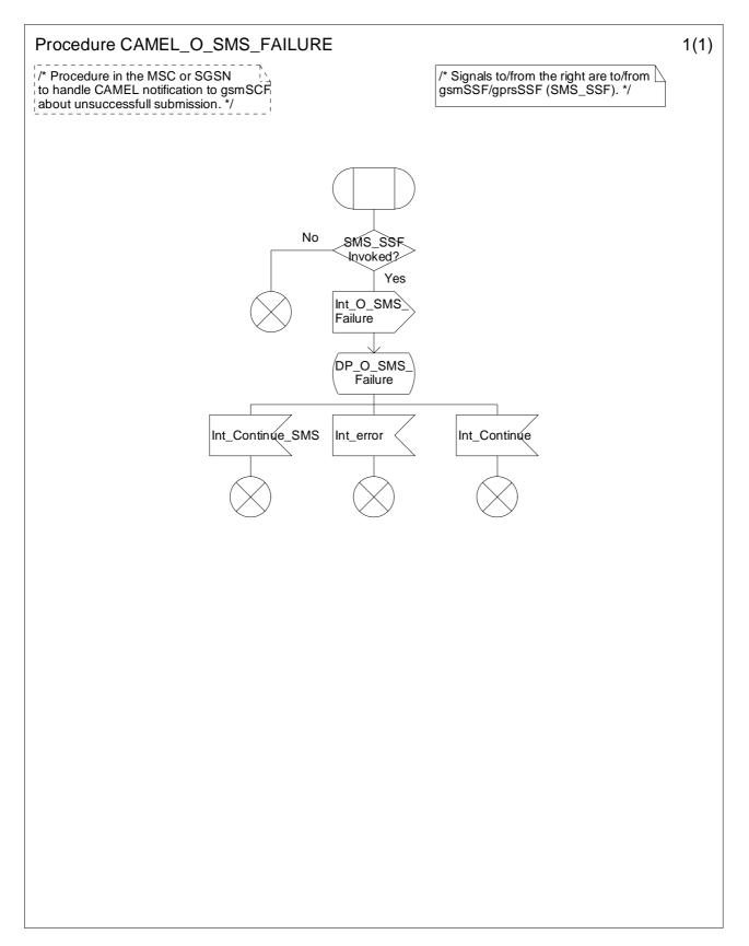
Figure 7.9: Procedure CAMEL\_O\_SMS\_FAILURE (sheet 1)
