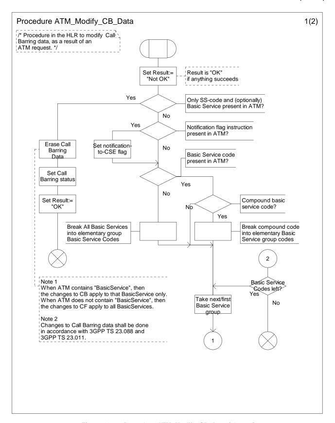
Figure 10.7a: Procedure ATM\_Modify\_CB\_Data (sheet 1)
