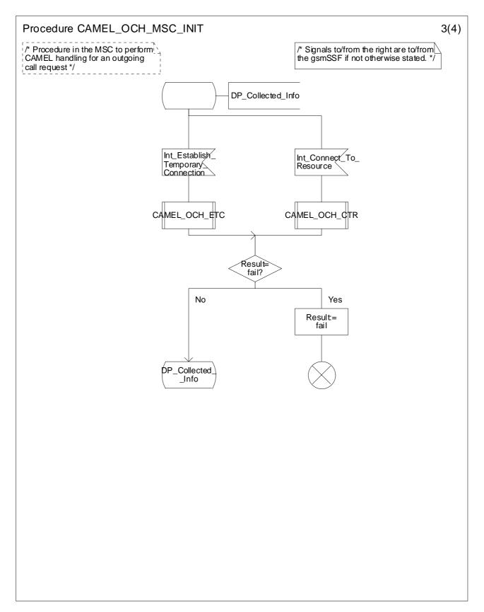
Figure 4.10c: Procedure CAMEL\_OCH\_MSC\_INIT (sheet 3)
