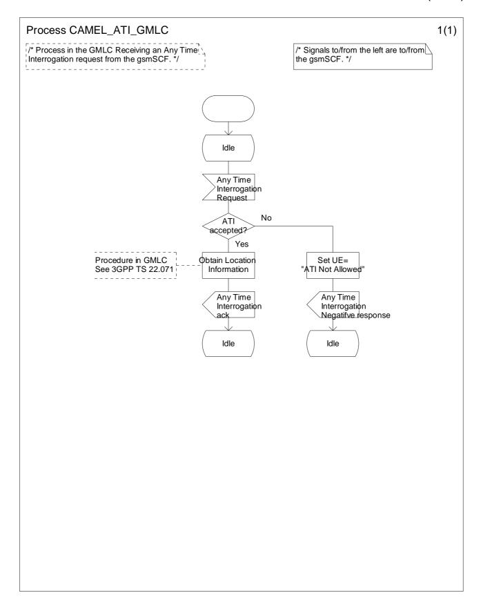
Figure 11.2: Process CAMEL\_ATI\_GMLC (sheet 1)
