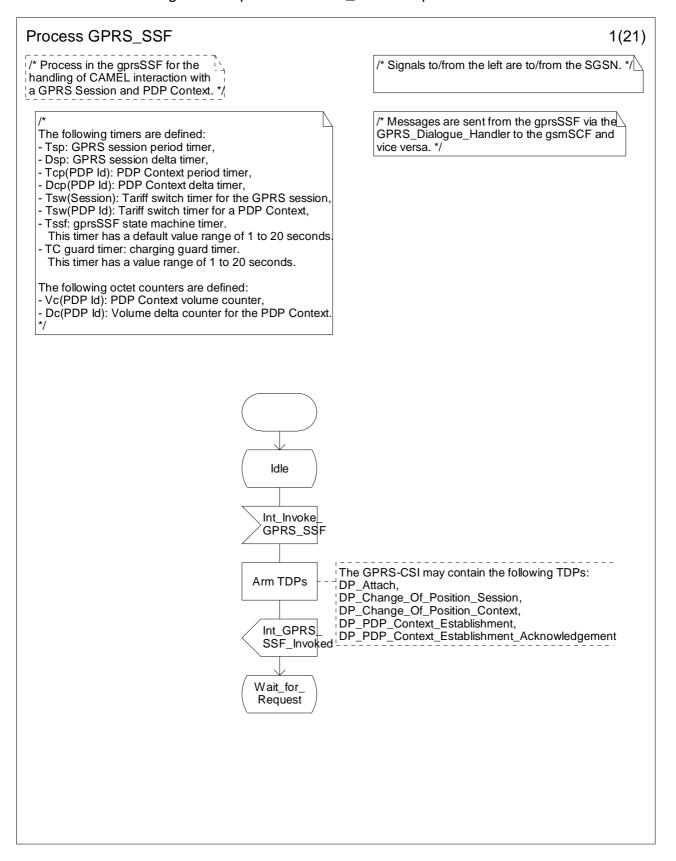
Figure 6.17a: Process GPRS\_SSF (sheet 1)
