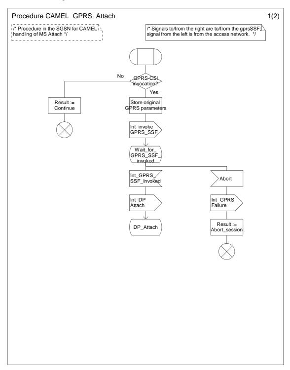
Figure 6.8a: Procedure CAMEL\_GPRS\_Attach (sheet 1)
