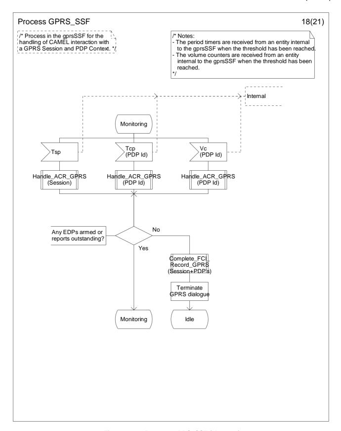
Figure 6.17r: Process GPRS\_SSF (sheet 18)
