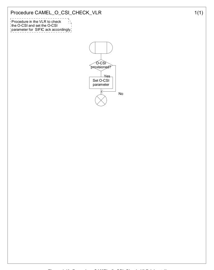
Figure 4.49: Procedure CAMEL\_O\_CSI\_Check\_VLR (sheet 1)
