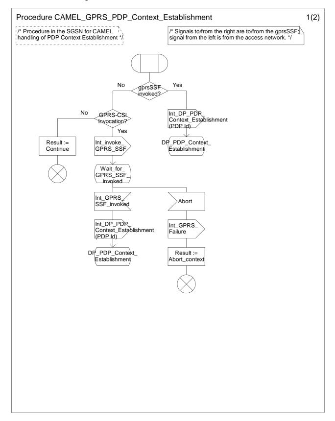
Figure 6.12a: Procedure CAMEL\_GPRS\_PDP\_Context\_Establishment (sheet 1)
