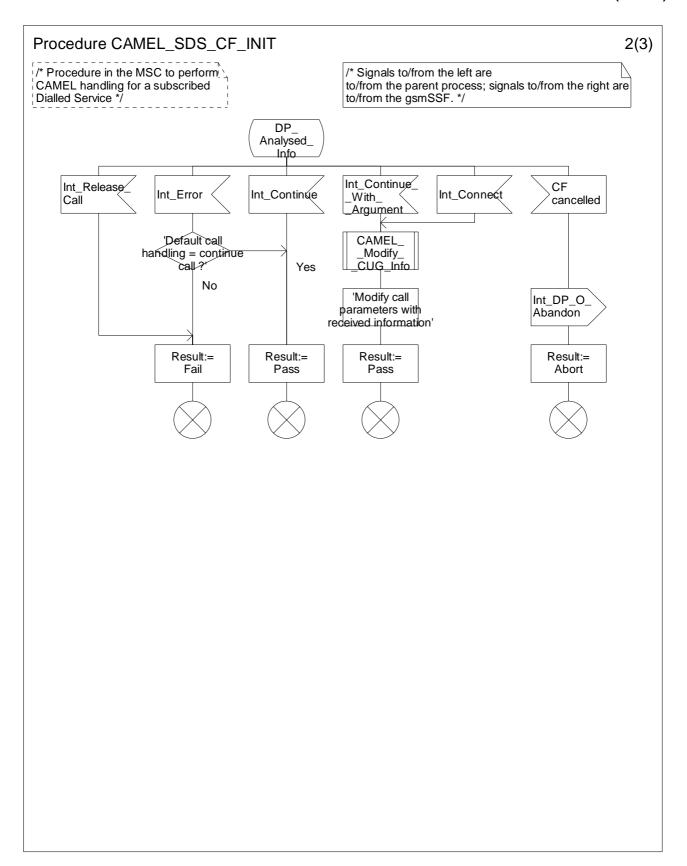
Figure 4.58b: Procedure CAMEL\_SDS\_CF\_INIT (sheet 2)
