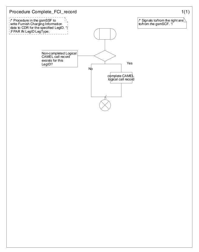
Figure 4.73: Procedure Complete\_FCI\_record (sheet 1)
