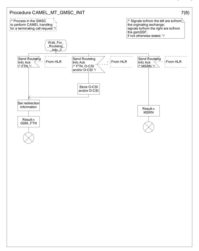
Figure 4.30g: Procedure CAMEL\_MT\_GMSC\_INIT (sheet 7)
