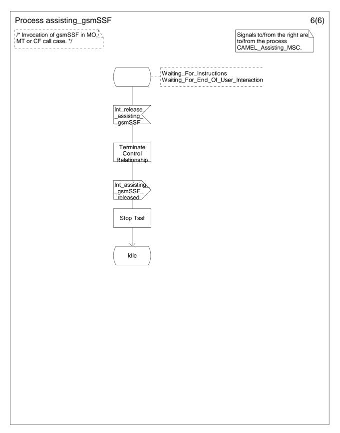
Figure 4.81f: Process Assisting\_gsmSSF (sheet 6)
