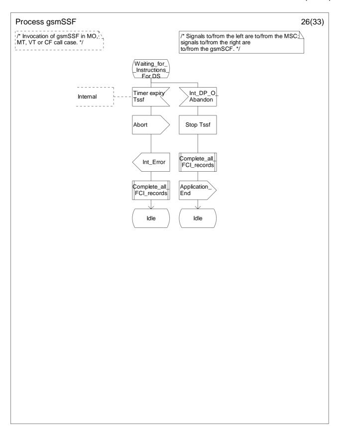
Figure 4.64z: Process gsmSSF (sheet 26)
