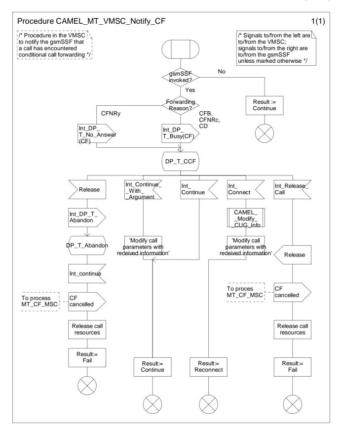
Figure 4.53: Procedure CAMEL\_MT\_VMSC\_Notify\_CF (sheet 0)
