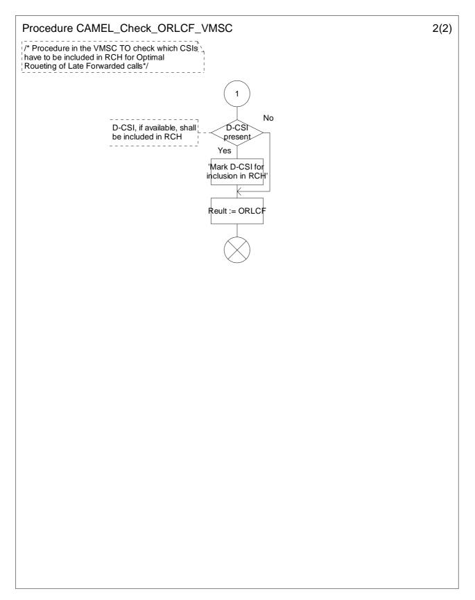
Figure 4.55b: Procedure CAMEL\_Check\_ORLCF\_VMSC (sheet 2)
