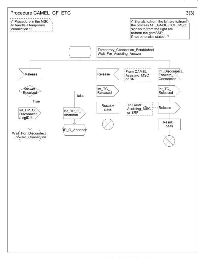
Figure 4.61c: Procedure CAMEL\_CF\_ETC (sheet 3)
