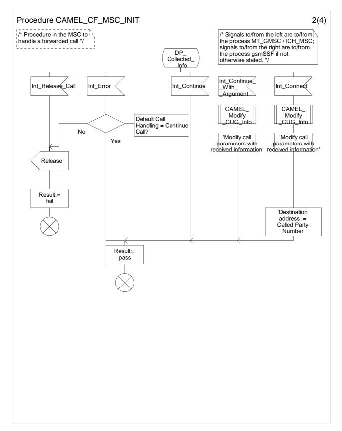
Figure 4.57b: Procedure CAMEL\_CF\_MSC\_INIT (sheet 2)
