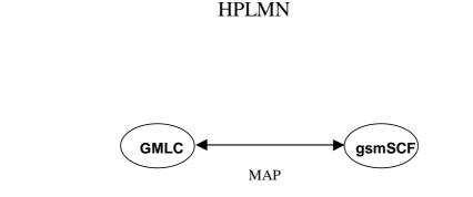
Figure 11.1b: Functional architecture for CAMEL Support of Location Services
