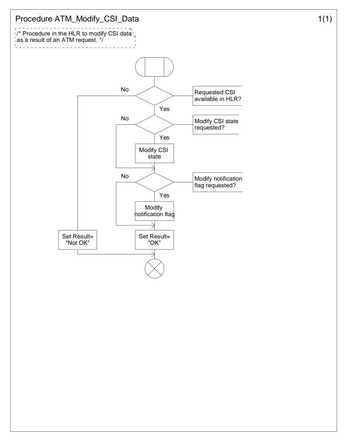
Figure 10.5: Procedure ATM\_Modify\_CSI\_Data (sheet 1)
