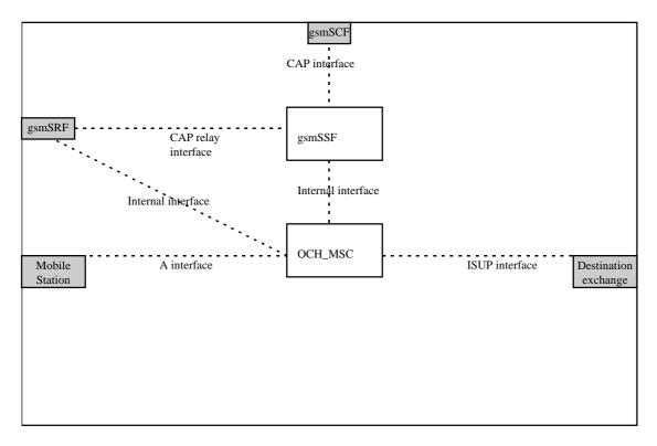
Figure 4.8a: Outgoing case (gsmSSF relay)
