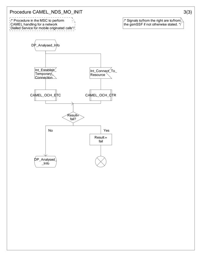
Figure 4.12c: Procedure CAMEL\_NDS\_MO\_INIT (sheet 3)
