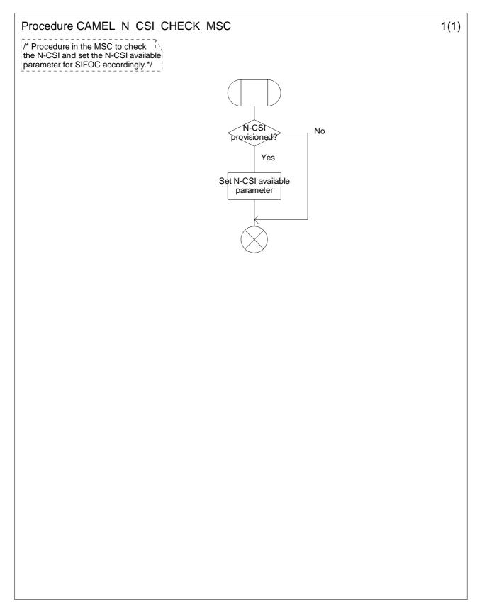
Figure 4.26: Procedure CAMEL\_N\_CSI\_CHECK\_MSC (sheet 1)
