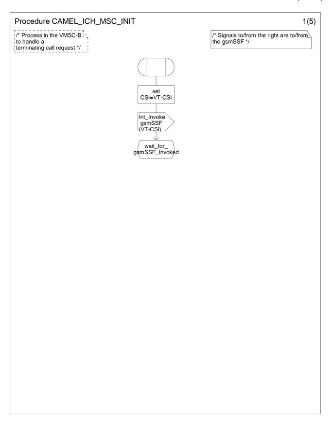
Figure 4.52a: Procedure CAMEL\_ICH\_MSC\_INIT (sheet 1)
