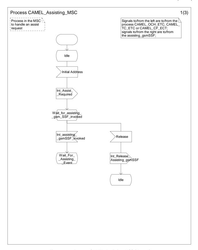
Figure 4.80a: Process CAMEL\_Assisting\_MSC (sheet 1)
