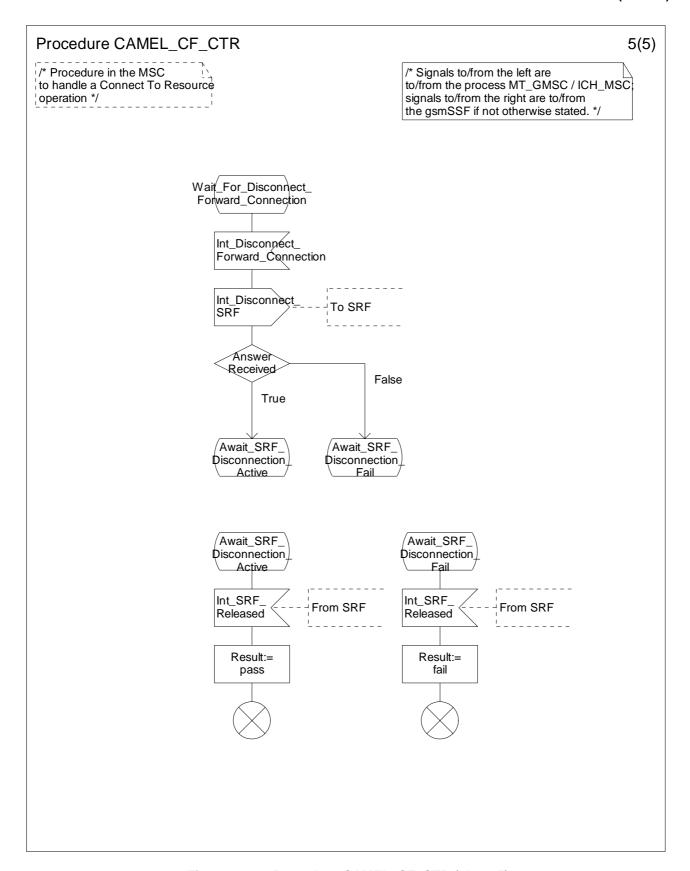
Figure 4.62e: Procedure CAMEL\_CF\_CTR (sheet 5)
