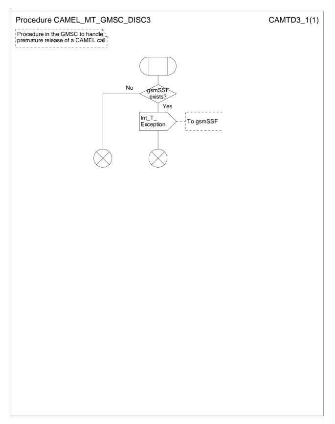
Figure 4.34: Procedure CAMEL\_MT\_GMSC\_DISC3 (sheet 1)
