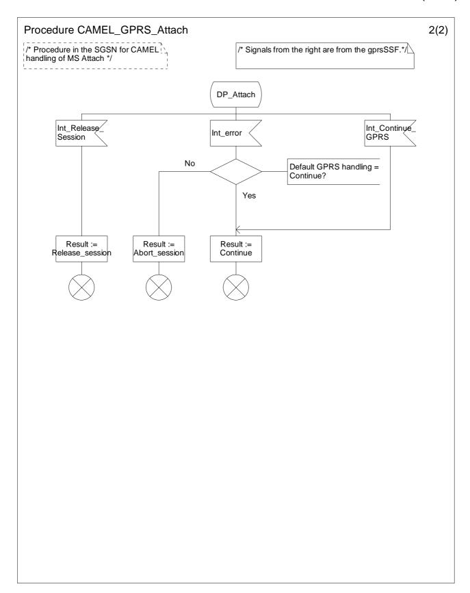
Figure 6.8b: Procedure CAMEL\_GPRS\_Attach (sheet 2)
