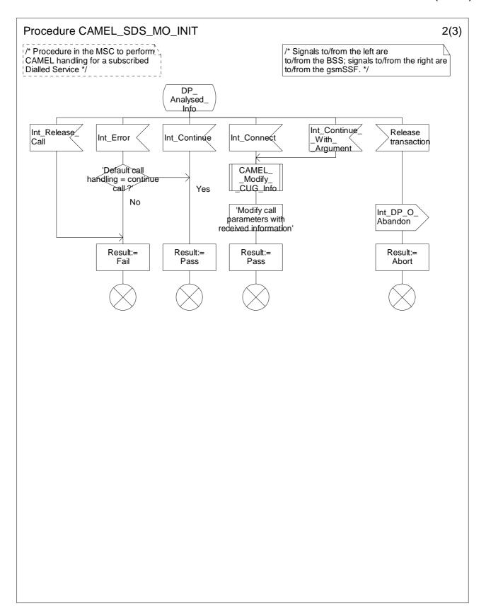
Figure 4.11b: Procedure CAMEL\_SDS\_MO\_INIT (sheet 2)
