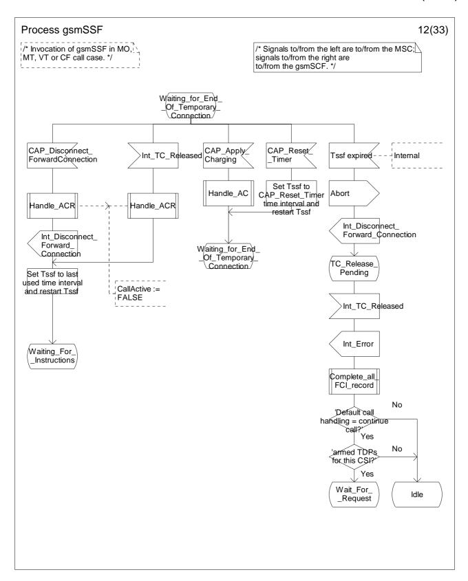
Figure 4.64I: Process gsmSSF (sheet 12)
