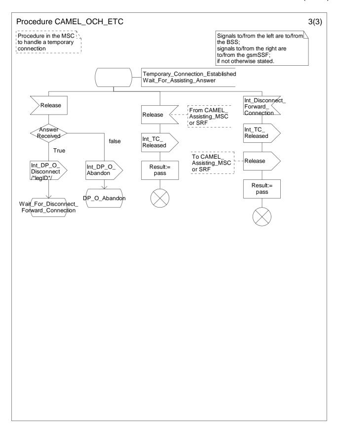
Figure 4.20c: Procedure CAMEL\_OCH\_ETC (sheet 3)
