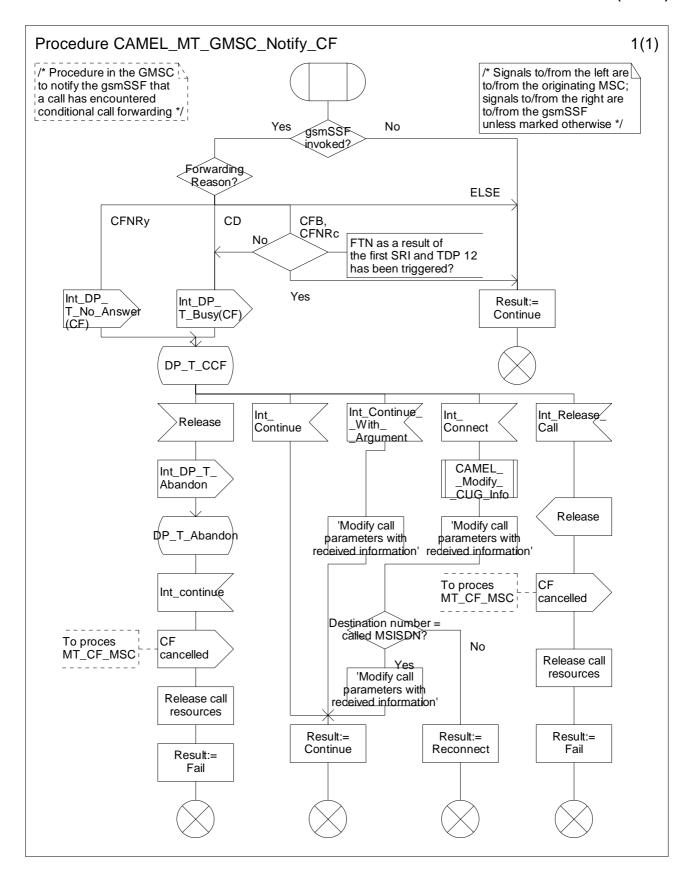
Figure 4.40: Procedure CAMEL\_MT\_GMSC\_Notify\_CF (sheet 0)
