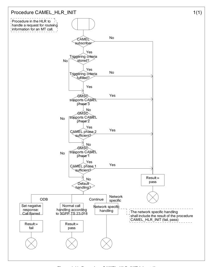
Figure 4.41: Procedure CAMEL\_HLR\_INIT (sheet 1)
