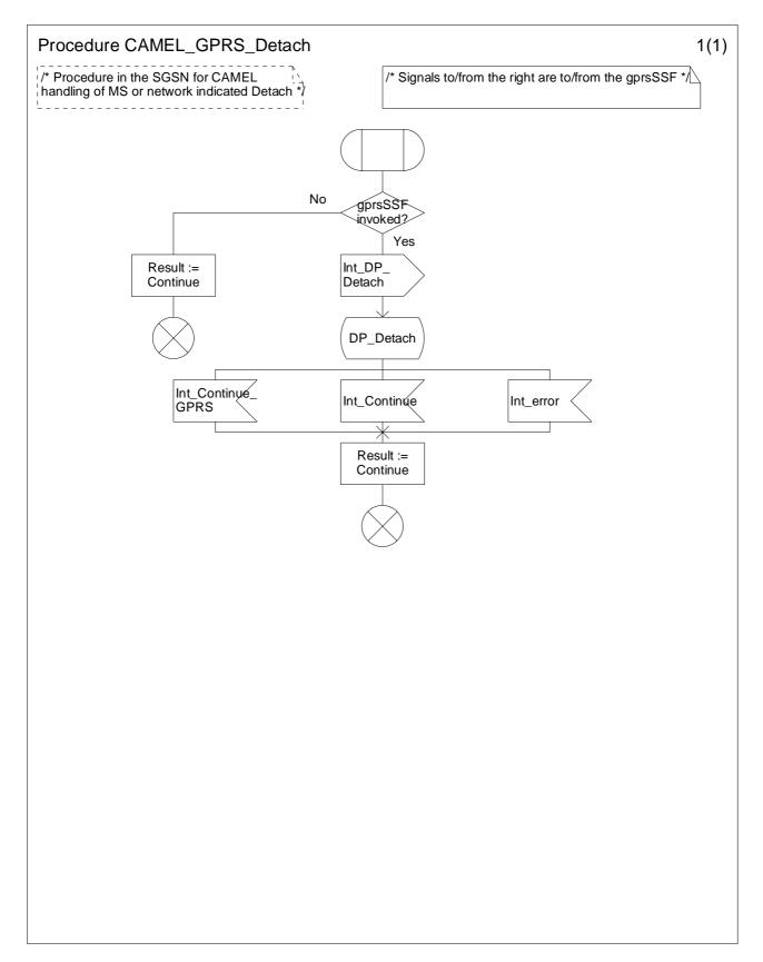
Figure 6.9: Procedure CAMEL\_GPRS\_Detach (sheet 1)
