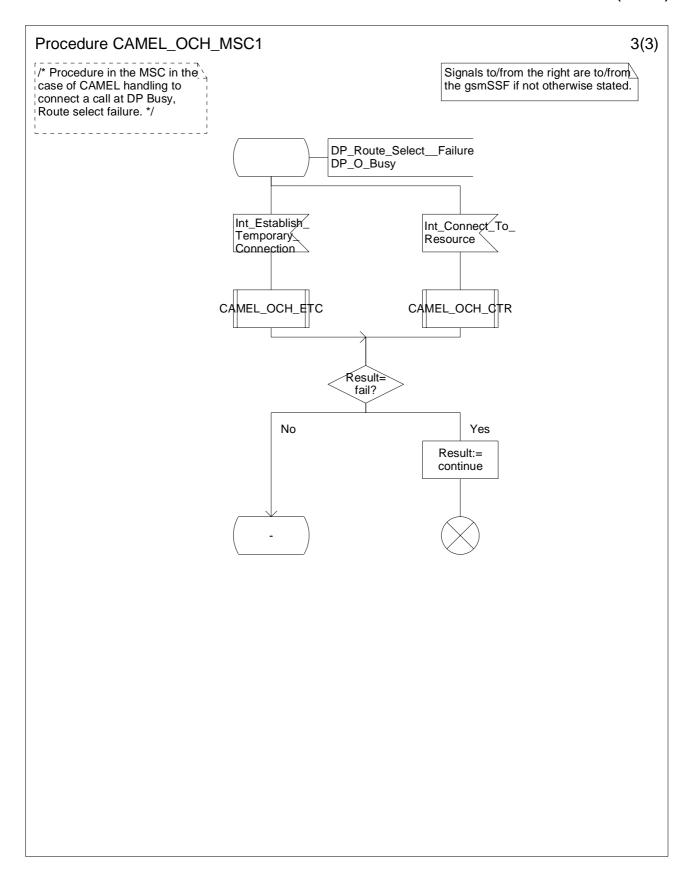
Figure 4.14c: Procedure CAMEL\_OCH\_MSC1 (sheet 3)
