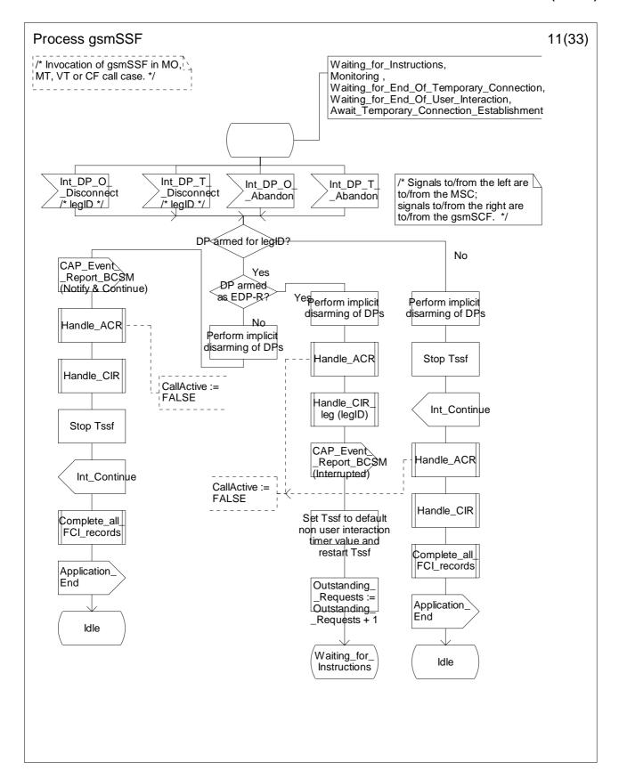
Figure 4.64k: Process gsmSSF (sheet 11)
