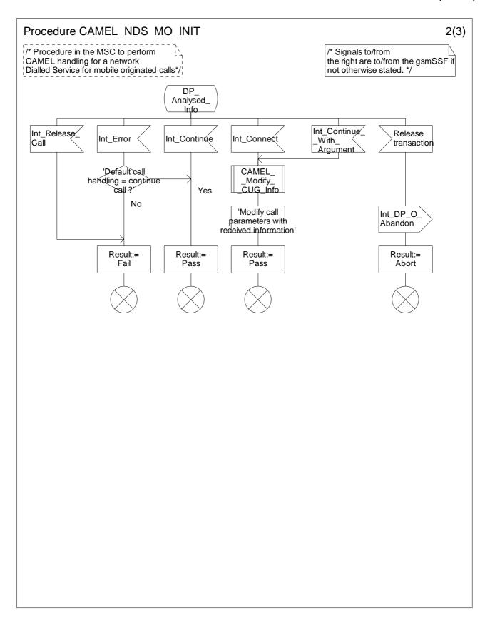
Figure 4.12b: Procedure CAMEL\_NDS\_MO\_INIT (sheet 2)
