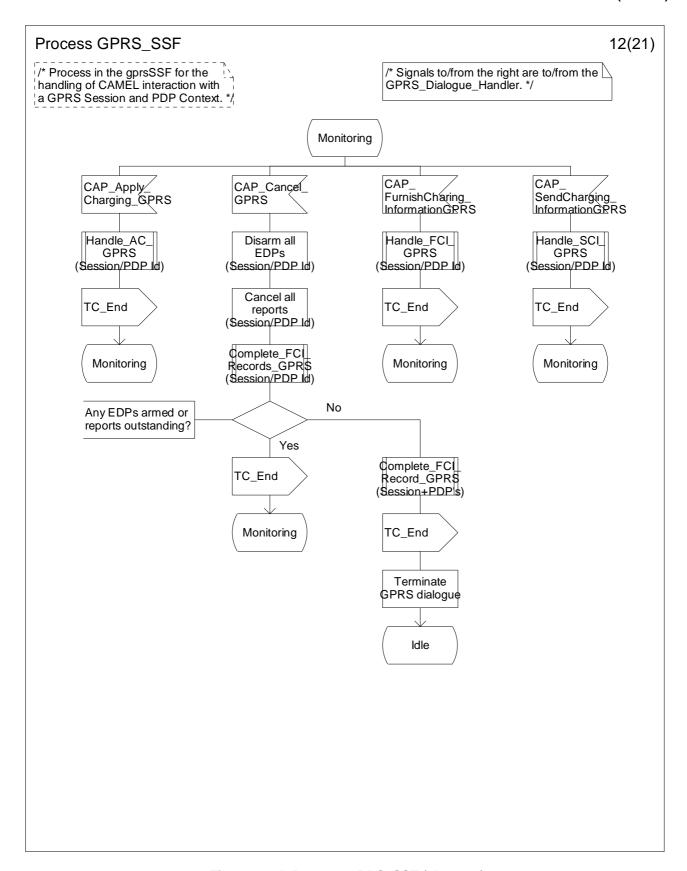
Figure 6.17I: Process GPRS\_SSF (sheet 12)
