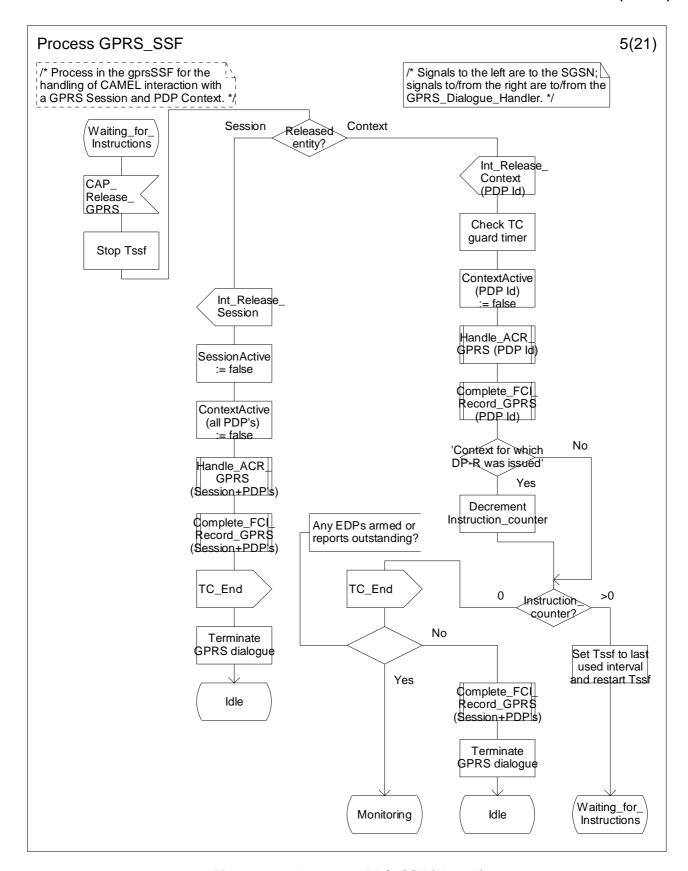
Figure 6.17e: Process GPRS\_SSF (sheet 5)
