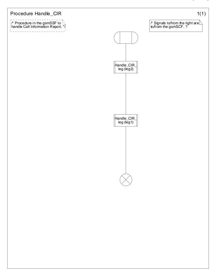
Figure 4.71: Procedure Handle\_CIR (sheet 1)
