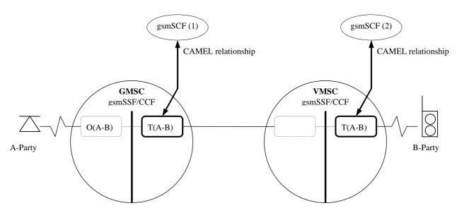
Figure 4.6: BCSM Scenario for Mobile Terminated Calls at the GMSC / VMSC
