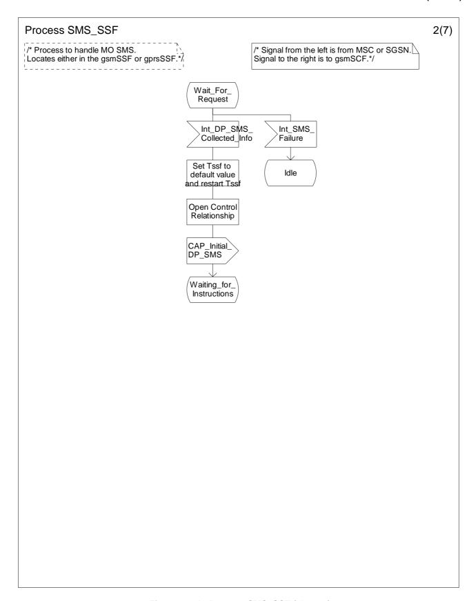
Figure 7.10b: Process SMS\_SSF (sheet 2)
