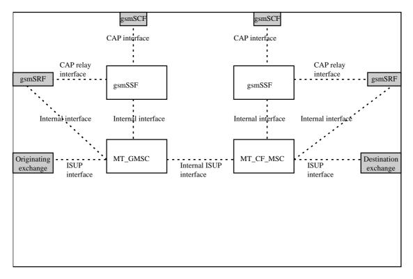
Figure 4.8c: Terminating GMSC case (gsmSSF relay)
