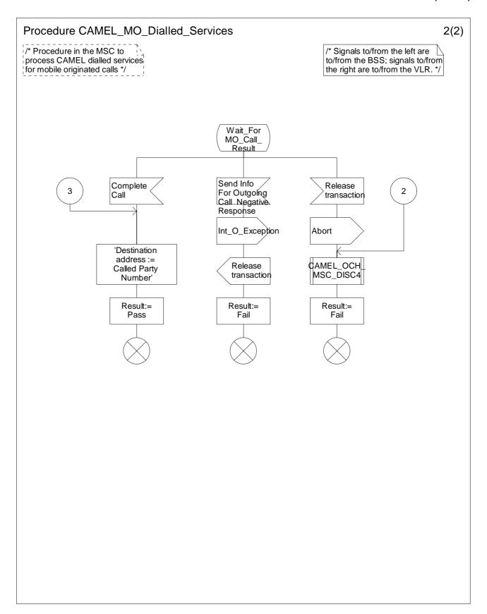
Figure 4.9b: Procedure CAMEL\_MO\_Dialled\_Services (sheet 2)
