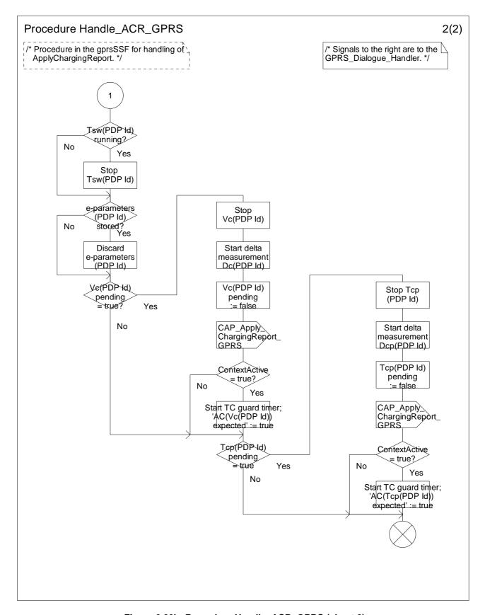
Figure 6.20b: Procedure Handle\_ACR\_GPRS (sheet 2)
