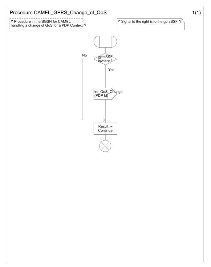
Figure 6.14: Procedure CAMEL\_GPRS\_Change\_Of\_QoS (sheet 1)
