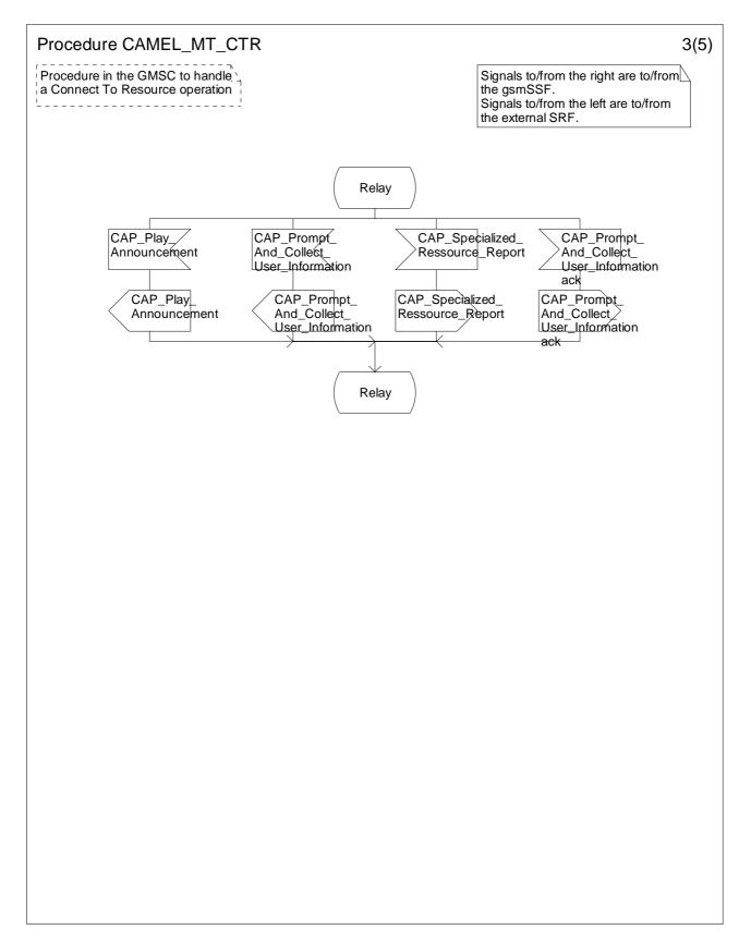
Figure 4.39c: Procedure CAMEL\_MT\_CTR (sheet 3)
