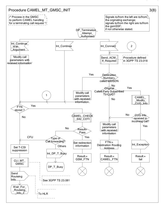
Figure 4.30c: Procedure CAMEL\_MT\_GMSC\_INIT (sheet 3)
