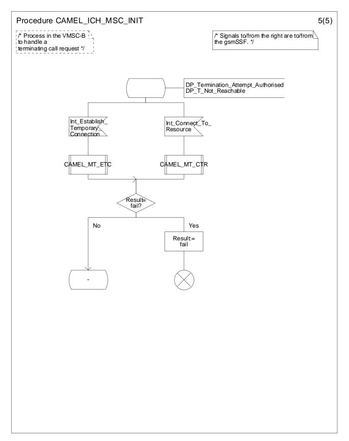
Figure 4.52e: Procedure CAMEL\_ICH\_MSC\_INIT (sheet 5)
