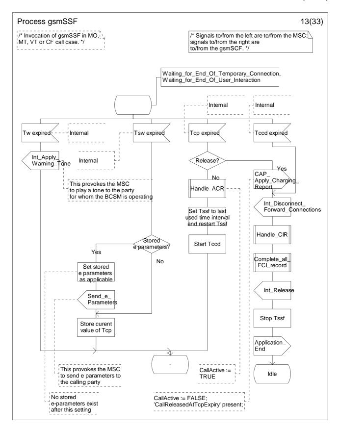
Figure 4.64m: Process gsmSSF (sheet 13)
