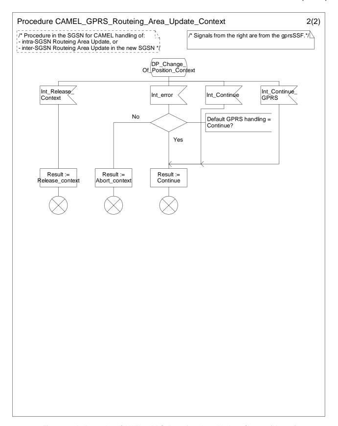
Figure 6.11b: Procedure CAMEL\_GPRS\_Routeing\_Area\_Update\_Context (sheet 2)
