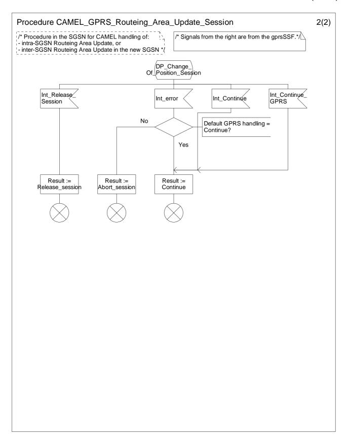
Figure 6.10b: Procedure CAMEL\_GPRS\_Routeing\_Area\_Update\_Session (sheet 2)
