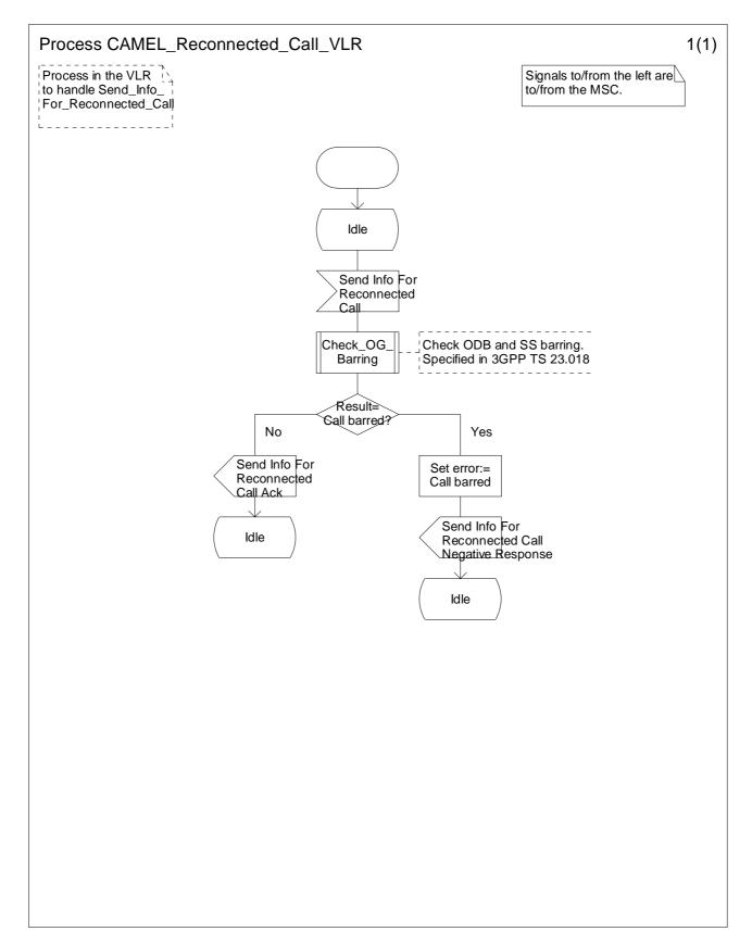
Figure 4.28: Process CAMEL\_Reconnected\_Call\_VLR (sheet 1)
