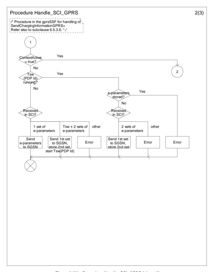
Figure 6.23b: Procedure Handle\_SCI\_GPRS (sheet 2)
