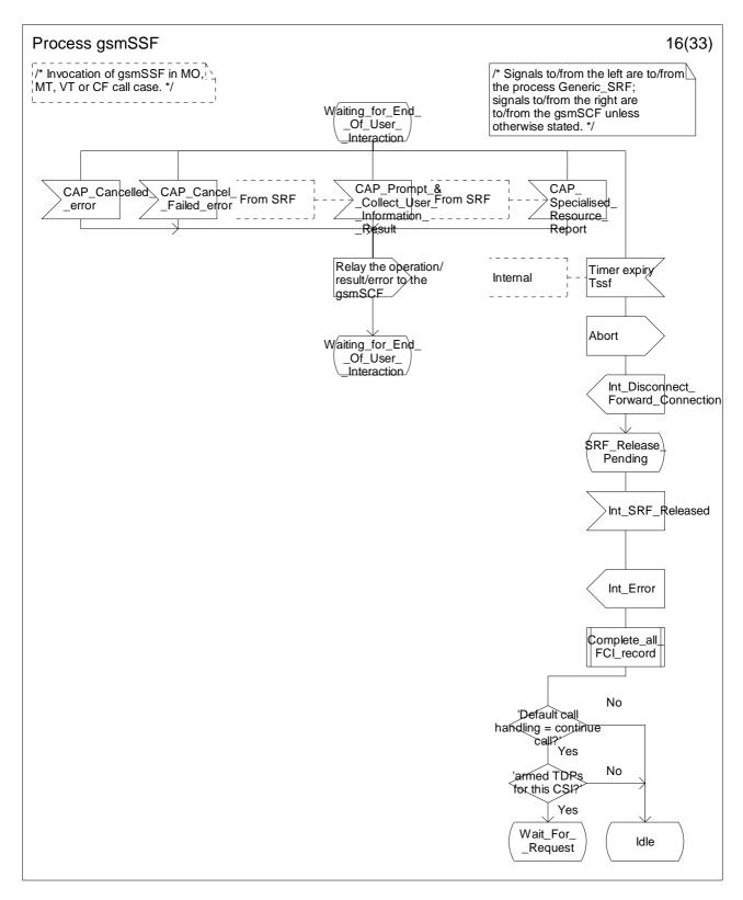
Figure 4.64p: Process gsmSSF (sheet 16)
