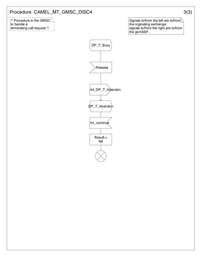
Figure 4.35c: Procedure CAMEL\_MT\_GMSC\_DISC4 (sheet 3)
