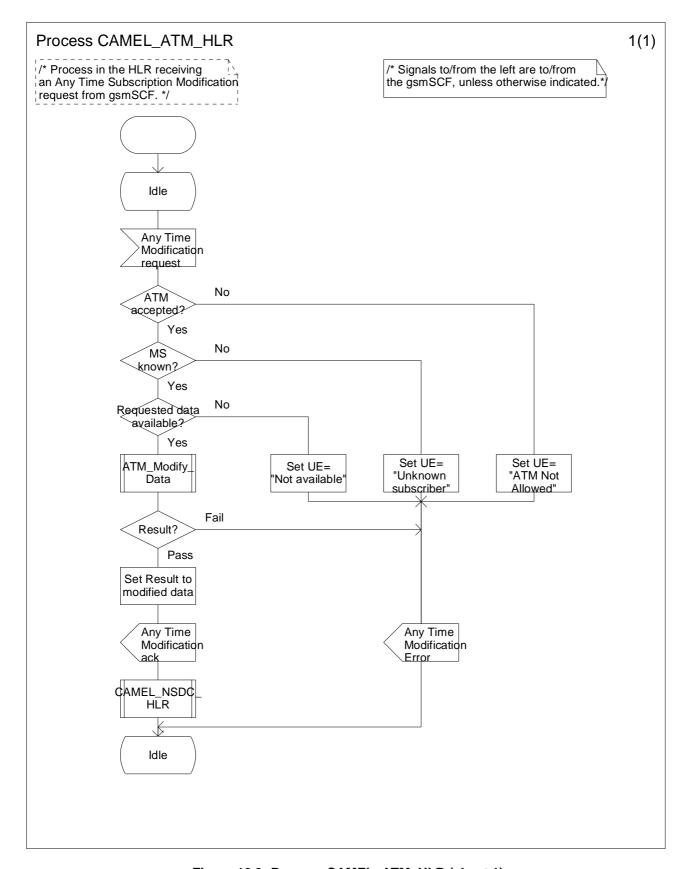
Figure 10.3: Process CAMEL\_ATM\_HLR (sheet 1)
