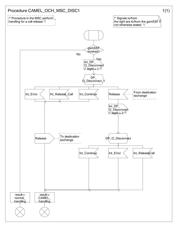
Figure 4.16: Procedure CAMEL\_OCH\_MSC\_DISC1 (sheet 1)
