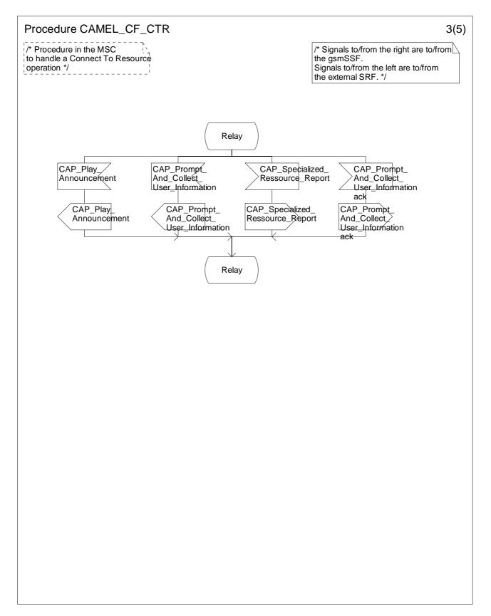
Figure 4.62c: Procedure CAMEL\_CF\_CTR (sheet 3)
