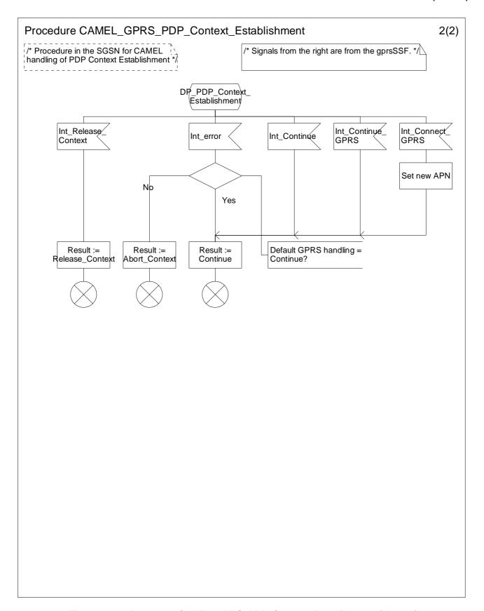
Figure 6.12b: Procedure CAMEL\_GPRS\_PDP\_Context\_Establishment (sheet 2)
