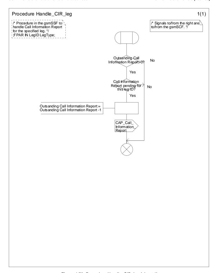
Figure 4.72: Procedure Handle\_CIR\_leg (sheet 1)
