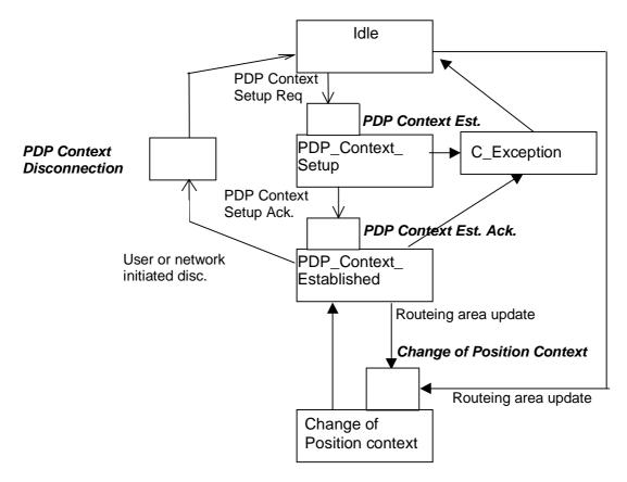
Figure 6.4: GPRS PDP Context State Model
