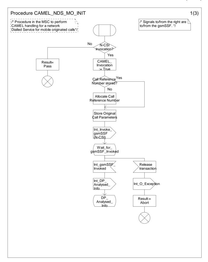
Figure 4.12a: Procedure CAMEL\_NDS\_MO\_INIT (sheet 1)
