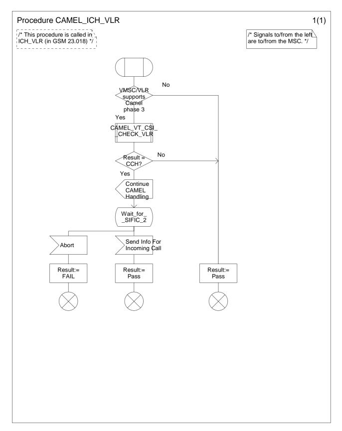
Figure 4.48: Procedure CAMEL\_ICH\_VLR (sheet 1)
