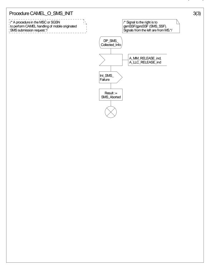
Figure 7.7c: Procedure CAMEL\_O\_SMS\_INIT (sheet 3)
