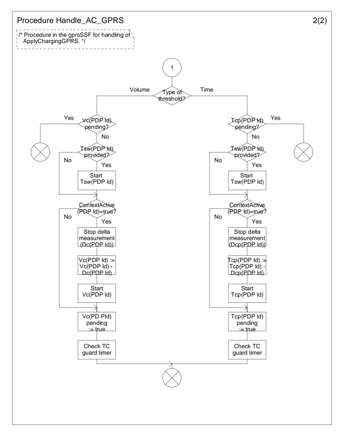
Figure 6.19b: Procedure Handle\_AC\_GPRS (sheet 2)
