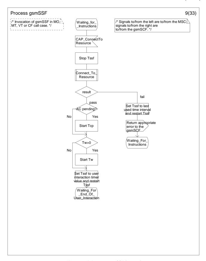
Figure 4.64i: Process gsmSSF (sheet 9)
