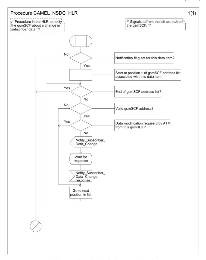
Figure 10.8: Procedure CAMEL\_NSDC\_HLR (sheet1)
