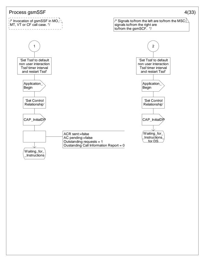
Figure 4.64d: Process gsmSSF (sheet 4)
