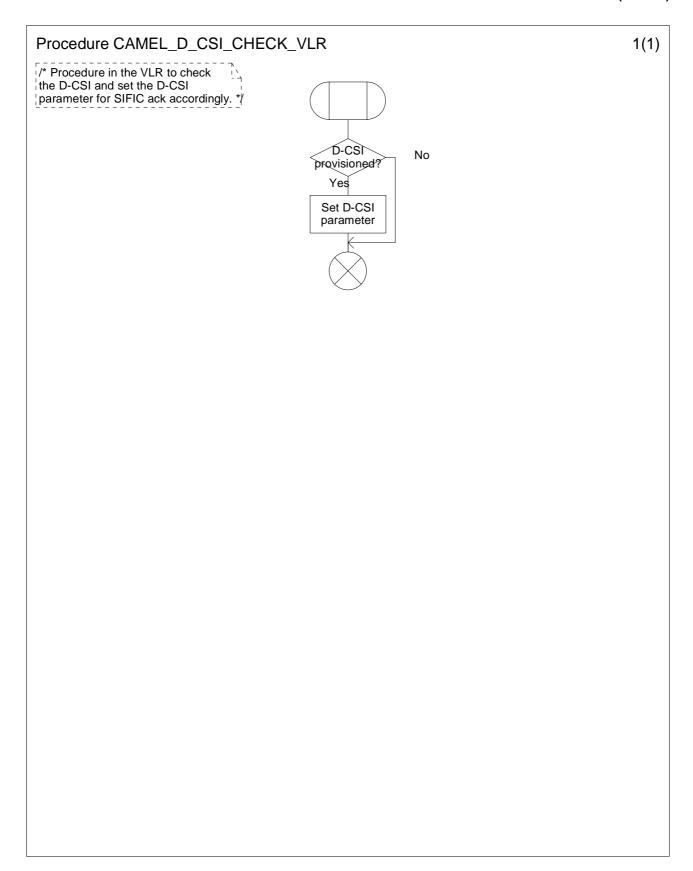
Figure 4.50: Procedure CAMEL\_D\_CSI\_Check\_VLR (sheet 1)
