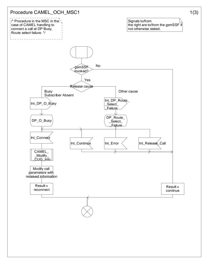
Figure 4.14a: Procedure CAMEL\_OCH\_MSC1 (sheet 1)
