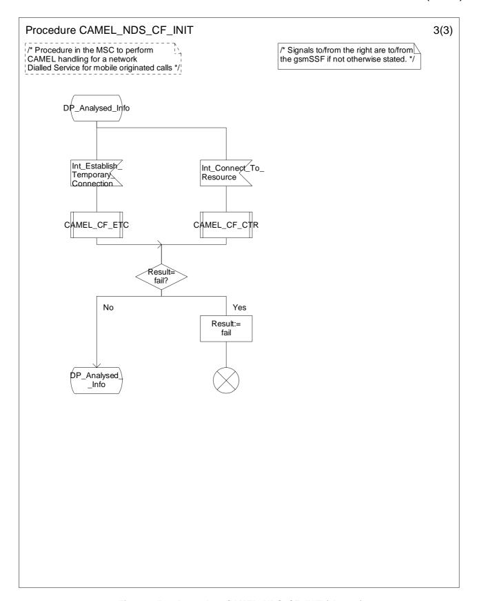
Figure 4.59c: Procedure CAMEL\_NDS\_CF\_INIT (sheet 3)
