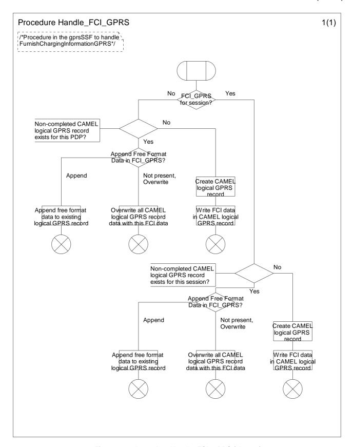
Figure 6.21: Procedure Handle\_FCI\_GPRS (sheet 0)
