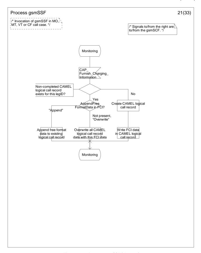
Figure 4.64u: Process gsmSSF (sheet 21)
