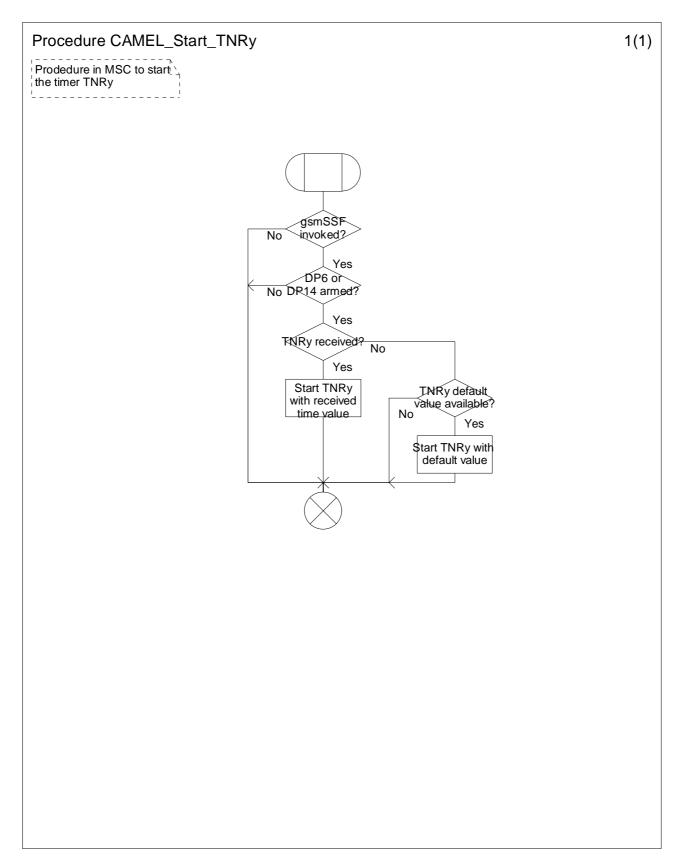
Figure 4.22: Procedure CAMEL\_Start\_TNRy (sheet 1)
