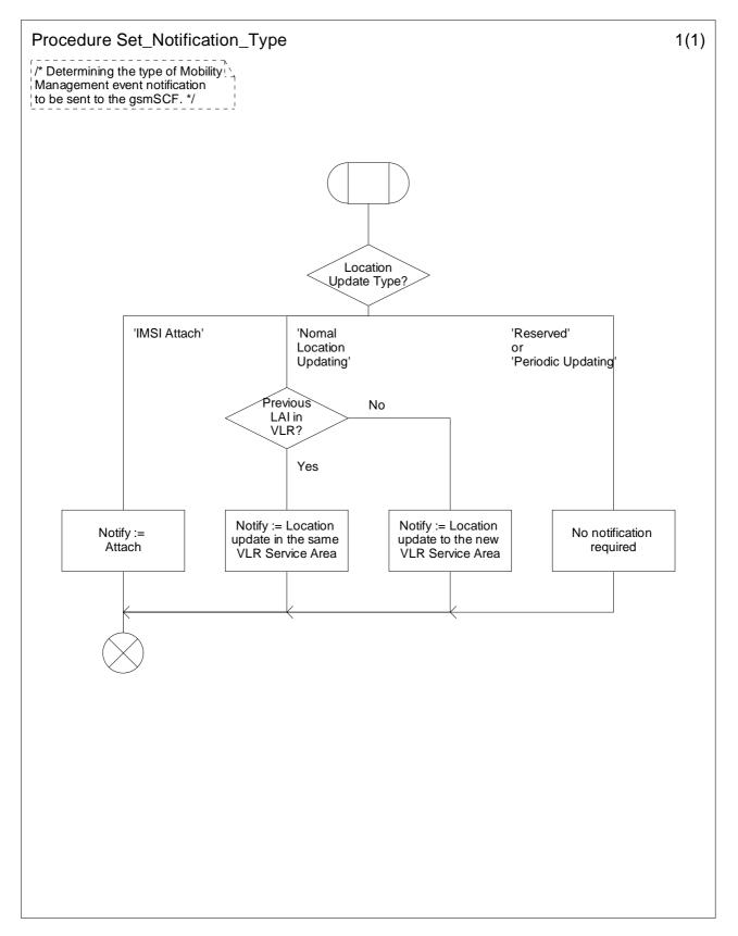
Figure 9.3: Procedure Set\_Notification\_Type (sheet 1)
