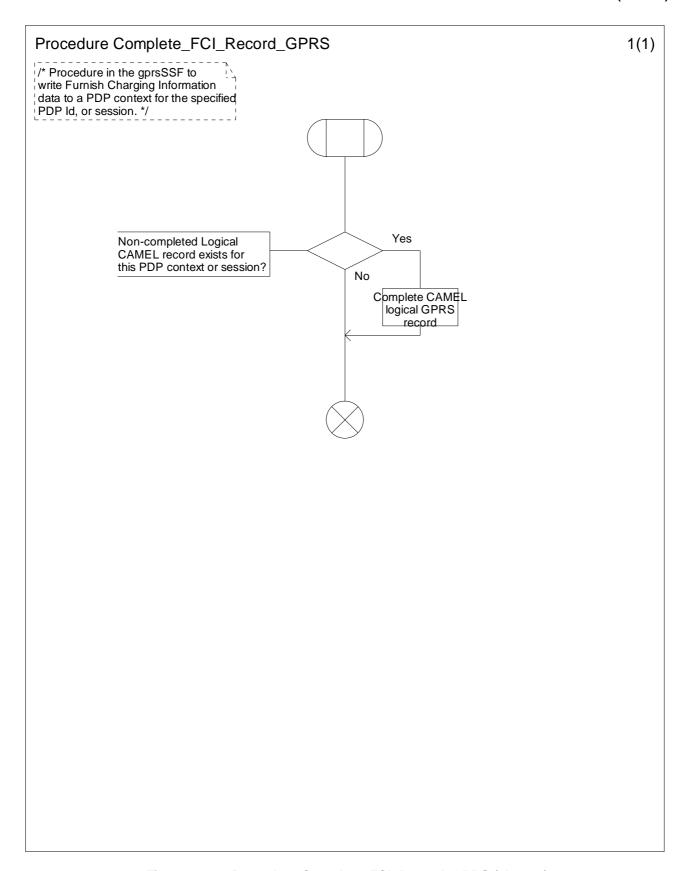
Figure 6.22a: Procedure Complete\_FCI\_Record\_GPRS (sheet 1)
