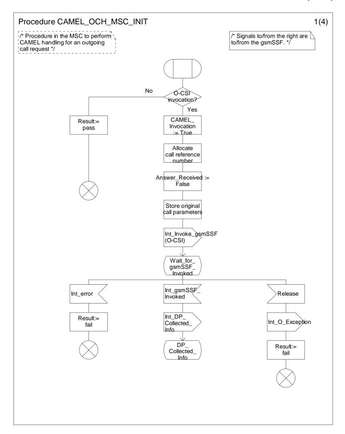
Figure 4.10a: Procedure CAMEL\_OCH\_MSC\_INIT (sheet 1)
