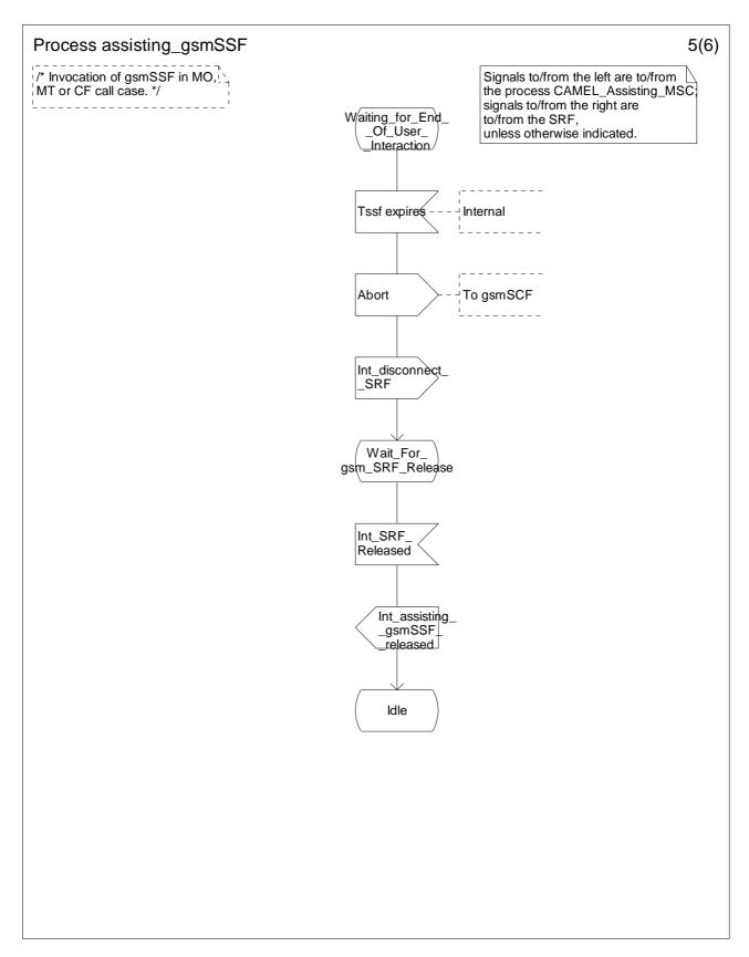
Figure 4.81e: Process Assisting\_gsmSSF (sheet 5)
