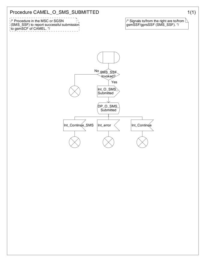
Figure 7.8: Procedure CAMEL\_O\_SMS\_SUBMITTED (sheet 1)
