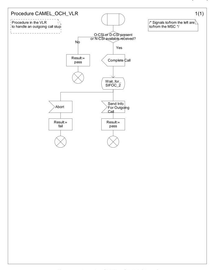
Figure 4.27: Procedure CAMEL\_OCH\_VLR (sheet 1)
