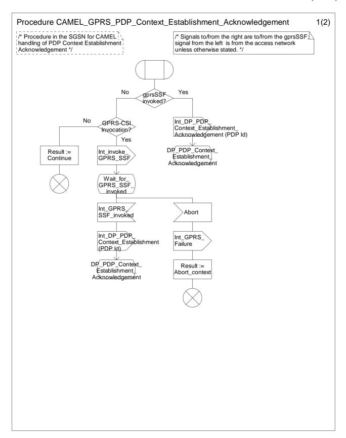
Figure 6.13a: Procedure CAMEL\_GPRS\_PDP\_Context\_Establishment\_Acknowledgement (sheet 1)
