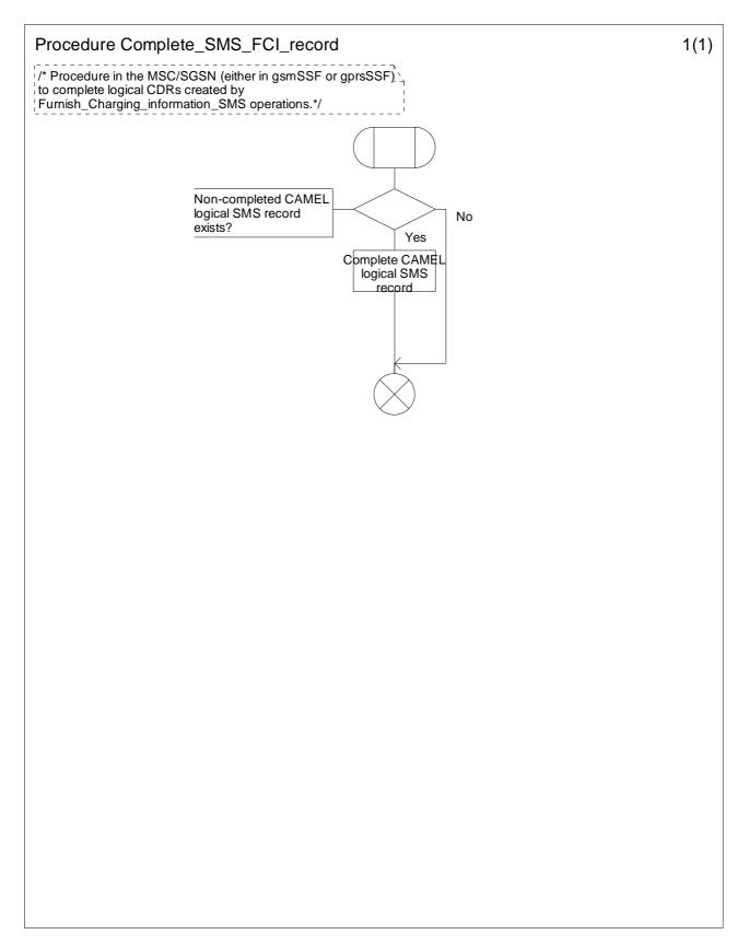
Figure 7.11: Procedure Complete\_SMS\_FCI\_record (sheet 1)
