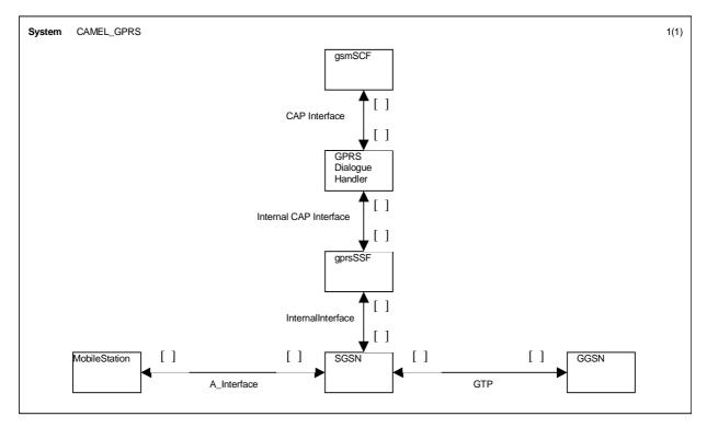
Figure 6.7: Architecture for CAMEL/GPRS interworking
