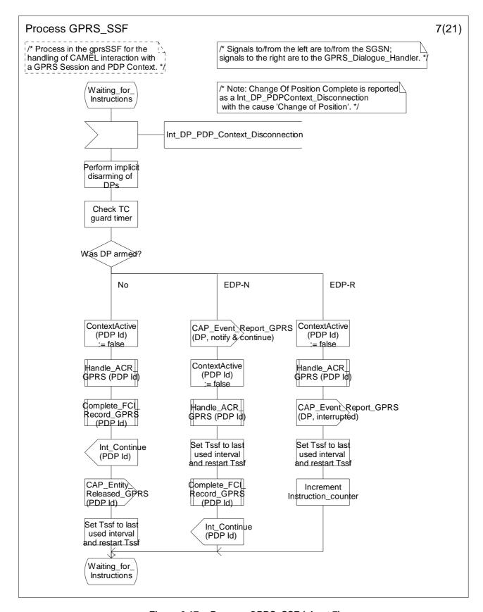
Figure 6.17g: Process GPRS\_SSF (sheet 7)
