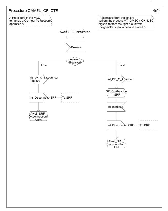
Figure 4.62d: Procedure CAMEL\_CF\_CTR (sheet 4)
