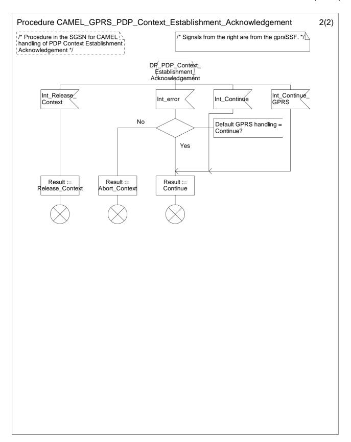
Figure 6.13b: Procedure CAMEL\_GPRS\_PDP\_Context\_Establishment\_Acknowledgement (sheet 2)
