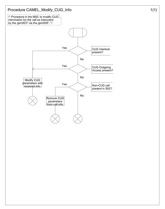
Figure 4.25: Procedure CAMEL\_Modify\_CUG\_Info (sheet 1)
