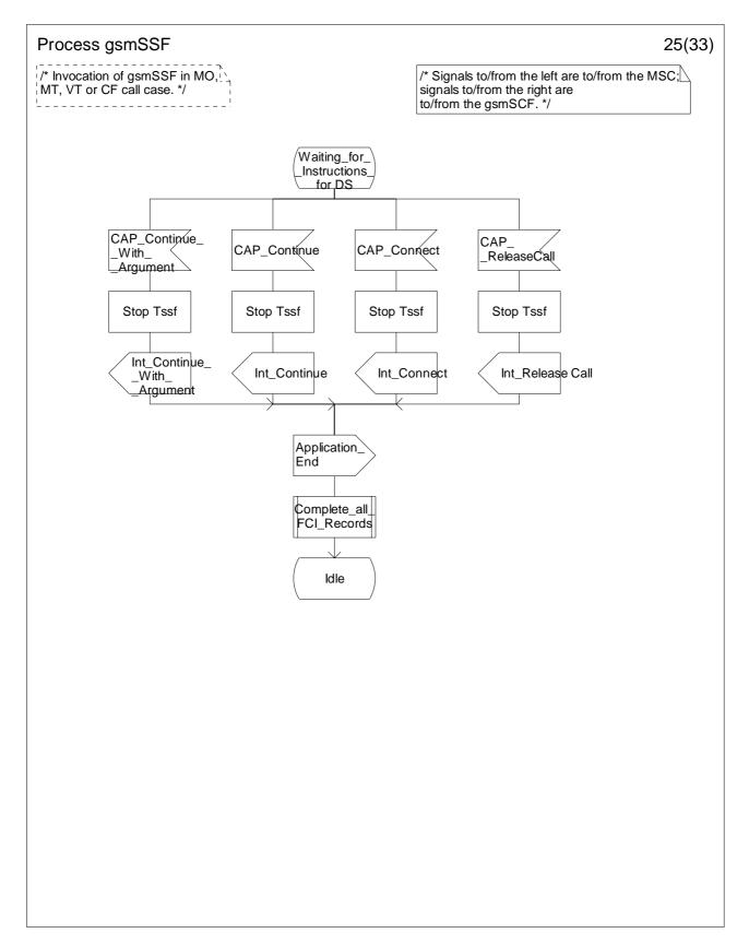
Figure 4.64y: Process gsmSSF (sheet 25)
