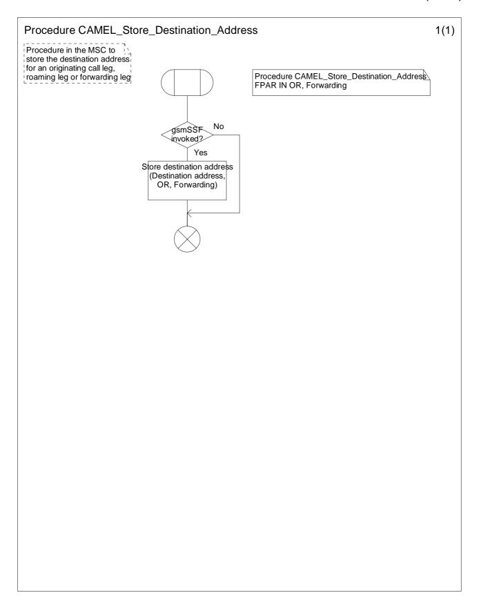
Figure 4.24: Procedure CAMEL\_Store\_Destination\_Address (sheet 1)
