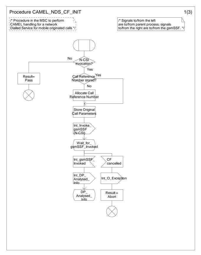
Figure 4.59a: Procedure CAMEL\_NDS\_CF\_INIT (sheet 1)
