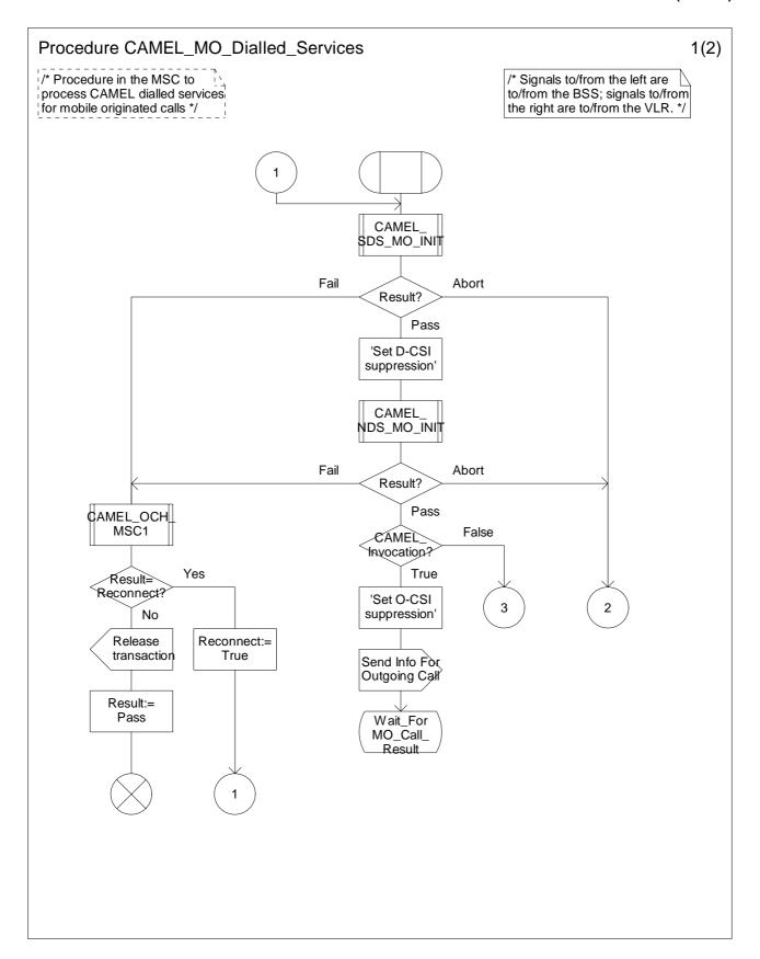
Figure 4.9a: Procedure CAMEL\_MO\_Dialled\_Services (sheet 1)
