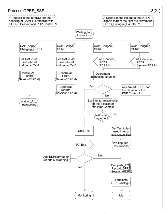
Figure 6.17c: Process GPRS\_SSF (sheet 3)
