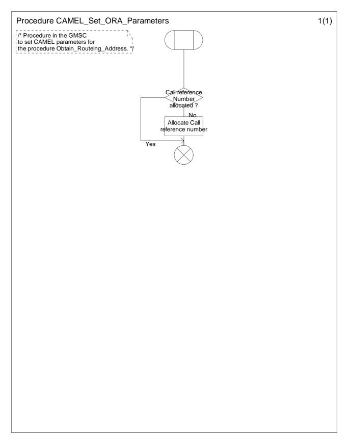
Figure 4.29: Procedure CAMEL\_Set\_ORA\_Parameters (sheet 1)
