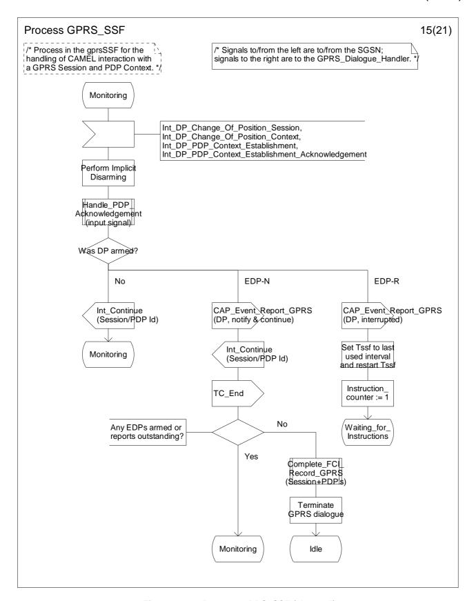
Figure 6.17o: Process GPRS\_SSF (sheet 15)
