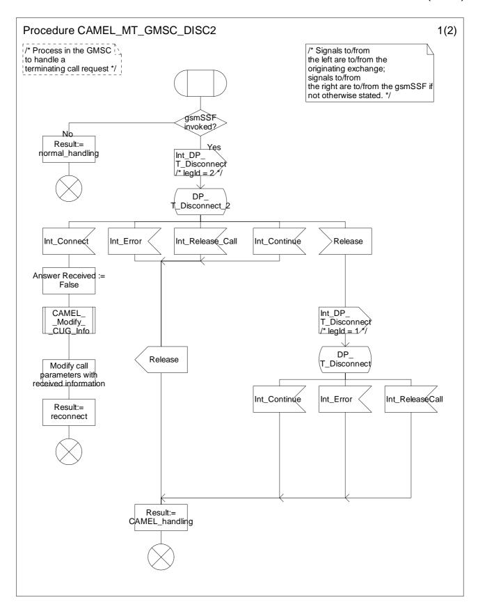
Figure 4.33a: Procedure CAMEL\_MT\_GMSC\_DISC2 (sheet 1)
