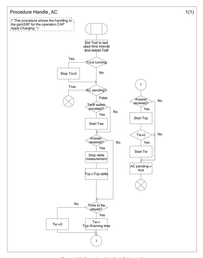
Figure 4.69: Procedure Handle\_AC (sheet 1)
