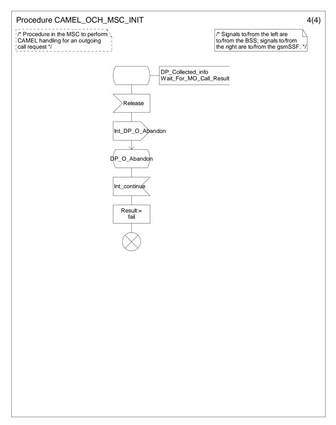
Figure 4.10d: Procedure CAMEL\_OCH\_MSC\_INIT (sheet 4)
