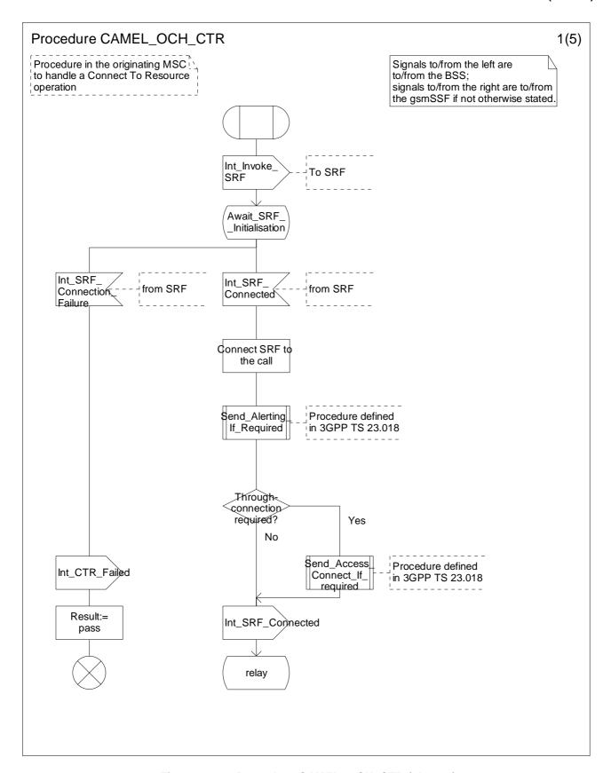
Figure 4.21a: Procedure CAMEL\_OCH\_CTR (sheet 1)
