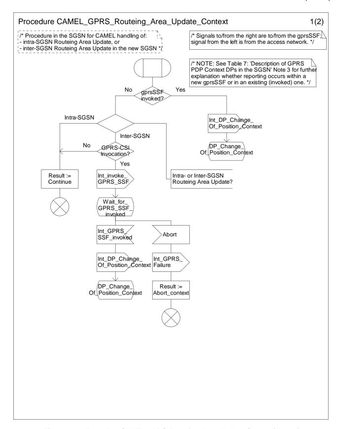
Figure 6.11a: Procedure CAMEL\_GPRS\_Routeing\_Area\_Update\_Context (sheet 1)
