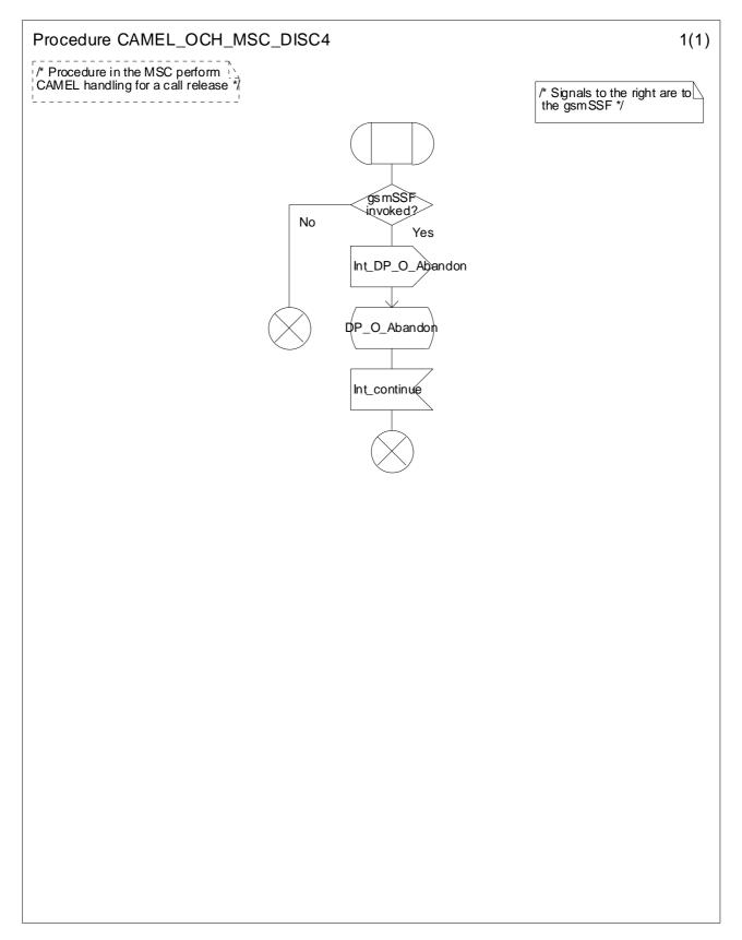
Figure 4.19: Procedure CAMEL\_OCH\_MSC\_DISC4 (sheet 1)
