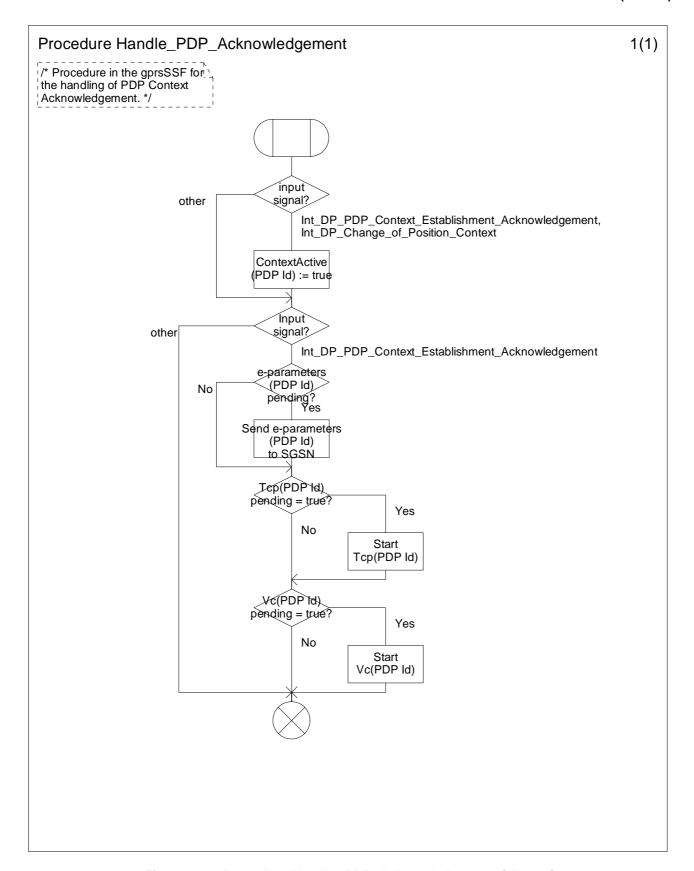
Figure 6.24: Procedure Handle\_PDP\_Acknowledgement (sheet 0)
