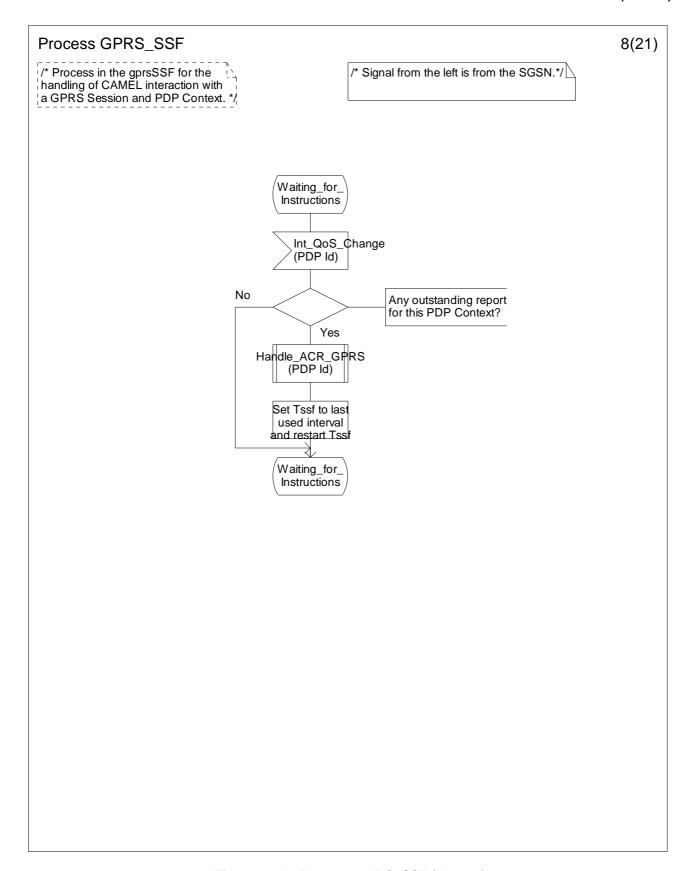
Figure 6.17h: Process GPRS\_SSF (sheet 8)
