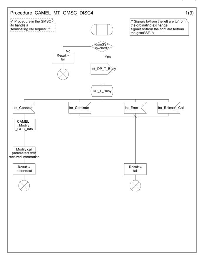
Figure 4.35a: Procedure CAMEL\_MT\_GMSC\_DISC4 (sheet 1)
