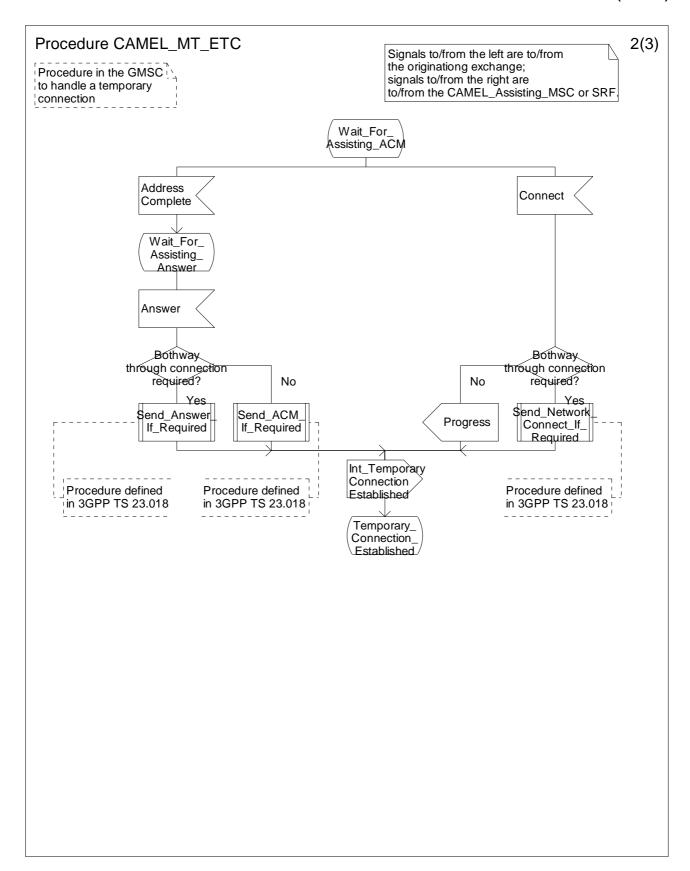
Figure 4.38b: Procedure CAMEL\_MT\_ETC (sheet 2)
