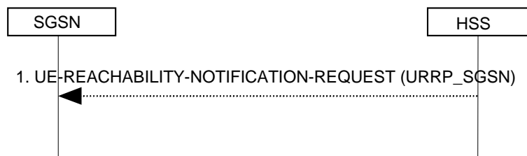
Figure 6.15-1: UE Reachability Notification Request Procedure
