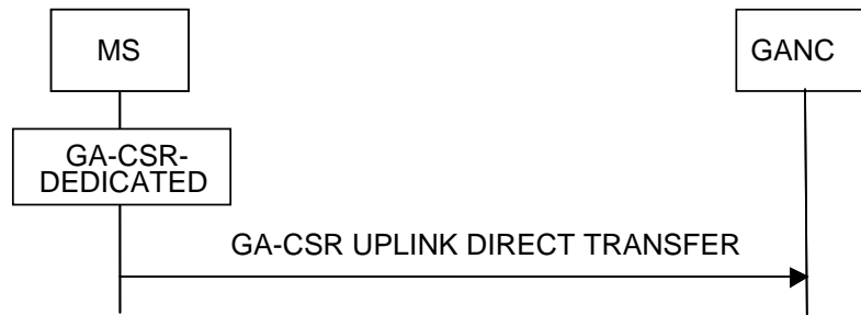
Figure 7.2.1.1 Uplink Direct Transfer, normal flow
