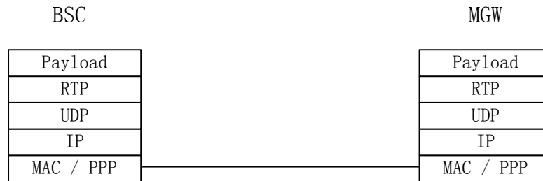
Figure 6.1.1.2.1: User Plane: AoIP protocol stack
