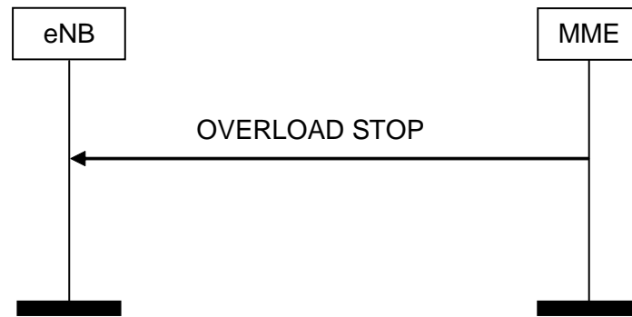
Figure 8.7.7.2-1: Overload Stop procedure
