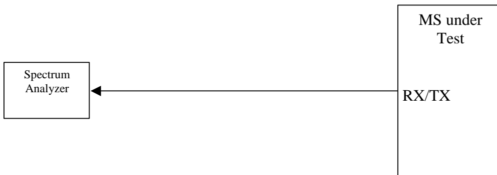
Figure A.8: Connection for Spurious Emission Test
