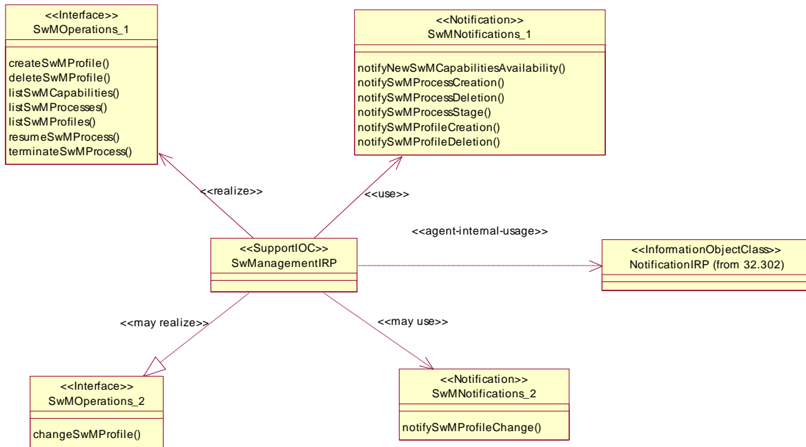
Figure 5.1-2 Operations and Notifications for ASWM
