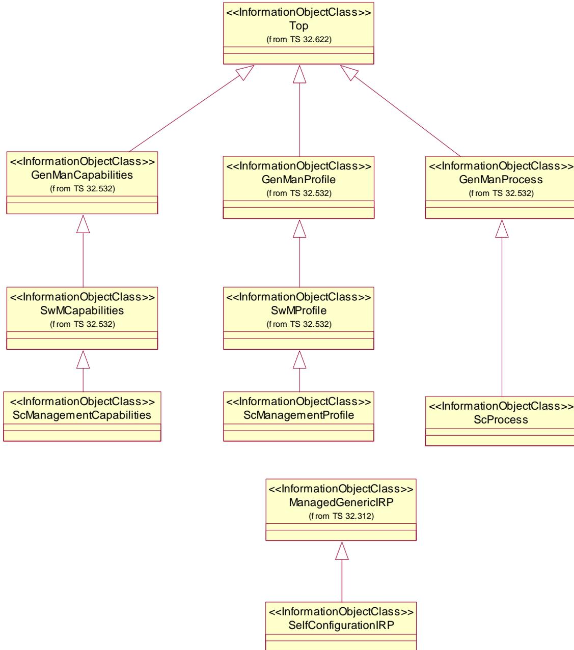
The following UML diagram describes the inheritance of the objects required for ARCF.
