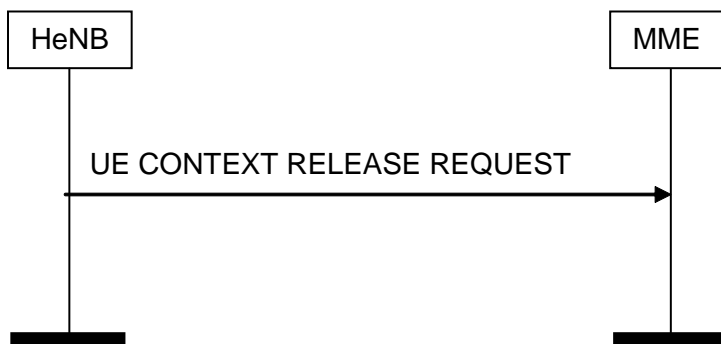
Figure 7 UE Context Release Request procedure. Successful operation
