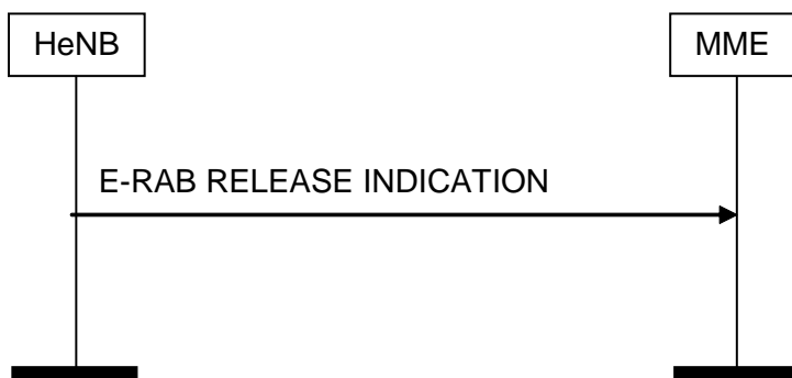
Figure 9 E-RAB Release INDICATION procedure. Successful operation
