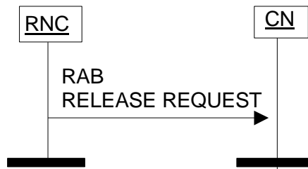
Figure: RAB Release Request procedure
