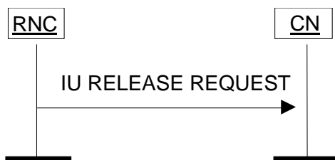
Figure: Iu Release Request procedure. Successful operation
