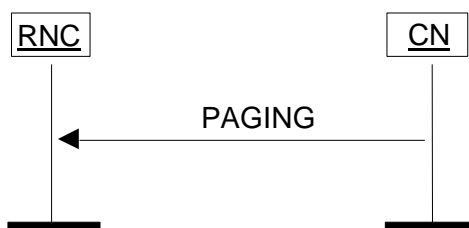
Figure: RANAP Paging procedure (Successful operation)
