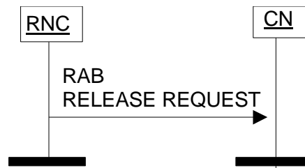
Figure: RAB Release Request procedure
