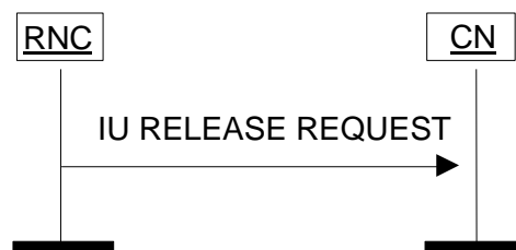
Figure: Iu Release Request procedure. Successful operation
