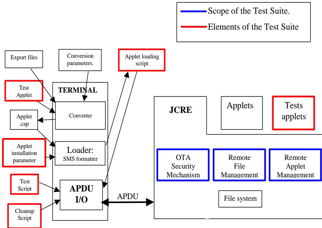
Note: This diagram shows the test architecture required to test interoperability at both API and bytecode level. The latter is currently not included in the current specification. The diagram is for information.
