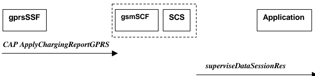
Figure 13-12: Call Flow for superviseDataSessionRes
