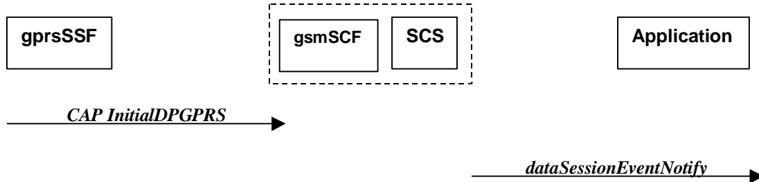
Figure 13-3: Call Flow for dataSessionEventNotify
