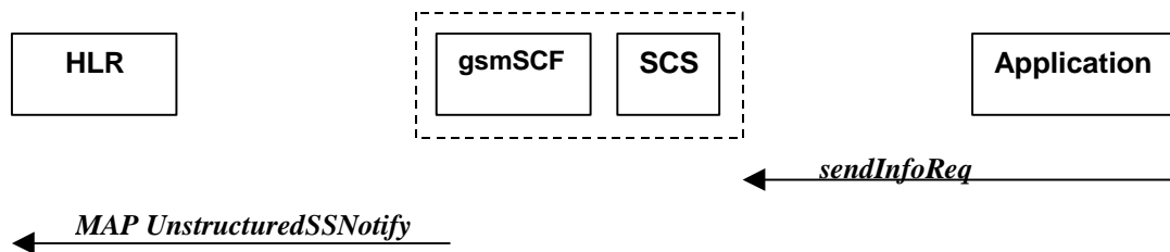
Figure 7-12: Call Flow for sendInfoReq (scenario 1)
