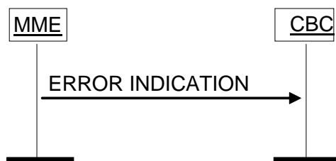
Figure 4.3.3B.2-2: Error Indication procedure, MME originated. Successful operation.
