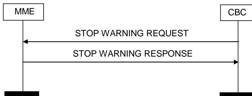
Figure 4.3.3A.2-1: Stop Warning Procedure, Successful Operation.
