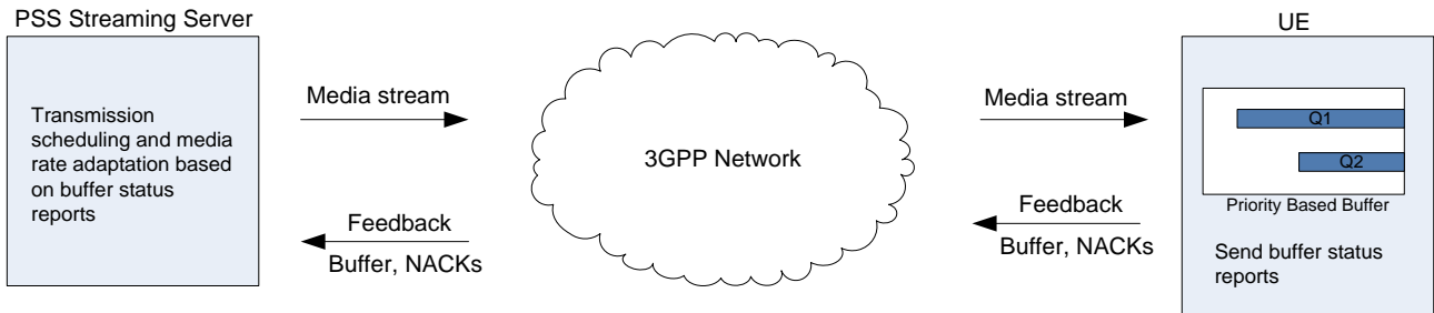
Figure 8: Transmission scheduling and media rate adaptation based on priority based buffer status reports
