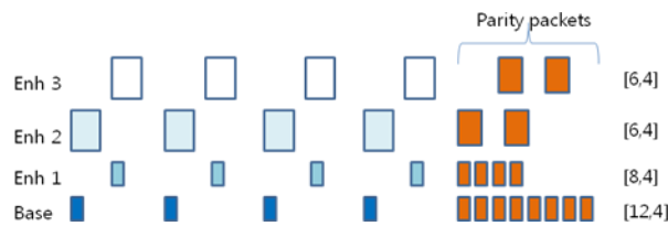
Figure 15: UEP (Unequal Error Protection): Important packets are protected with higher code rate
