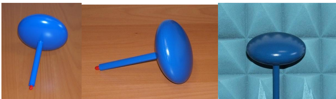
Figure 7.7 Examples of reference magnetic dipoles (loop antennas) [41].
