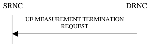
Figure 6: UE Measurement Termination procedure, Successful Operation
