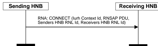
Figure 7.3.2.2.1-1: Signalling Connection Establishment – Direct Iurh-connectivity.
