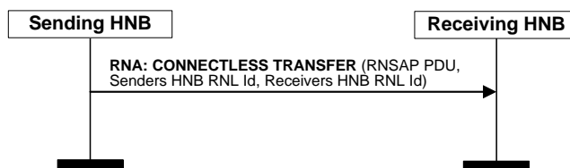
Figure 7.3.2.5.1-1: Connectionless data transfer – Direct Iurh-connectivity.
