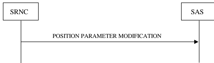
Figure 9e: Position Parameter Modification procedure, Successful Operation
