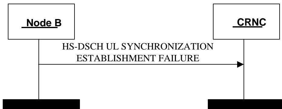
Figure 12D: HS-DSCH UL Synchronization Establishment Failure procedure
