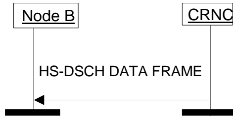
Figure 6A: HS-DSCH Data Transfer procedure
