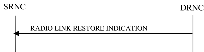
Figure 19: Radio Link Restoration procedure, Successful Operation
