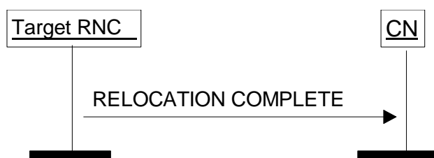
Figure 10: Relocation Complete procedure. Successful operation.
