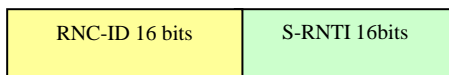
Figure A2.1.1.2: RNC-Side, split of U-RNTI in RNC-ID and S-RNTI in the case of many small RNCs deployed
