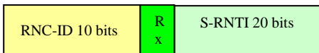
Figure A2.1.3.1: RNC Side, RNC-ID split into extended RNC-ID and sub-RNC indicator.
