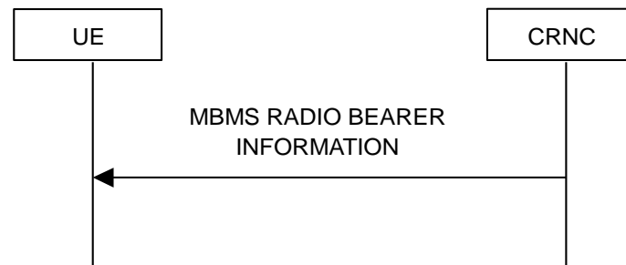
Figure 8.3.3: MBMS radio bearer information signalling flow
