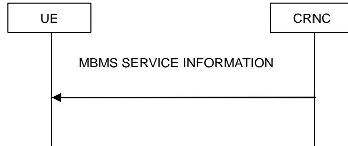
Figure 8.3.2: MBMS service information signalling flow
