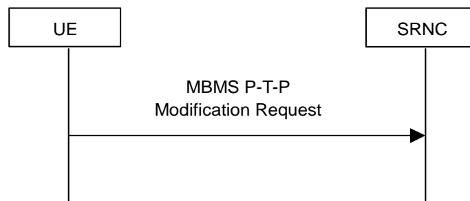
Figure 8.3.9: MBMS P-T-P Modification Request.
