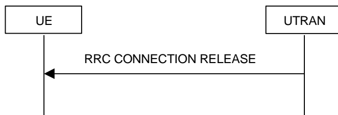
Figure 8.1.4-2: RRC Connection Release procedure on the CCCH
