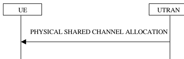
Figure 8.2.7-1: Physical Shared Channel Allocation
