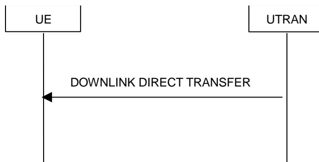
Figure 8.1.9-1: Downlink Direct transfer, normal flow
