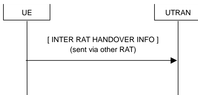
Figure 8.1.16-1: Inter RAT handover information transfer, normal flow
