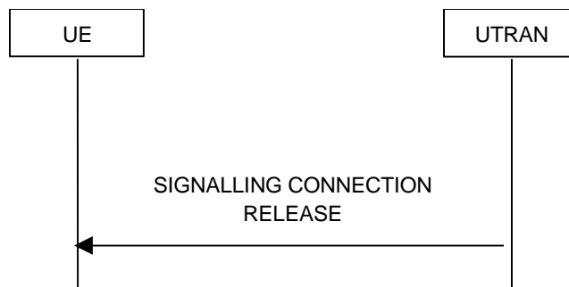
Figure 8.1.13-1: Signalling connection release procedure, normal case
