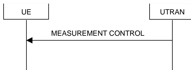
Figure 8.4.1-1: Measurement Control, normal case
