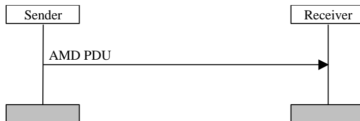
Figure 11.3: Acknowledged mode data transfer procedure
