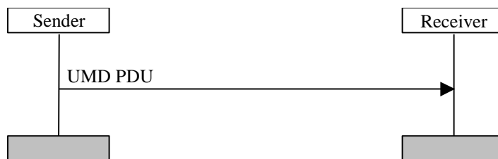
Figure 11.2: Unacknowledged mode data transfer procedure
