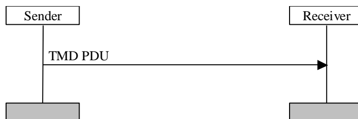
Figure 11.1: Transparent mode data transfer procedure
