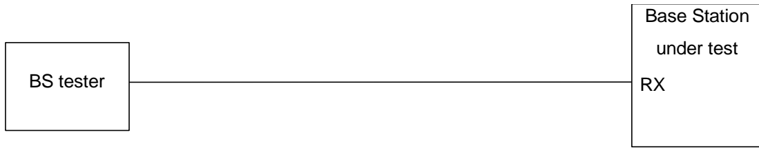
Figure B.15A: Functional Set-up for Verification of the internal BLER calculation for BS without Rx diversity
