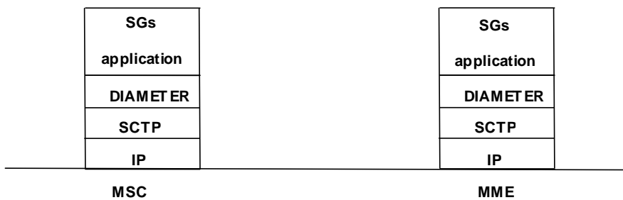
Fig. 10.14.1.1.2.1: Protocol architecture for alternative 2
