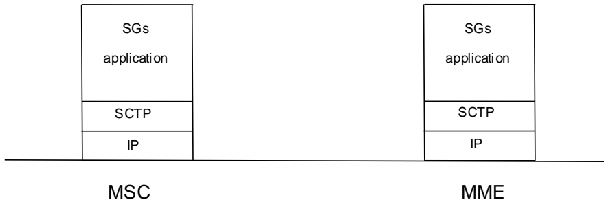
Fig. 10.14.1.1.2.2: Protocol architecture for alternative 2'
