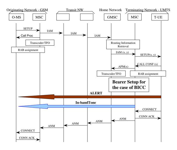
Figure 7.5.5: GSM MS  $\wedge$  UMTS UE call, APM-user not supported in the GSM network
