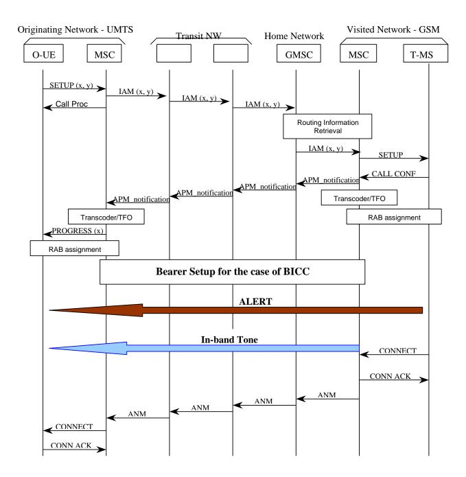
Figure 7.5.3: UMTS UE ∧ GSM MS call, APM-user not supported in the GSM
