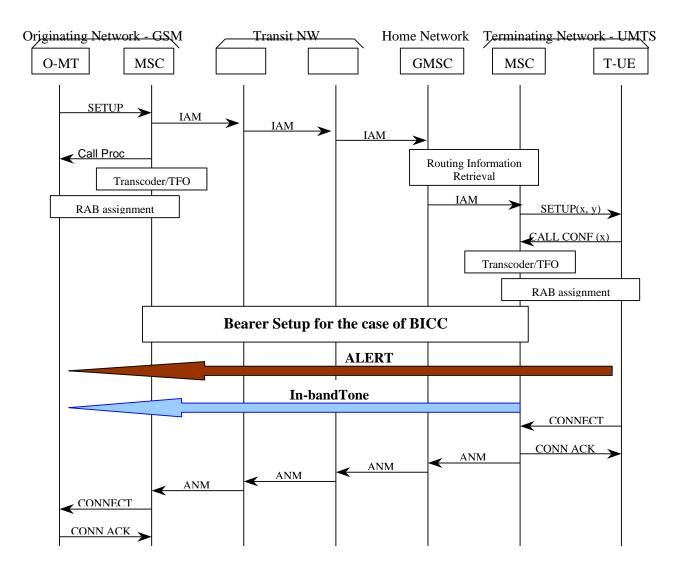
Figure 7.5.4: GSM MS  $_{\wedge}$  UMTS UE call, APM-user not supported in the GSM network
