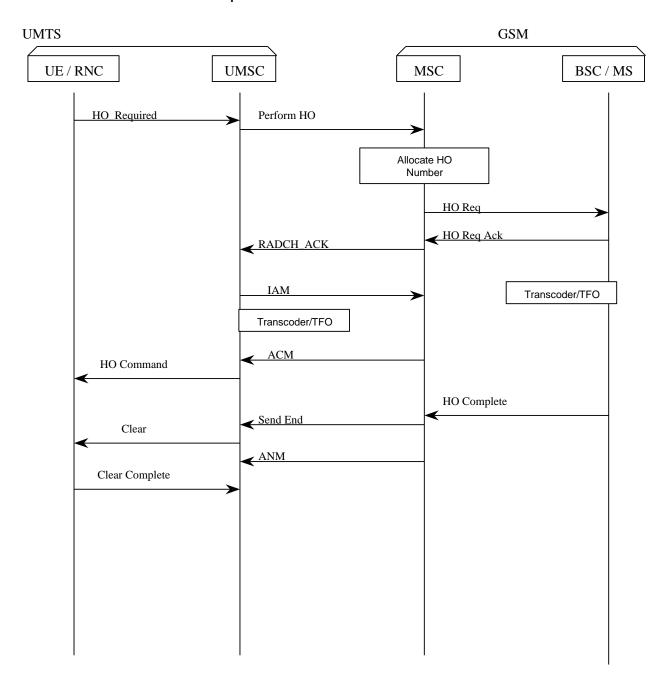
Figure 7.5.6: UMTS A GSM Handover after transcoder free establishment
