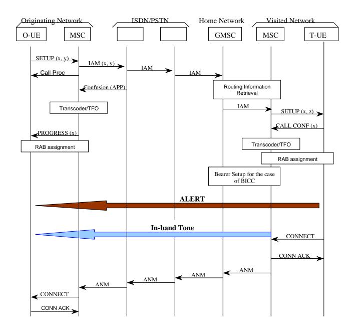
Figure 7.5.2: UMTS UE - UMTS UE call with transit network (PSTN/ISDN) not supporting
