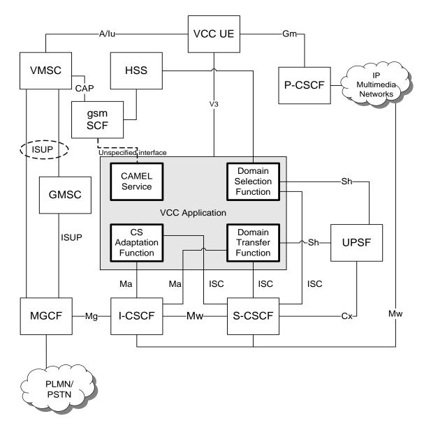
NOTE: Not all standard GSM interfaces are depicted in the architecture. Connection between the elements (VMSC, GMSC, MGCF) may be via a transit network. CS domain termination may bypass the GMSC.
