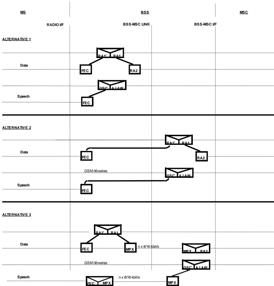
Figure 8: Location of transcoding and rate adaptation
