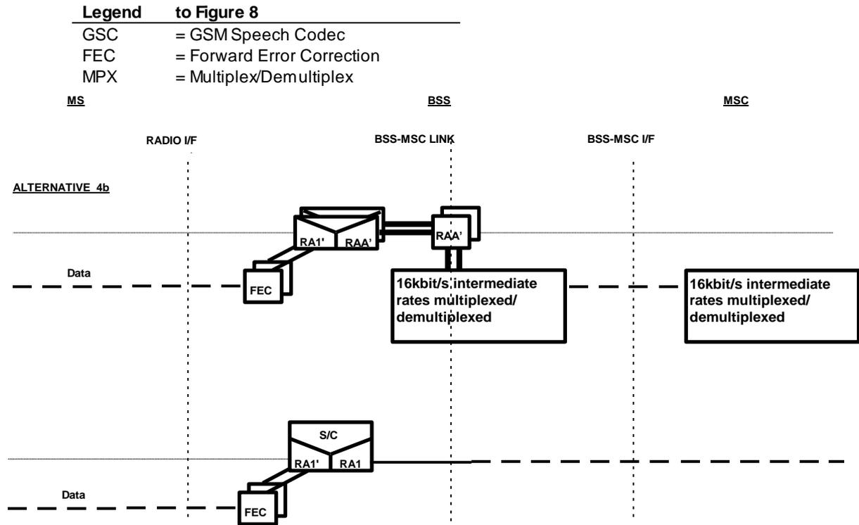
Figure 8 (concluded): Location of transcoding and rate adaptation
