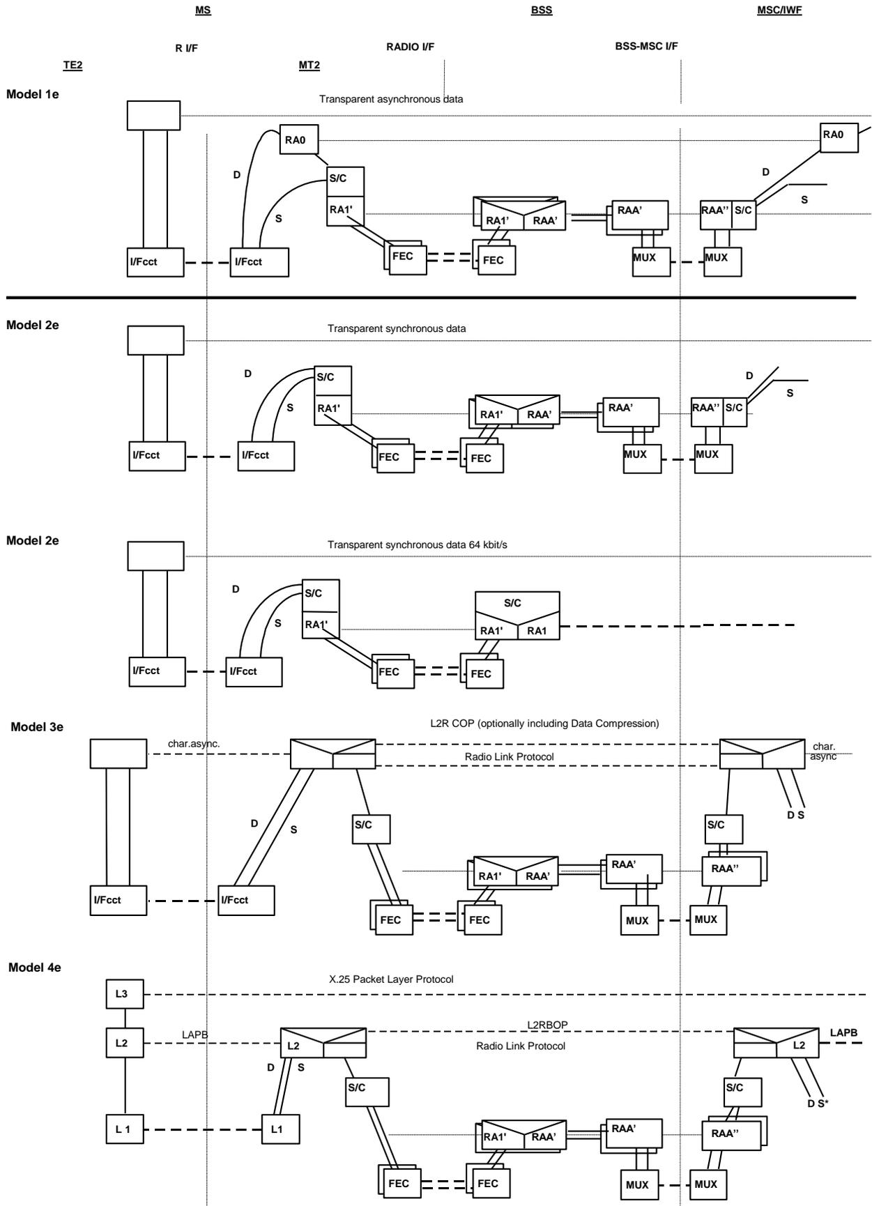
Figure 7 (continued) : Information transfer protocol models for GSM PLMN connections using 14.4 channels
