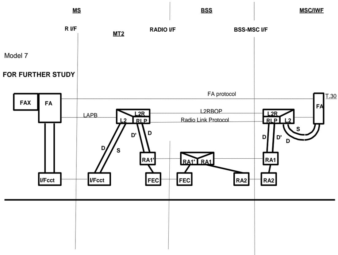
Figure 6 (continued): Information transfer protocol models for GSM PLMN connections
