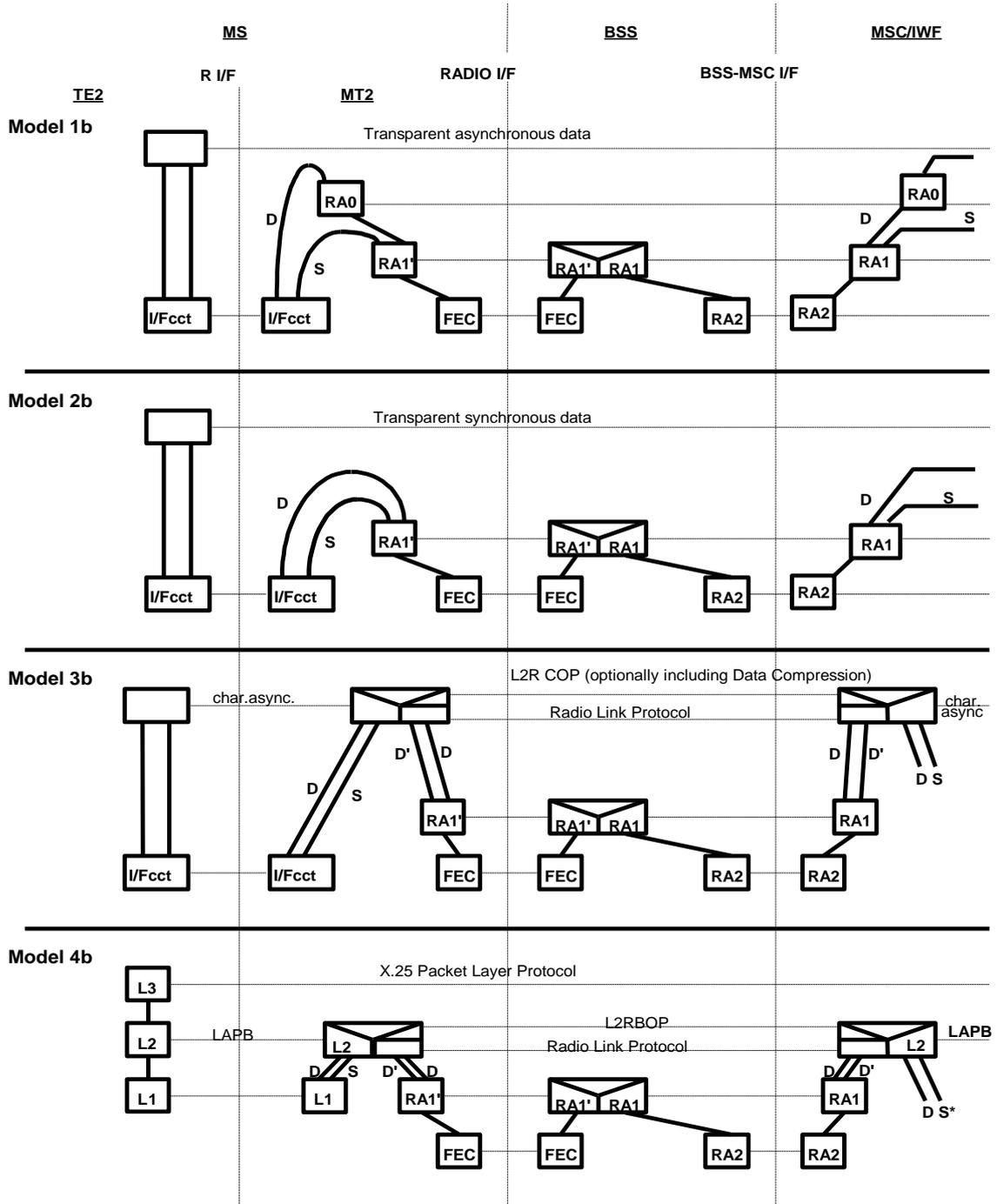
Figure 6 (continued): Information transfer protocol models for GSM PLMN connections
