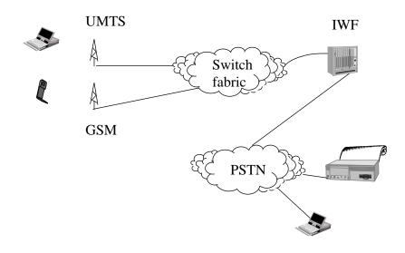
The IWF provides a range of modems which can be accessed via a circuit switched or packet switched connection. These modems could talk over the PSTN to other modems or to fax machines, entirely at the discretion of the caller. The caller would first establish a connection to the modem and the instruct the modem as to how to set the call up from there. When the call is disconnected then a message is sent back to the user advising of the call cost.
