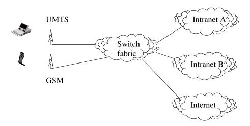
This scenario shows how connections can be established to the Internet or Intranets, following the GPRS model.
