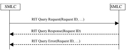
This operation allows a SMLC to query RIT information from another SMLC. This operation consists of sending of a RIT Query Request. It includes the Request ID, that is used to identify different queries. The RIT Query Request also includes the description of the scheduling of RIT Indication operations in the reverse direction. This includes the following cases:
