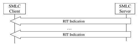
In the autonomous mode the procedure consists of one or more RIT Indication operations.
