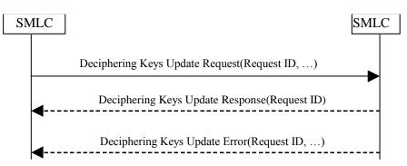
This operation allows a SMLC controlling deciphering keys to send the keys to another SMLC Client.
