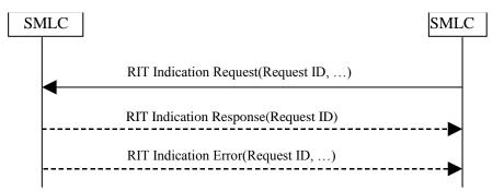
This operation allows a SMLC to send RIT information to another SMLC. It can be used both in the cased of autonomous provision, and the provision of RIT information on request.
