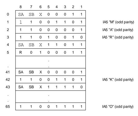
Figure 2c A 66-octet RLP L2RCOP PDU with status octets separated by more than 23 octets
